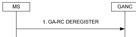
Figure 56: De-Registration initiated by the MS
