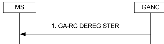
Figure 57: De-Registration initiated by the GANC
