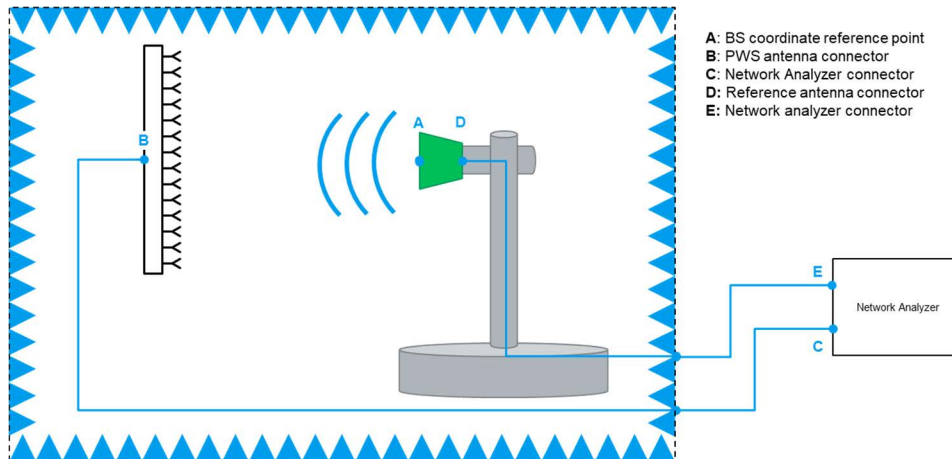
Figure 8.6-1: Path loss calibration in PWS, TX requirements
