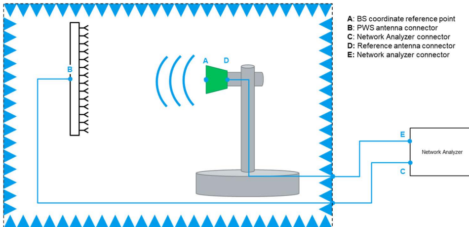
Figure 8.6-1: Path loss calibration in PWS, TX requirements
