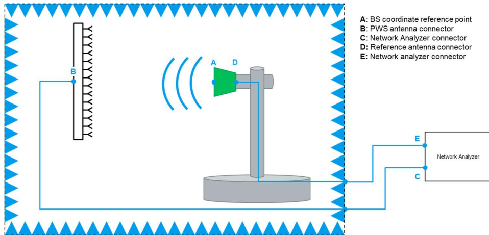
Figure 8.6-1: Path loss calibration in PWS, TX requirements
