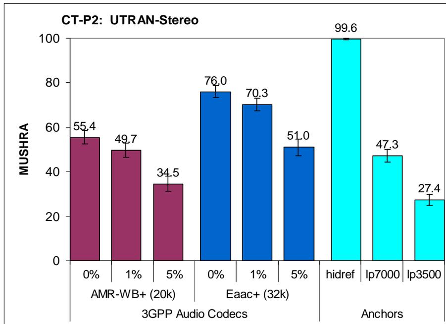
Figure 25: Results for UTRAN, lower-rate at three levels of PLR (stereo mode)
