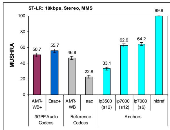
Figure 19: Results at 18 kbps for MMS (stereo)
