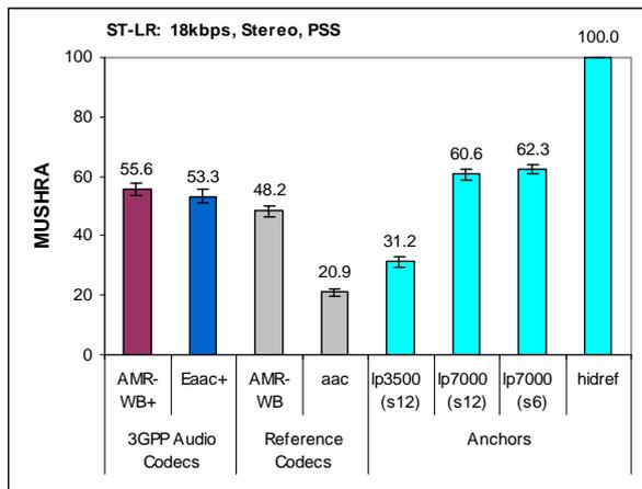
Figure 14: Results at 18 kbps for PSS (stereo)
