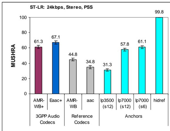
Figure 15: Results at 24 kbps for PSS (stereo)
