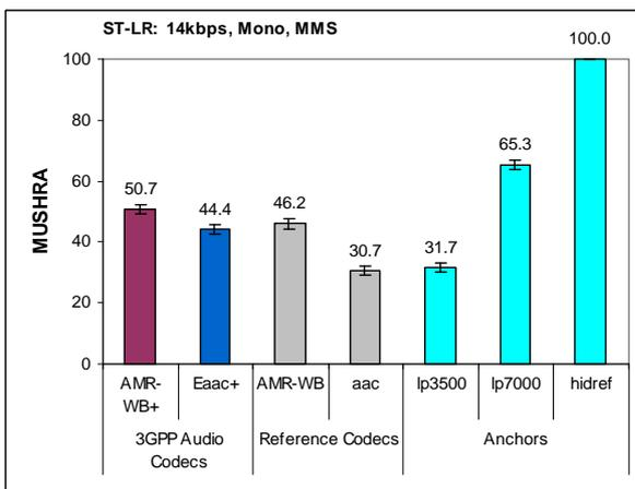
Figure 18: Results at 14 kbps for MMS (mono)
