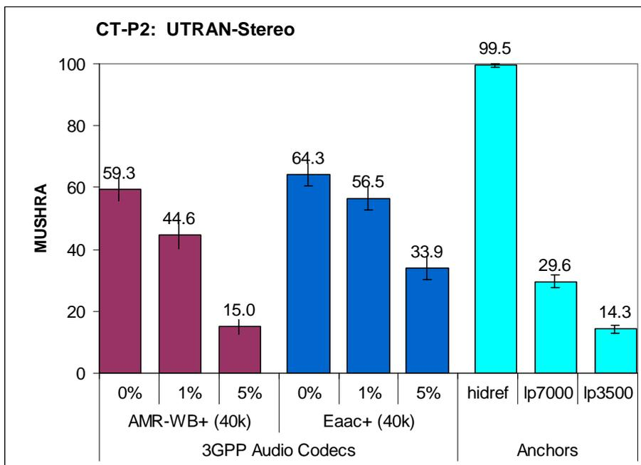
Figure 26: Results for UTRAN, Higher-rate at Three Levels of PLR (stereo mode)
