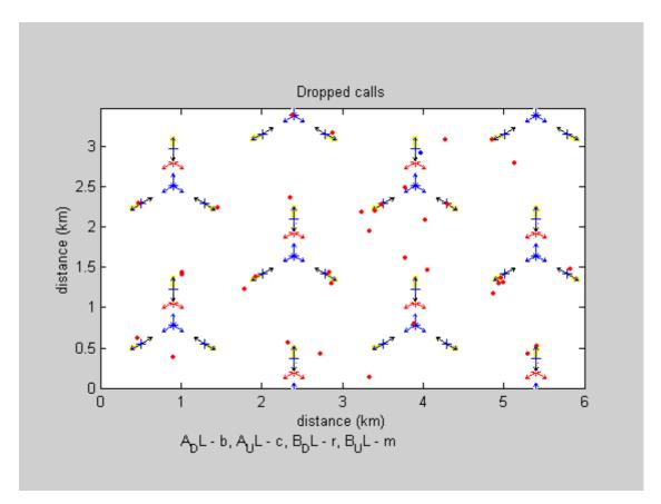
Figure 6.46: Dropped calls for operator A and operator B in case 2 – ACRR = 4 dB.
