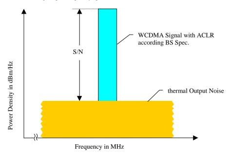
Fig. 4.2: Repeater output frequency spectrum.
