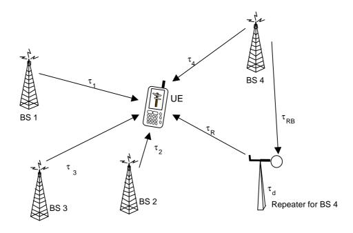
Fig. 4.4: Illustration of the effect of a repeater installation in a network using OTDOA based LCS.
