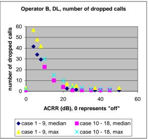
Figure 6.43: Number of dropped calls due to DL causes for operator A and operator B.
