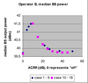
Figure 6.37: Median BS output power for operator A and operator B.
