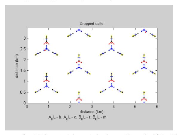
Figure 6.63: Dropped calls for operator A and operator B in case 18 – ACRR = 45 dB.
