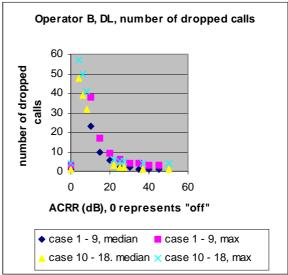
Figure 6.16: Number of dropped calls due to DL causes, operator A and operator B.
