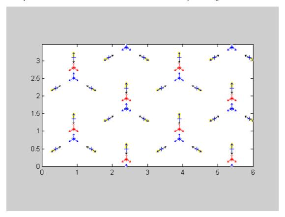
Figure 6.9: Infrastructure scenario. Operator A (blue) uses repeaters (+ positions). Operator B (red) does not use repeaters. Black arrows show repeater antenna directions. Yellow shade indicate service antenna.
