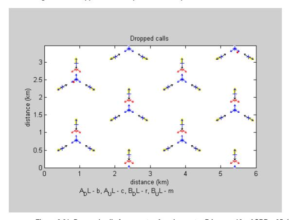
Figure 6.61: Dropped calls for operator A and operator B in case 16 – ACRR = 35 dB.
