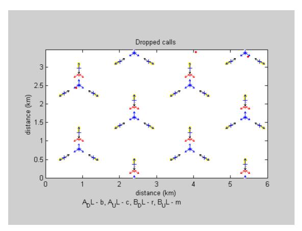
Figure 6.58: Dropped calls for operator A and operator B in case 13 – ACRR = 20 dB.
