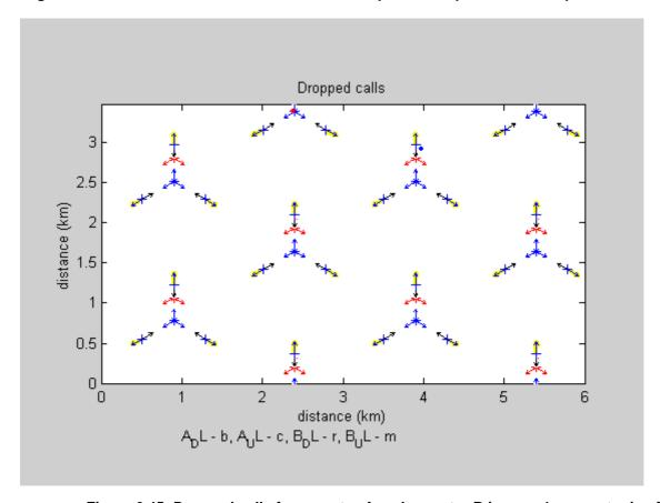
Figure 6.45: Dropped calls for operator A and operator B in case 1 – repeater is off.
