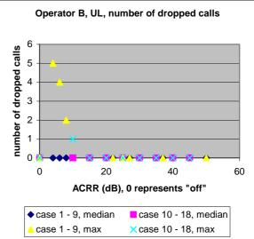
Figure 6.42: Number of saturated repeaters for operator A and number of dropped calls due to UL causes for operator B. Note that no calls were dropped due to UL causes for operator A.
