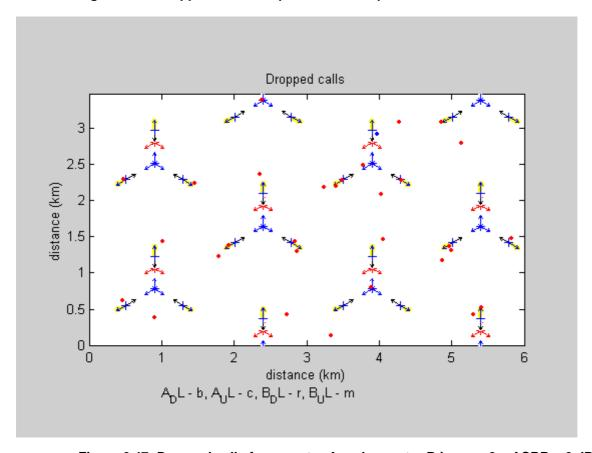
Figure 6.47: Dropped calls for operator A and operator B in case 3 – ACRR = 6 dB.
