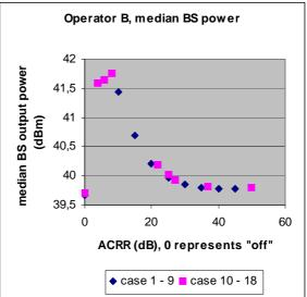
Figure 6.10: Median BS output power, operator A and operator B.
