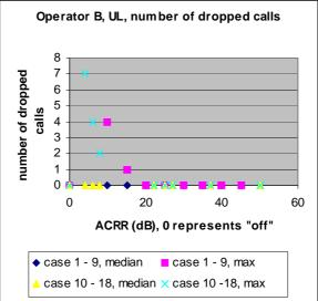
Figure 6.15: Operator A number of saturated repeaters and operator B number of dropped calls due to UL causes. Note that no calls were dropped due to UL causes for operator A.
