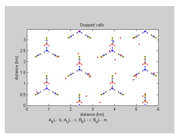
Figure 6.48: Dropped calls for operator A and operator B in case 4 – ACRR = 8 dB.
