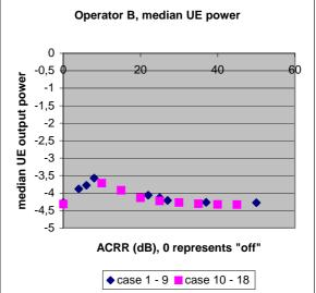
Figure 6.40: Median UE output power for operator A and operator B.
