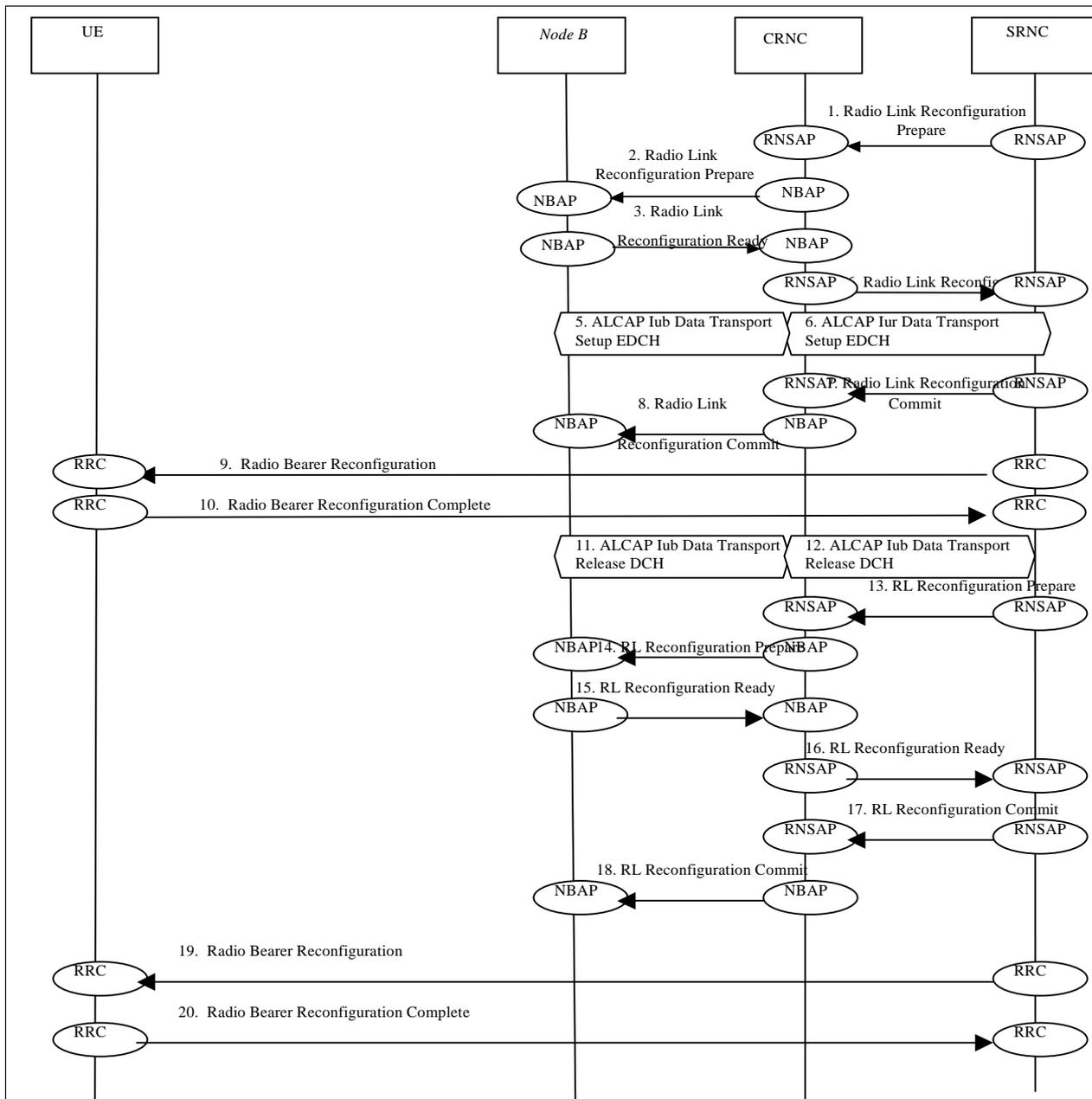
Figure 52: E-DCH Establishment and E-DCH TTI Reconfiguration
