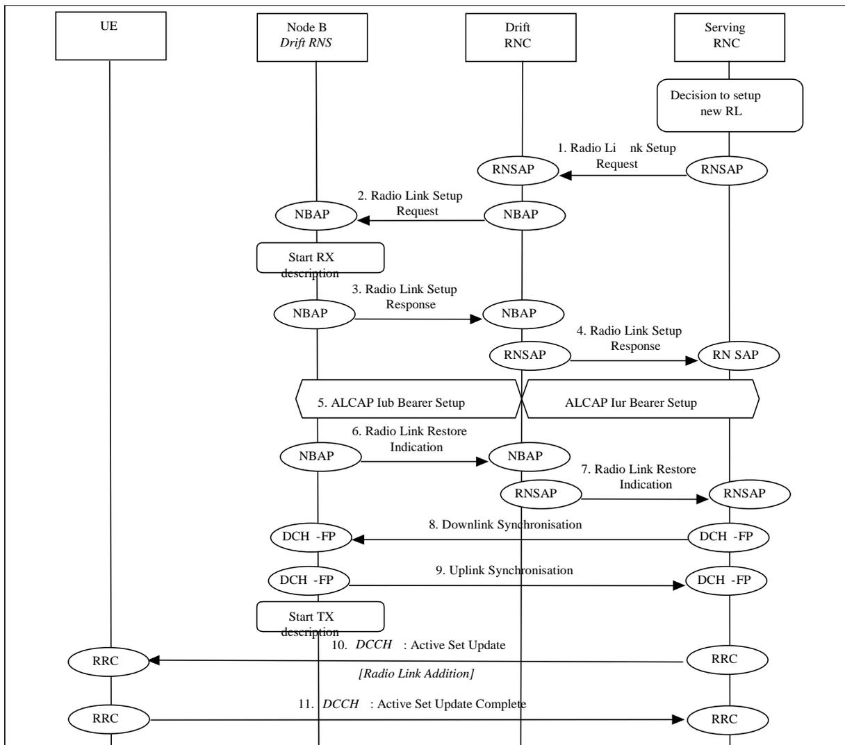
**Figure 24: Soft Handover - Radio Link Addition (Branch Addition)**
