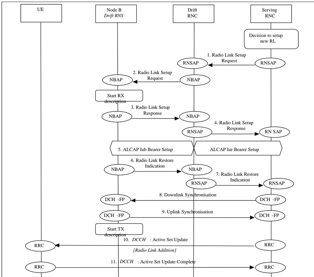
**Figure 53: Soft Handover - Radio Link Addition (Branch Addition)**
