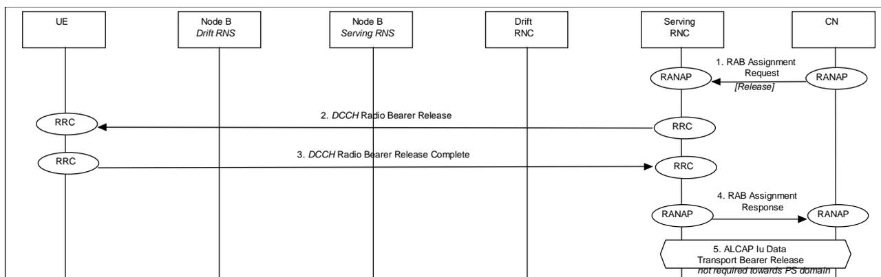
**Figure 19: Radio Access Bearer Release - RACH/FACH - RACH/FACH Release**
