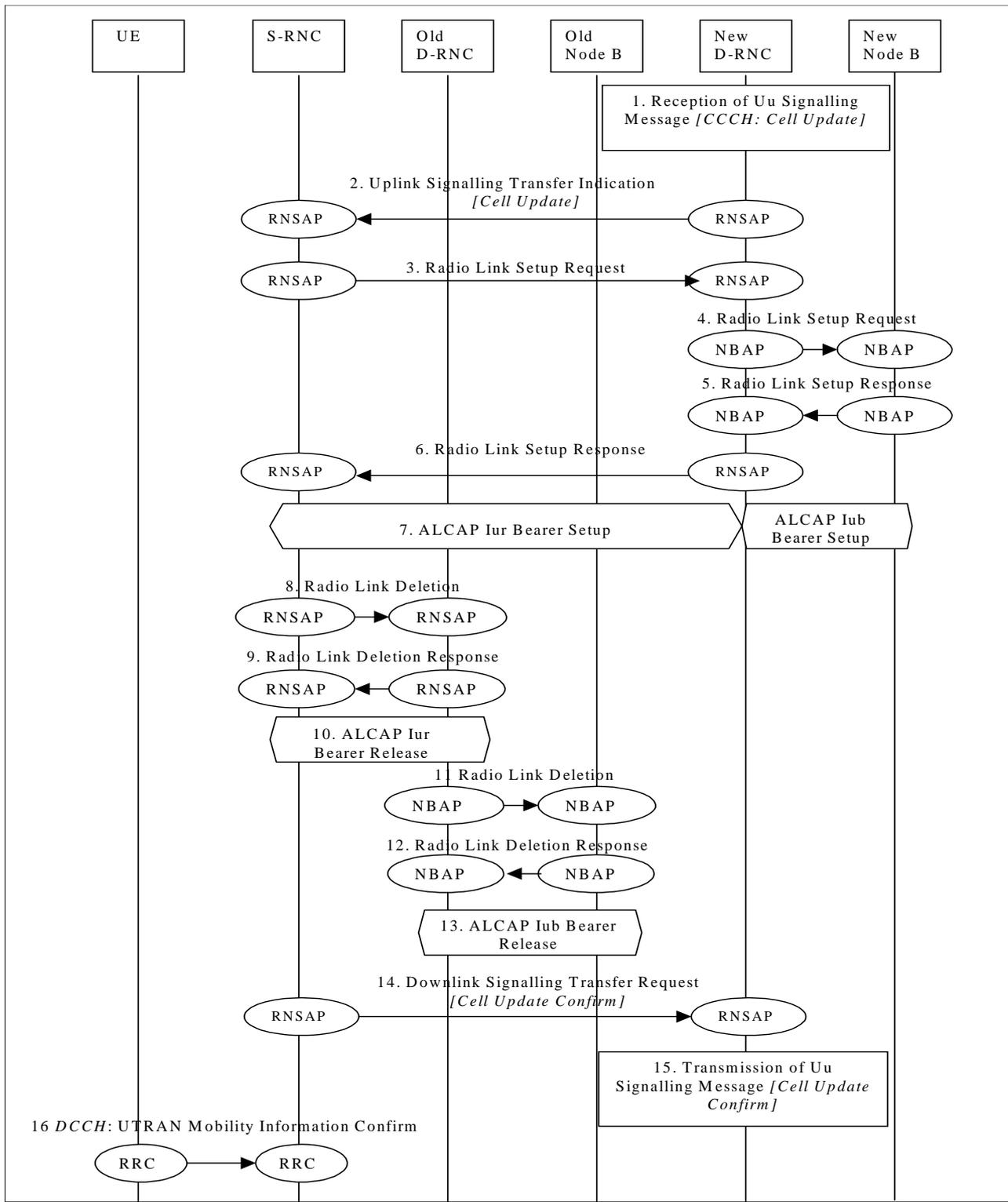
**Figure 11: RRC connection Re-establishment (Anchor approach) – DCH Re-establishment**
