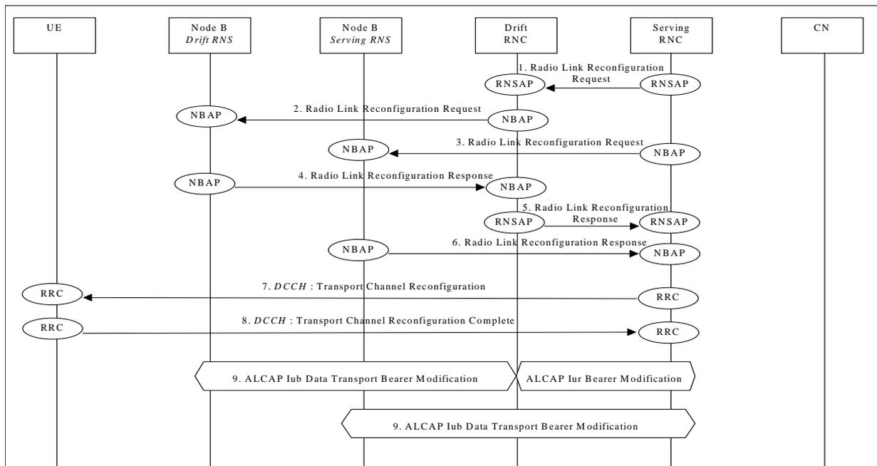
Figure 42b: Unsynchronised Transport Channel Reconfiguration, Bandwidth Decrease
