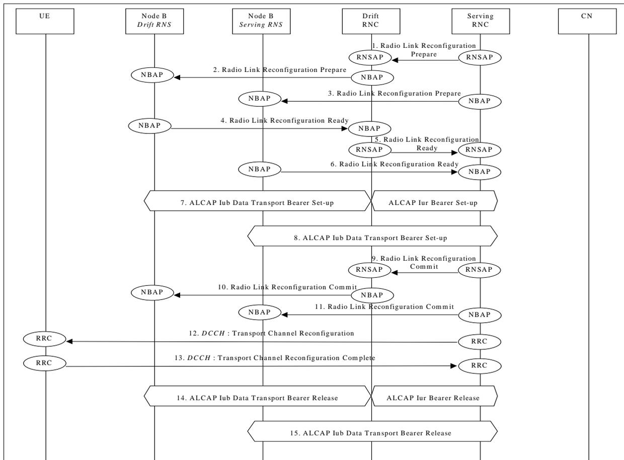
Figure 41: Synchronised Transport Channel Reconfiguration
