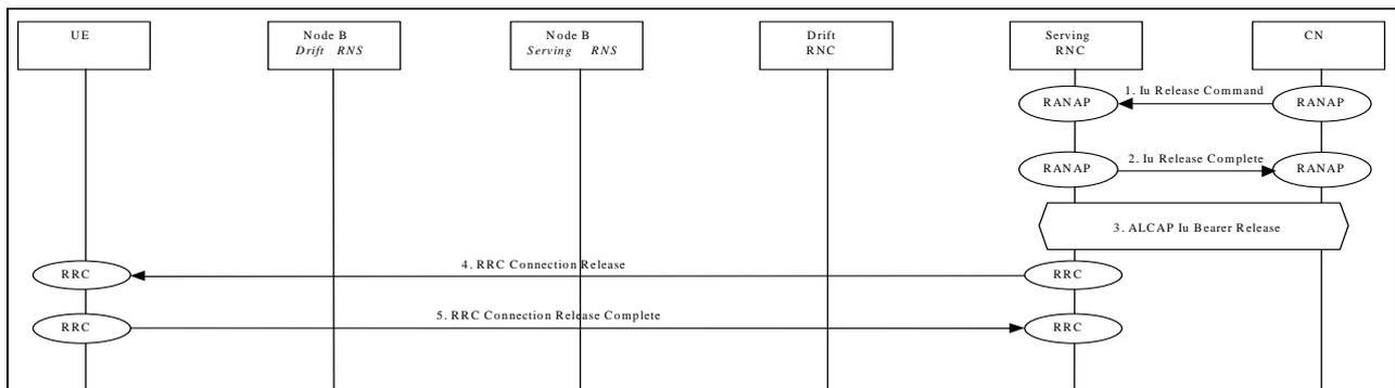
**Figure 10: RRC Connection release of a common transport channel**
