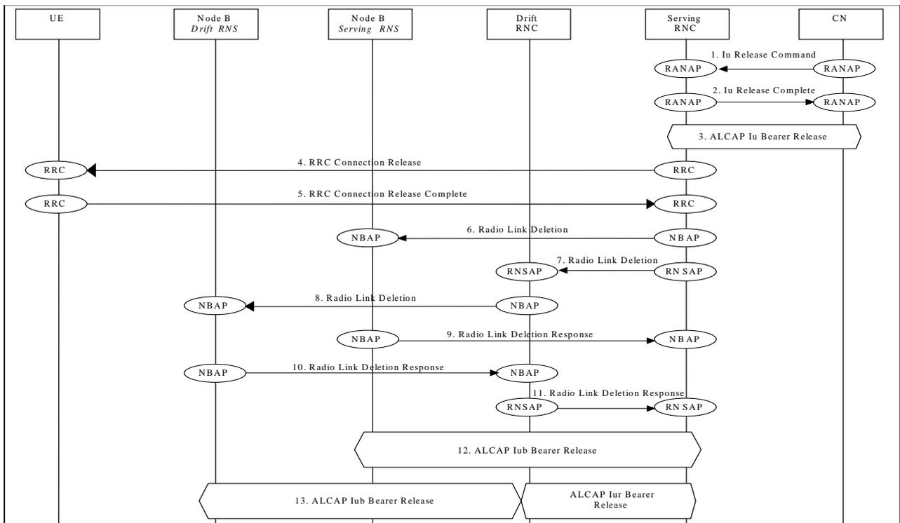
**Figure 9: RRC Connection release of a dedicated channel**
