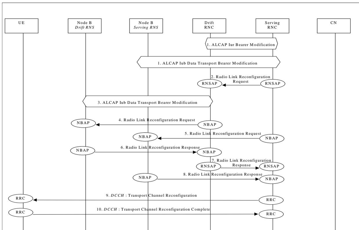
Figure 42a: Unsynchronised Transport Channel Reconfiguration, Bandwidth Increase
