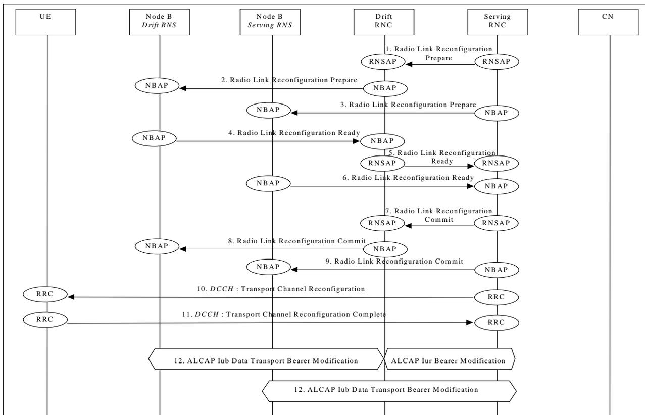
Figure 41b: Synchronised Transport Channel Reconfiguration, Bandwidth Decrease
