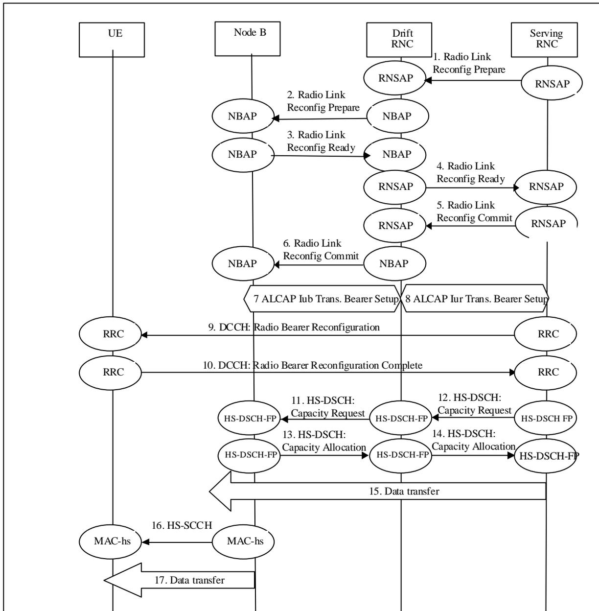
**Figure 45b: HS-DSCH Configuration and Capacity Allocation**
