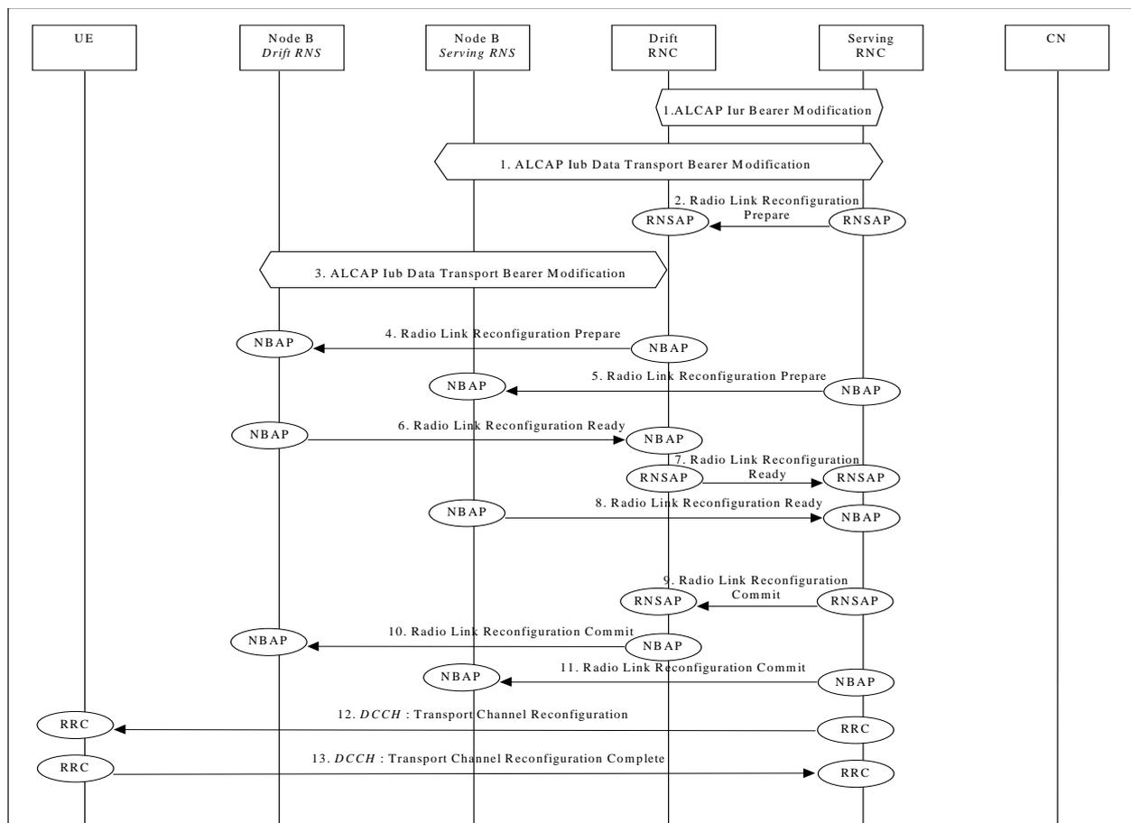
Figure 41a: Synchronised Transport Channel Reconfiguration, Bandwidth Increase
