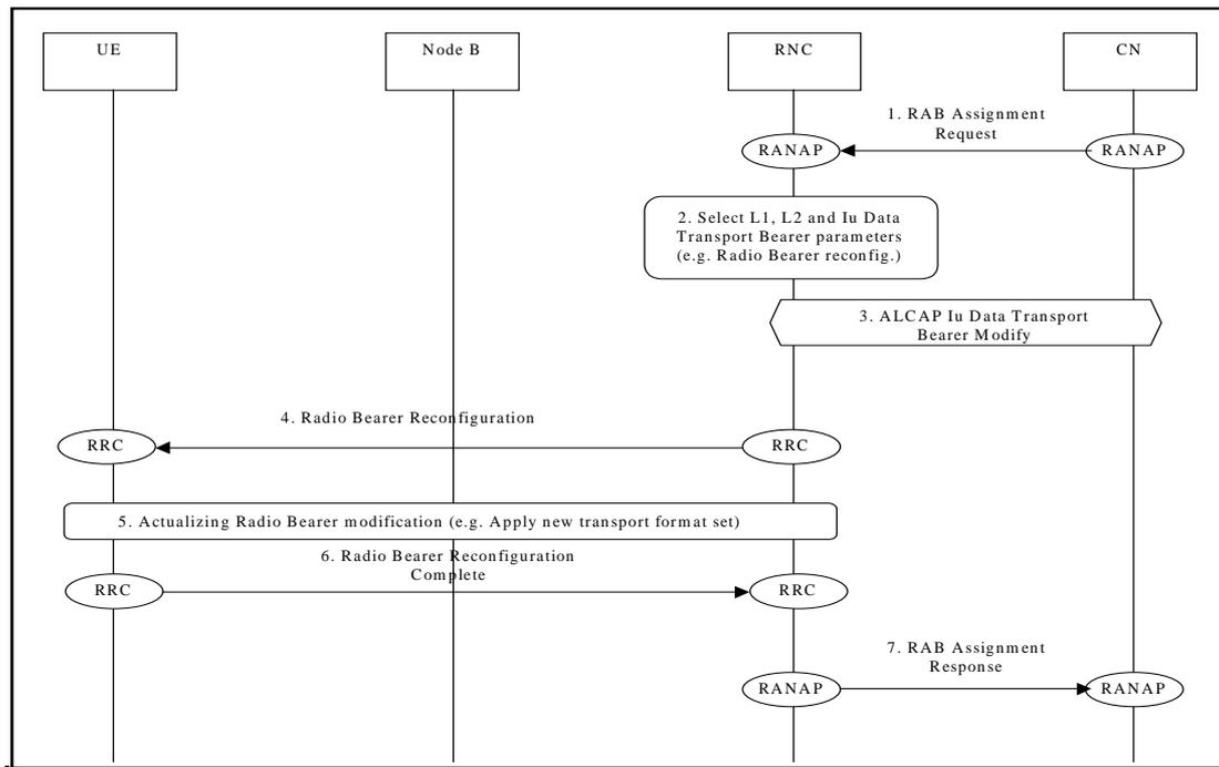
**Figure 21: Radio Access Bearer Modification – RACH/FACH Modification**
