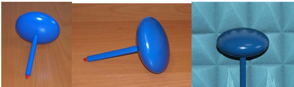
Figure 7.7 Examples of reference magnetic dipoles (loop antennas) [41].
