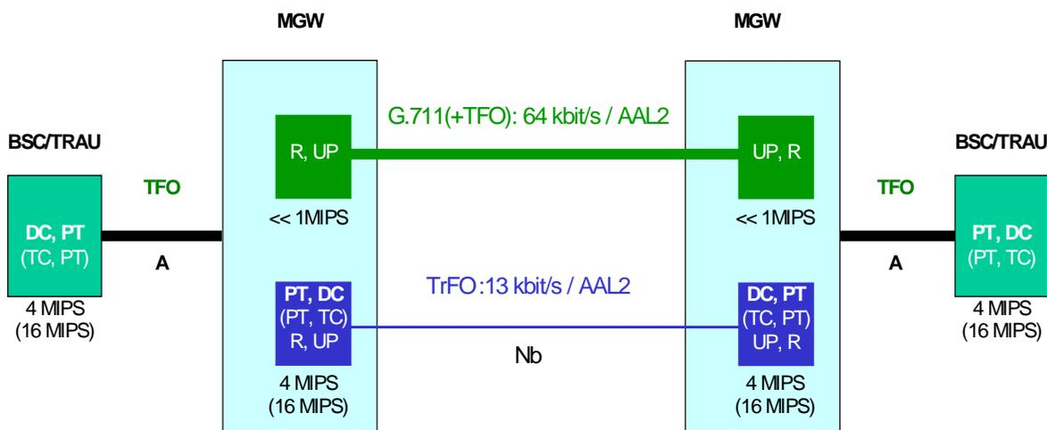
Note: The MIPS values in brackets() indicate the DSP-resource usage in the short TFO-setup phase, when TC is used.
