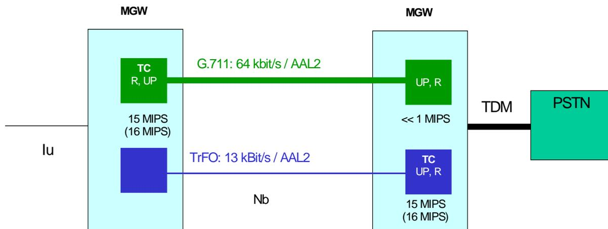
NOTE: The MIPS values in brackets() indicate the DSP-resource usage in the short TFO-setup phase, when TC is used.
