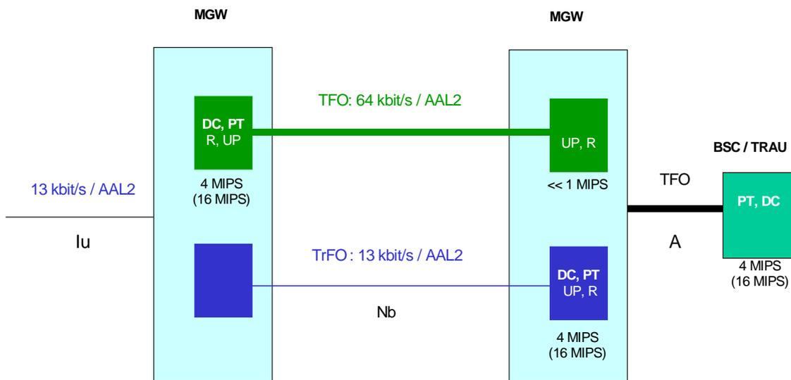
Figure 5.1.3-2: Bandwidth and resource usage for RNC to BSC call via BICN
