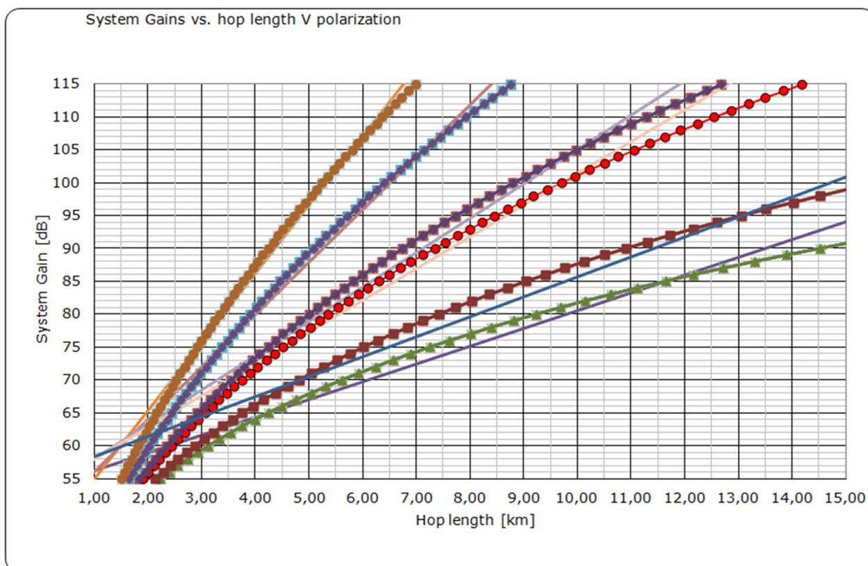
**Figure A.1: System Gain versus hop length [V polarization]**
