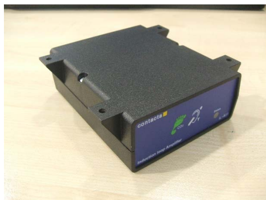
Figure 4: Small area hearing loop driver, typically installed under a counter
