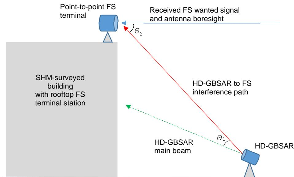
**Figure D.2: Representative worst-case scenario of HD-GBSAR to FS interference (V-plane only)**
