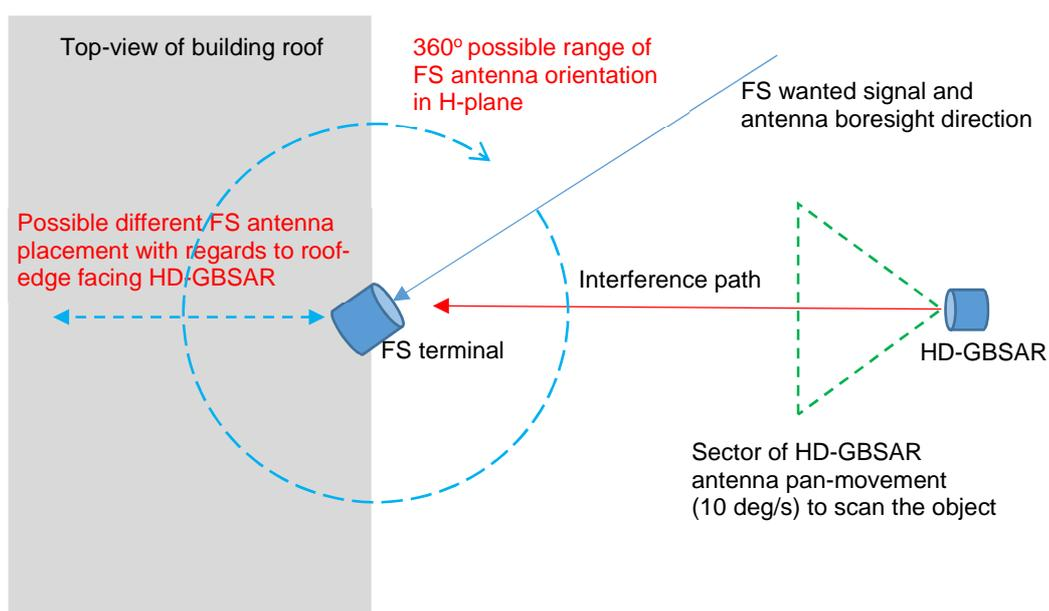
**Figure D.3: HD-GBSAR to FS interference scenario in H-plane**
