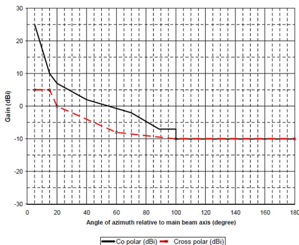
Figure D.1: Representative Radiation Pattern Envelope of FS antenna in 71-76 GHz
