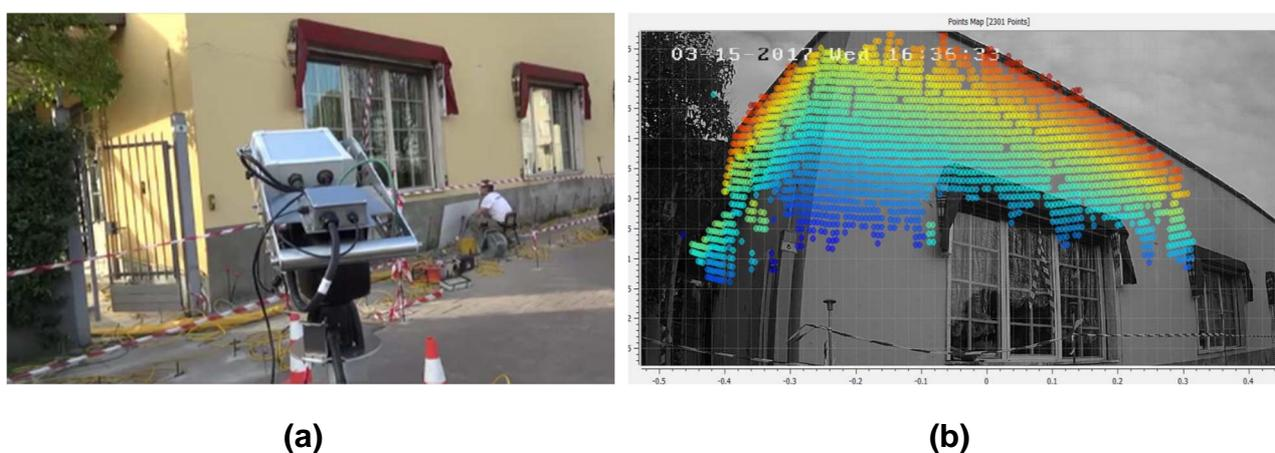
NOTE: (a) Deployment, (b) Measured displacement heat map.
