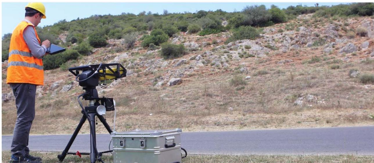
**Figure A.7: HD-GBSAR used for natural landslide monitoring**
