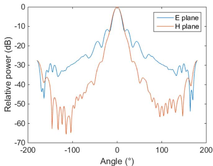
**Figure 4: HD-GBSAR antenna Type 2 radiation pattern**
