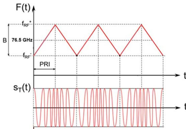
Figure B.1: HD-GBSAR signal in the frequency and time domain
