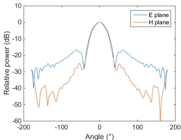
**Figure 3: HD-GBSAR antenna Type 1 radiation pattern**
