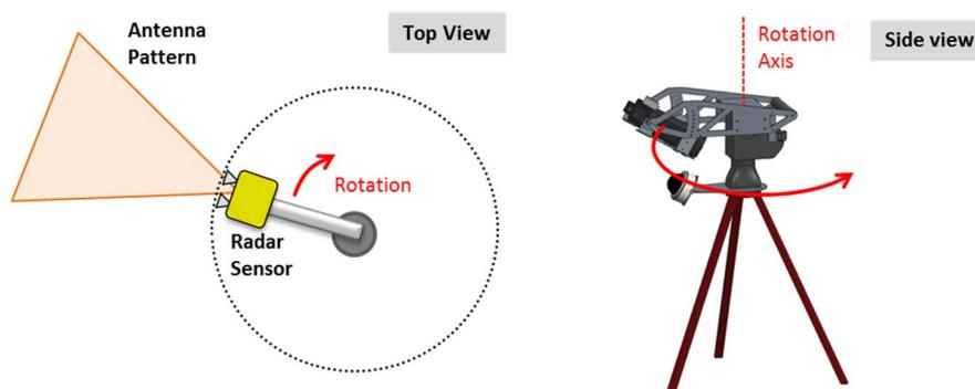
Figure B.2: Arc SAR acquisition
