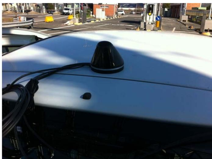
Figure 7: ITS-SU roof-top antenna installed in vehicle
