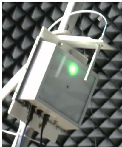
**Figure 10: Test antenna close to HDR-DSRC RSU, measuring the OBU and ITS-SU spectrum**
