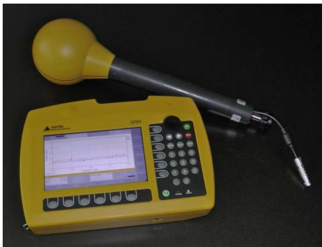
Figure 16: SRM 3006 with antenna
