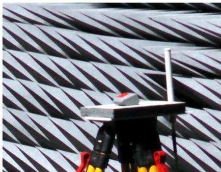
**Figure 11: Test antenna close to HDR-DSRC OBU, measuring the RSU spectrum**
