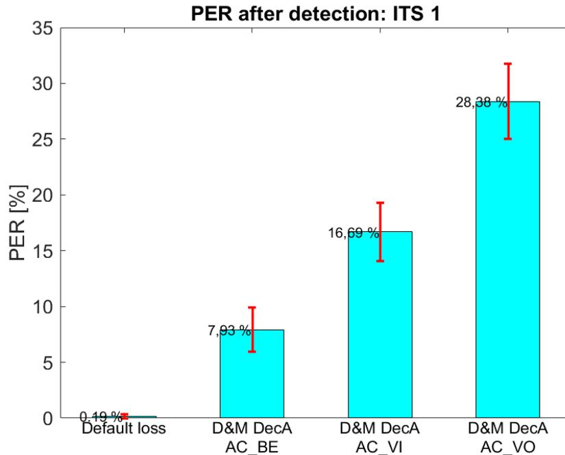
NOTE: Decreased EDCA Plan A method is used. Wi-Fi packet duration is 2,5 ms.
