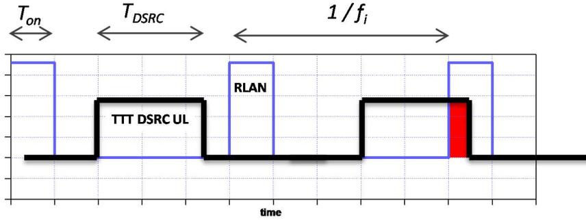
**Figure A.2: Interference can happen when victim and interferer transmit at the same time**
