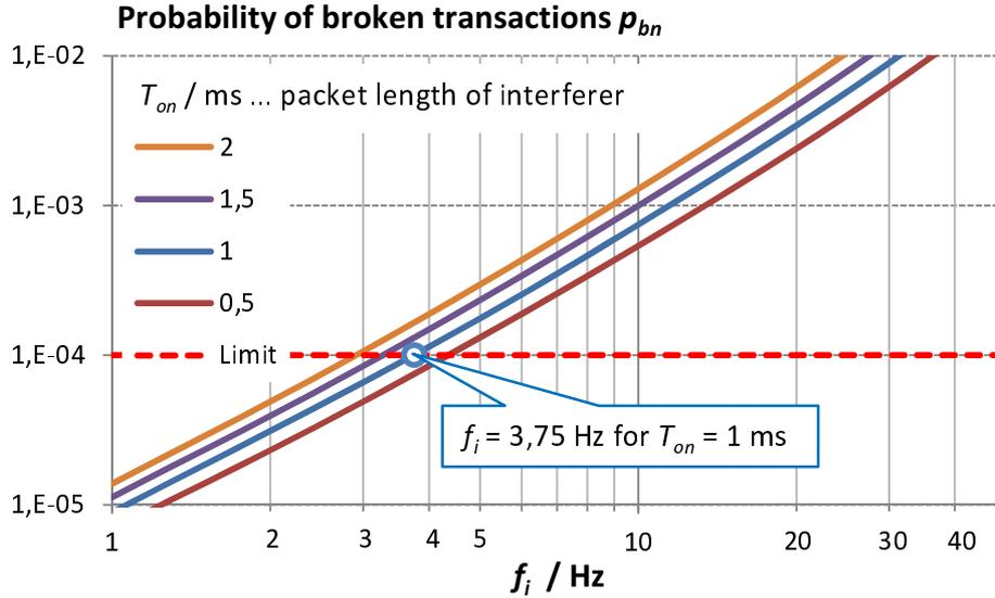
**Figure A.3: Probability of broken toll transactions in a 4 lane MLFF tolling scenario for a vehicle speed of 100 km/h and different RLAN message duration as function of the total average RLAN message rate  $f_i$**
