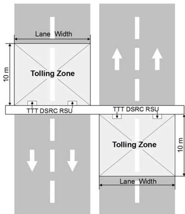
**Figure A.1: Example of tolling zone geometry**
