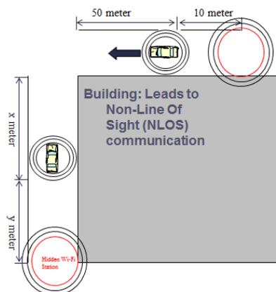
Figure B.2: Intersection collision avoidance (scenario 2)
