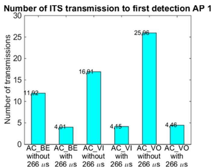
**Figure B.25: The average number of ITS transmissions needed before first successful detection at AP**
