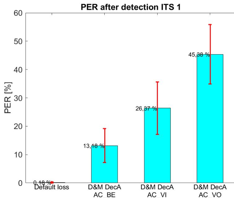
NOTE: Decreased EDCA Plan A method is used. Wi-Fi packet duration is 2,5 ms.
