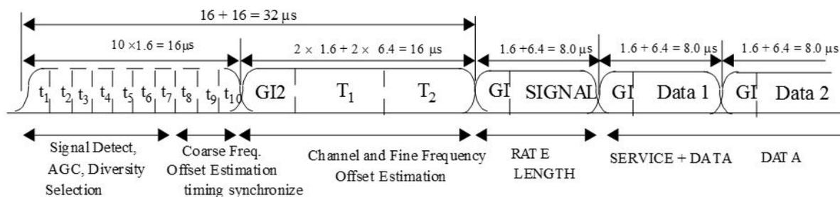
Figure 8: 10 MHz ITS-G5 preamble
