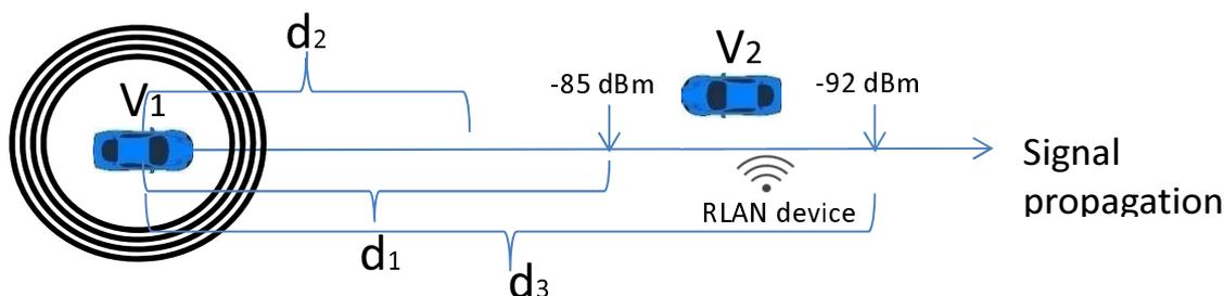
Figure B.19: RLAN interference due to limitation in detecting ITS transmissions
