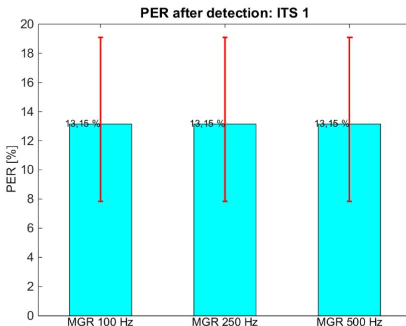
NOTE: Decreased EDCA Plan A method is used. Wi-Fi packet duration is 2,5 ms. Packets use AC\_BE.
