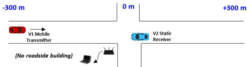
Figure B.30: Scenario - Static ITS Receiver, Mobile ITS transmitter
