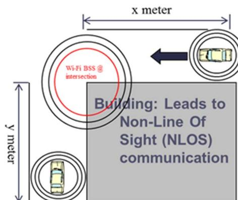
**Figure B.1: Intersection collision avoidance (scenario 1)**
