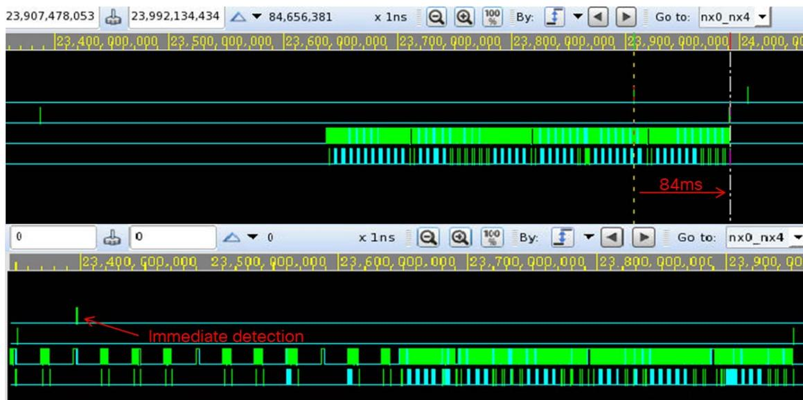
**Figure B.10: Snap shot of simulation comparing detection time of Detect and Vacate and Decreased EDCA Plan B**
