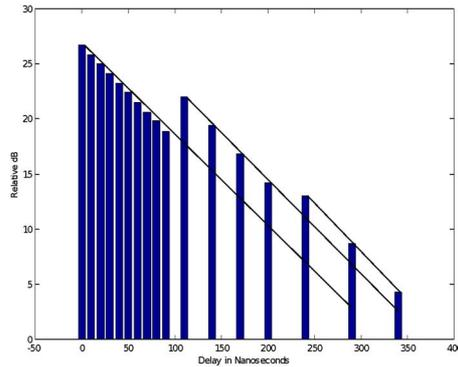
**Figure B.3: Model D delay profile with cluster extension (overlapping clusters)**
