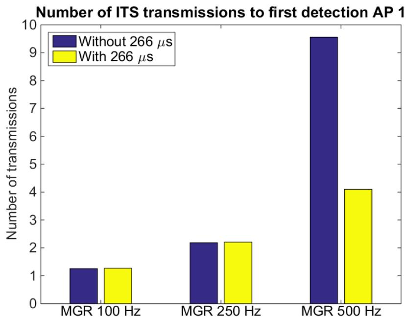
NOTE: Packets use AC\_BE. Each packet lasts 1 ms.
