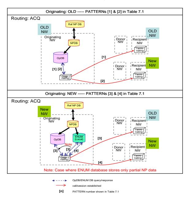
Figure 7.1: Example of call routing/database lookup method for transition type "Solution C => Option 2"
