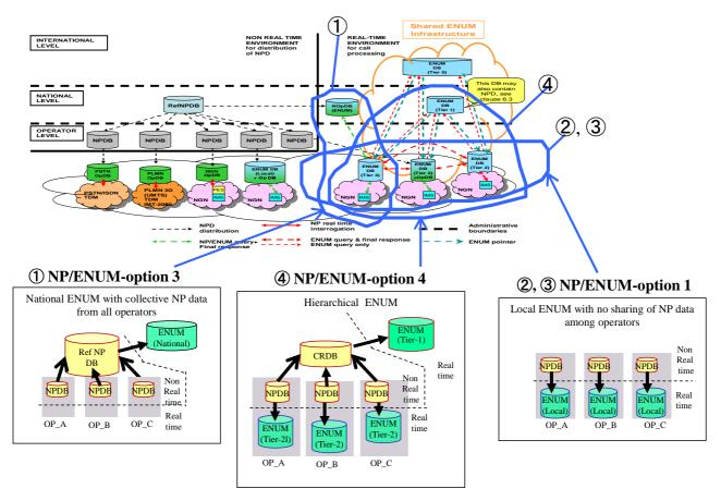
Figure A.4.2: Creating options for ENUM-like solution based on use cases provided in GSMA IR.67 [i.8]
