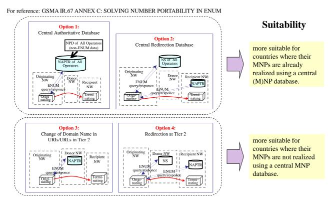
Figure A.2.3: Use cases for ENUM-like mechanisms in GSMA IR.67 [i.8]
