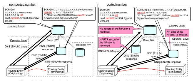
Figure 6.2: Example of call setup process for Hierarchical ENUM (NP/ENUM-option 4)
