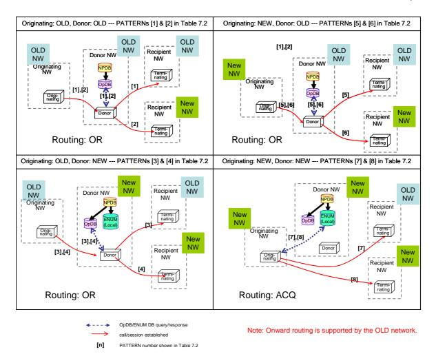
Figure 7.2: Example of call routing/database lookup method for transition type "Solution A => Option 1"
