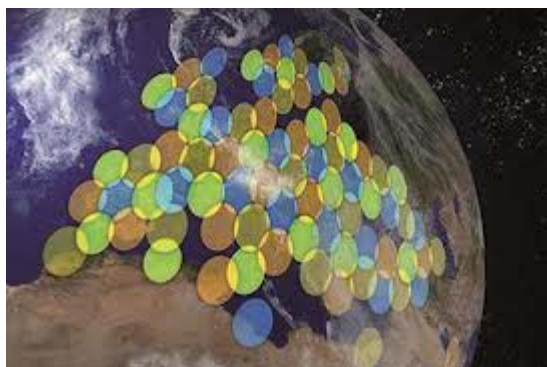
Figure 5: Illustration of a frequency re-use pattern in a multi beam satellite (reuse factor 4)
