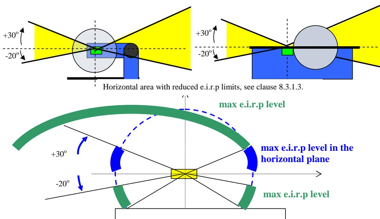
**Figure 18: Restriction on angular sector for material sensing devices**
