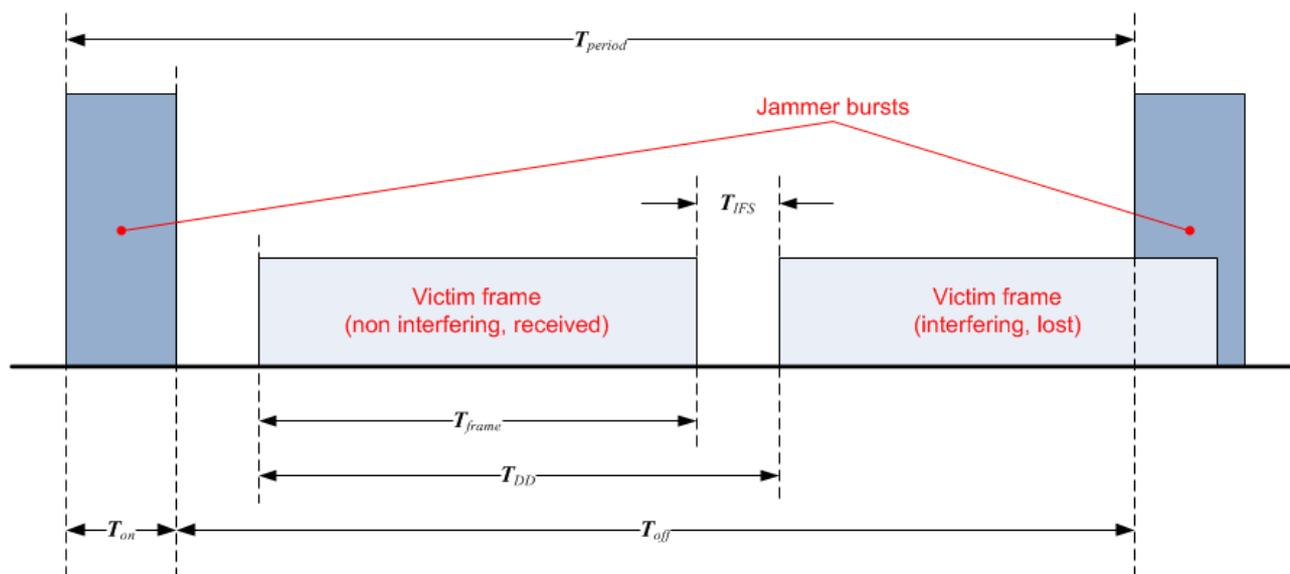
Figure A.1: Exemplary case of interference between a jamming service and a victim service
