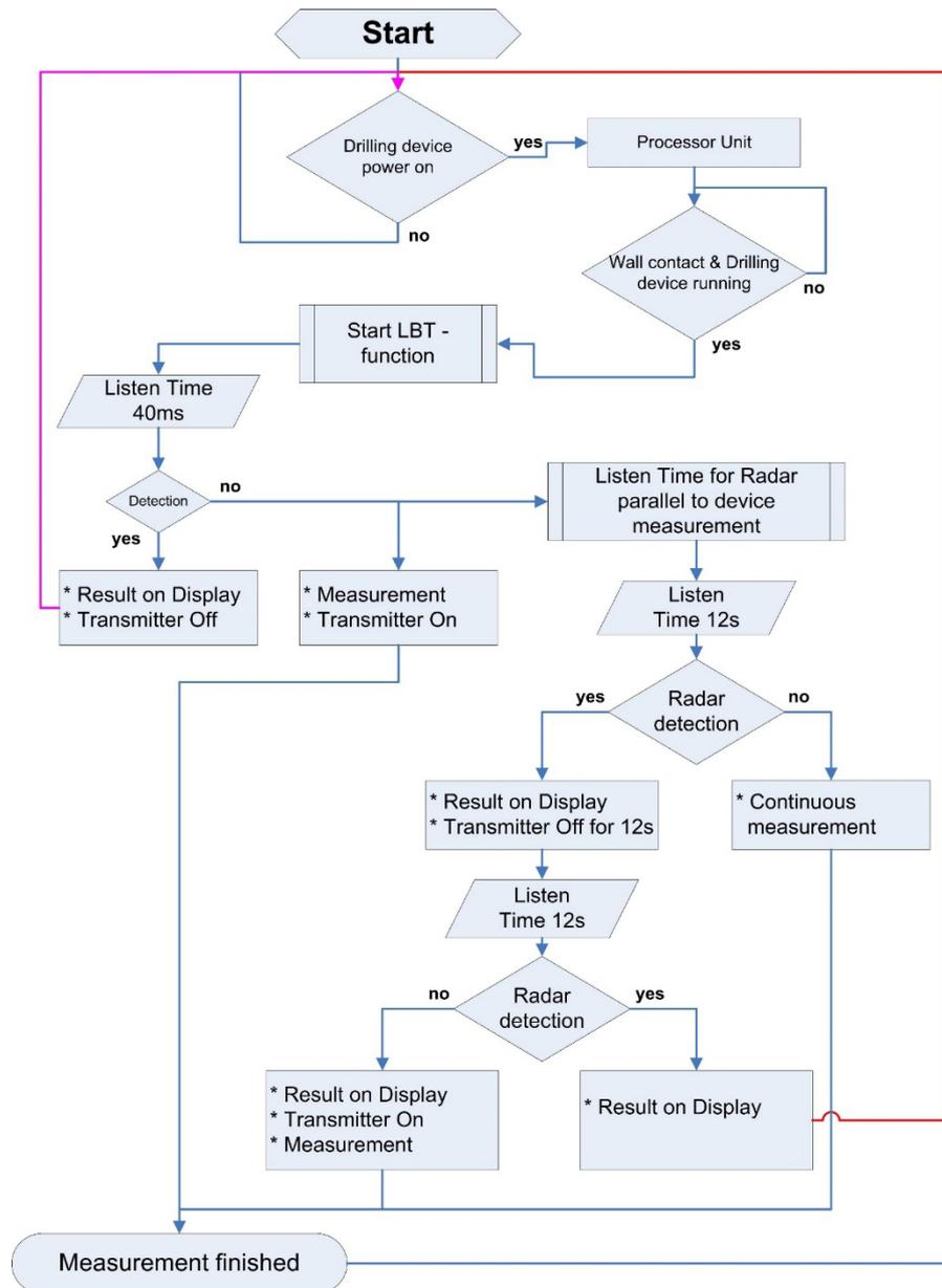
**Figure 3: Flow diagram of LBT mechanism for non-BMA Material Sensing Device, Category B**
