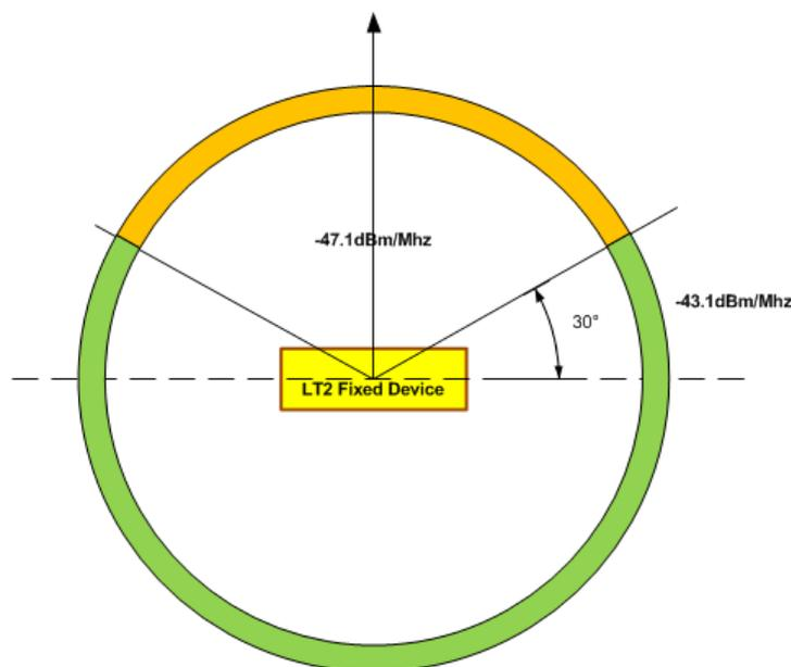
**Figure 17: Emitted power limits for angular sectors for LT2 devices, fixed outdoor**
