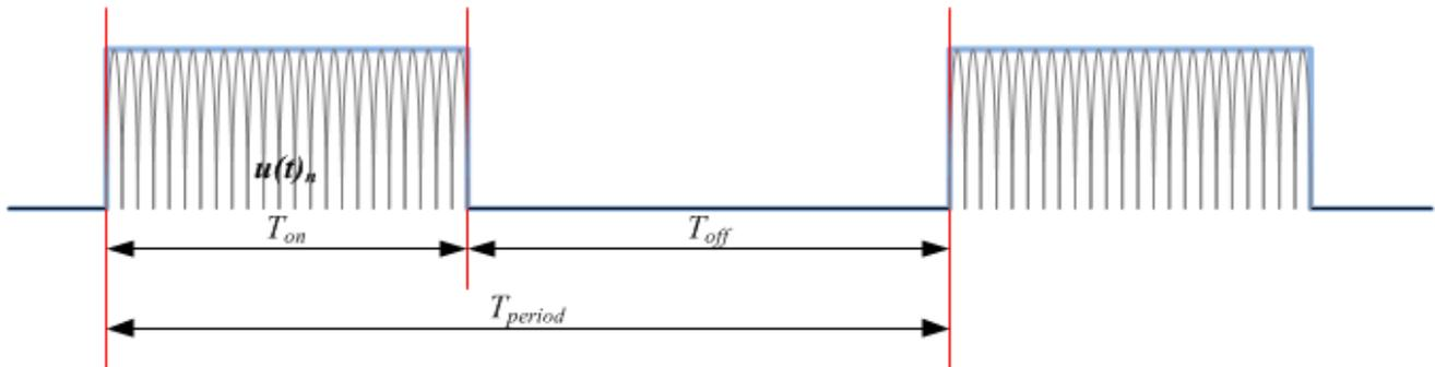
**Figure B.3: Windowed-pulsed signal example for the aggregate mathematical model**
