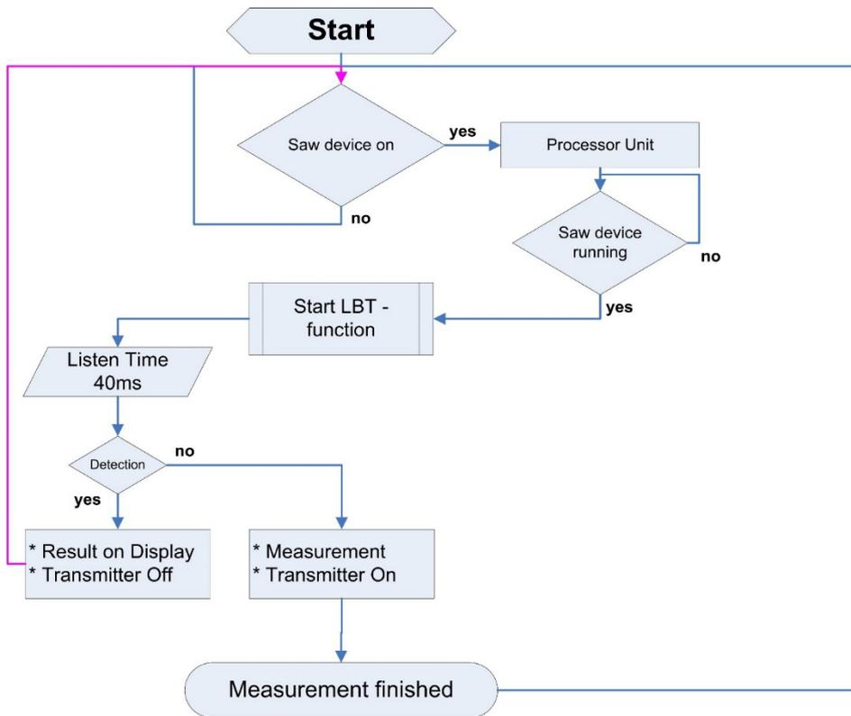
Figure 2: Flow diagram of LBT mechanism for non-BMA Material Sensing Device, Category A
