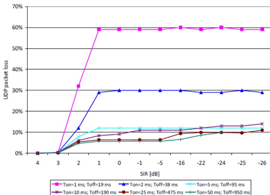
**Figure A.3: UDP packet loss rates versus WiMAX Signal-to-Interference Ratio (SIR) for various pulses, RSSI = -84,6 dBm (from [i.32])**
