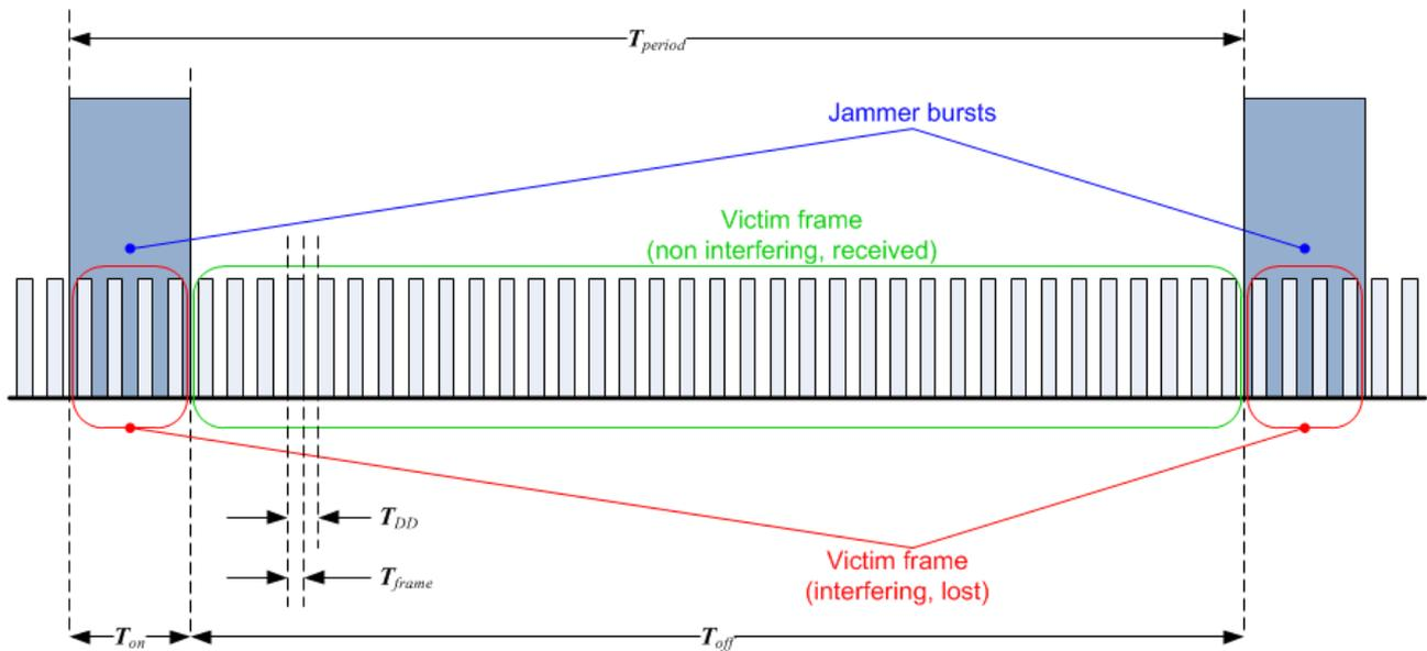
Figure A.4: Collisions when  $T_{\text{on}} \gg T_{\text{frame}}$ , and  $T_{\text{period}} \gg T_{\text{DD}}$ :  $\text{PoC} = T_{\text{on}}/T_{\text{period}}$
