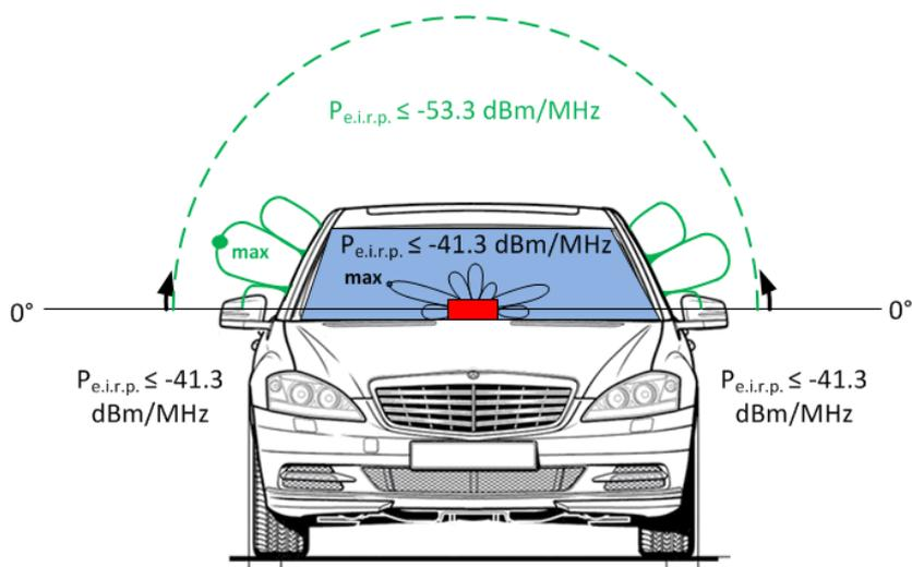
Figure 16: Principle of the regulations [i.25]
