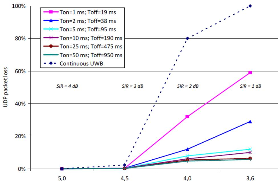
Figure A.2: UDP packet loss versus equivalent distance to interferer (LOS), victim RSSI = -84,6 dBm (from [i.32])
