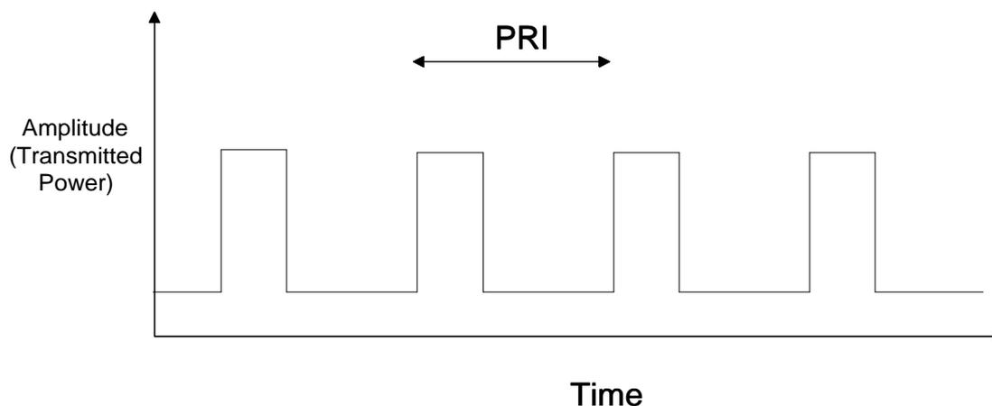
**Figure 13: Typical pulse modulation scheme**
