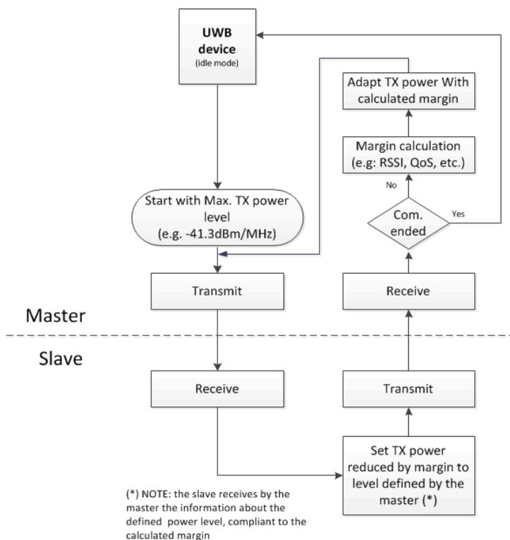
**Figure 10: Option for a master slave application using TPC: the master determines the level of TX power basing on quality of link (e.g. RSSI, QoS, or other link quality indications)**
