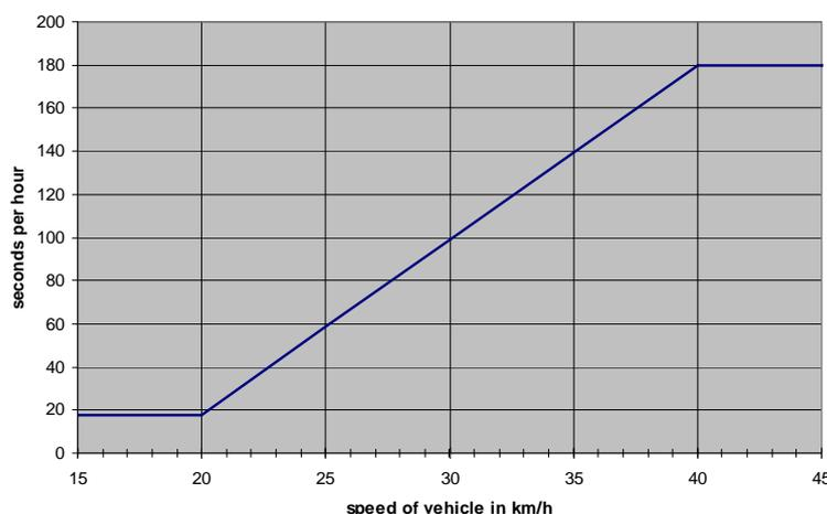
Figure 12: Trading LDC with vehicle speed in EN 302 065-3 [i.25]
