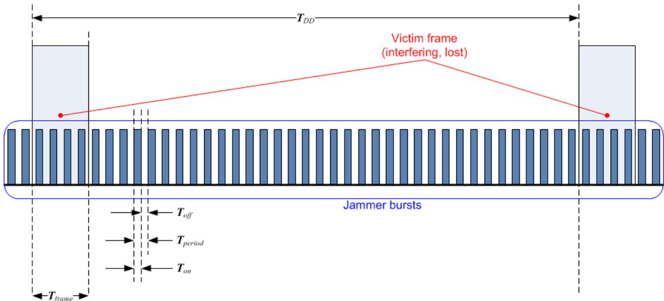
Figure A.5: Collisions when  $T_{\text{on}} \ll T_{\text{frame}}$ , and  $T_{\text{period}} \ll T_{\text{DD}}$ :  $\text{PoC} = 100\%$
