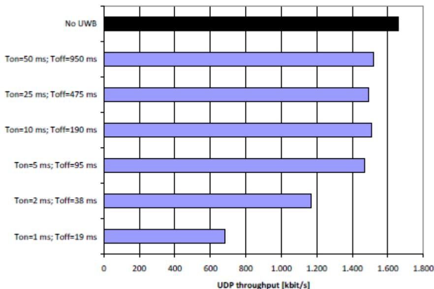
**Figure B.2: WiMAX UDP throughput for different UWB LDC schemes, UWB distance = 0,5 m, RSSI = -90,6 dBm, (Figure 4 from [i.32])**
