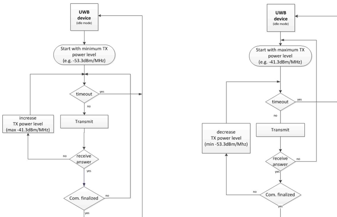
**Figure 9: Two options for a simple application using TPC: start at minimum TX power and start at maximum TX power, then adapt the power to the level required to finalize the communication**
