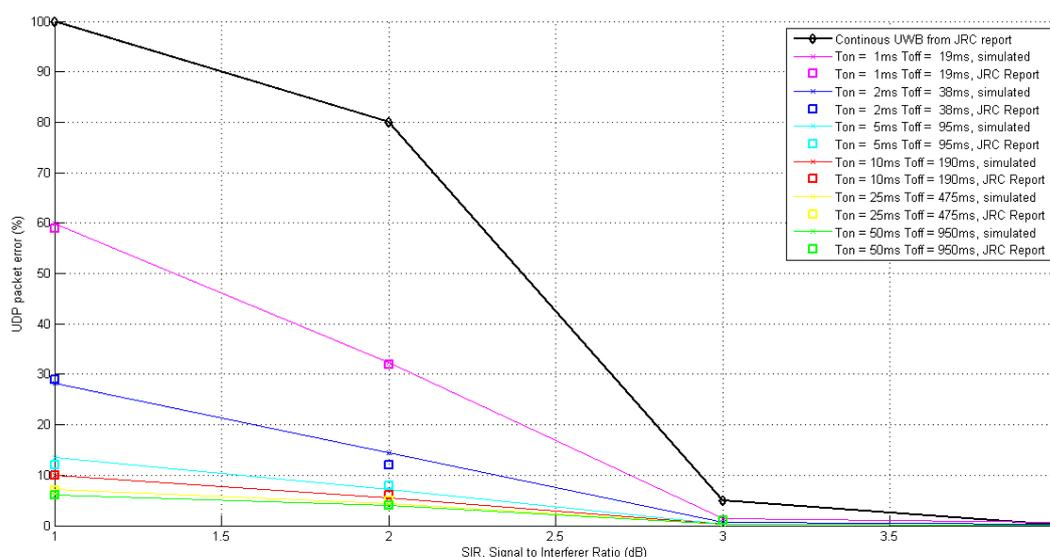
**Figure A.6: Simulations results of WiMAX UDP PER versus SIR, 5 % of duty cycle, compared against the relevant experimental data from [i.32]**
