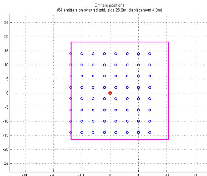
NOTE: Density of emitters is 1 device per 16 m<sup>2</sup>. The red point is the victim receiver.
