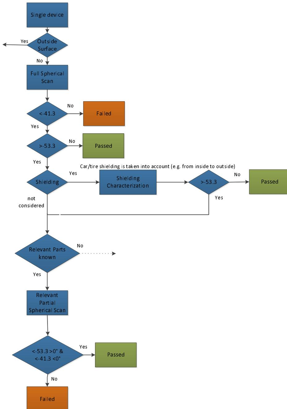
Figure 20: Measurement Flow for devices mounted inside a tyre
