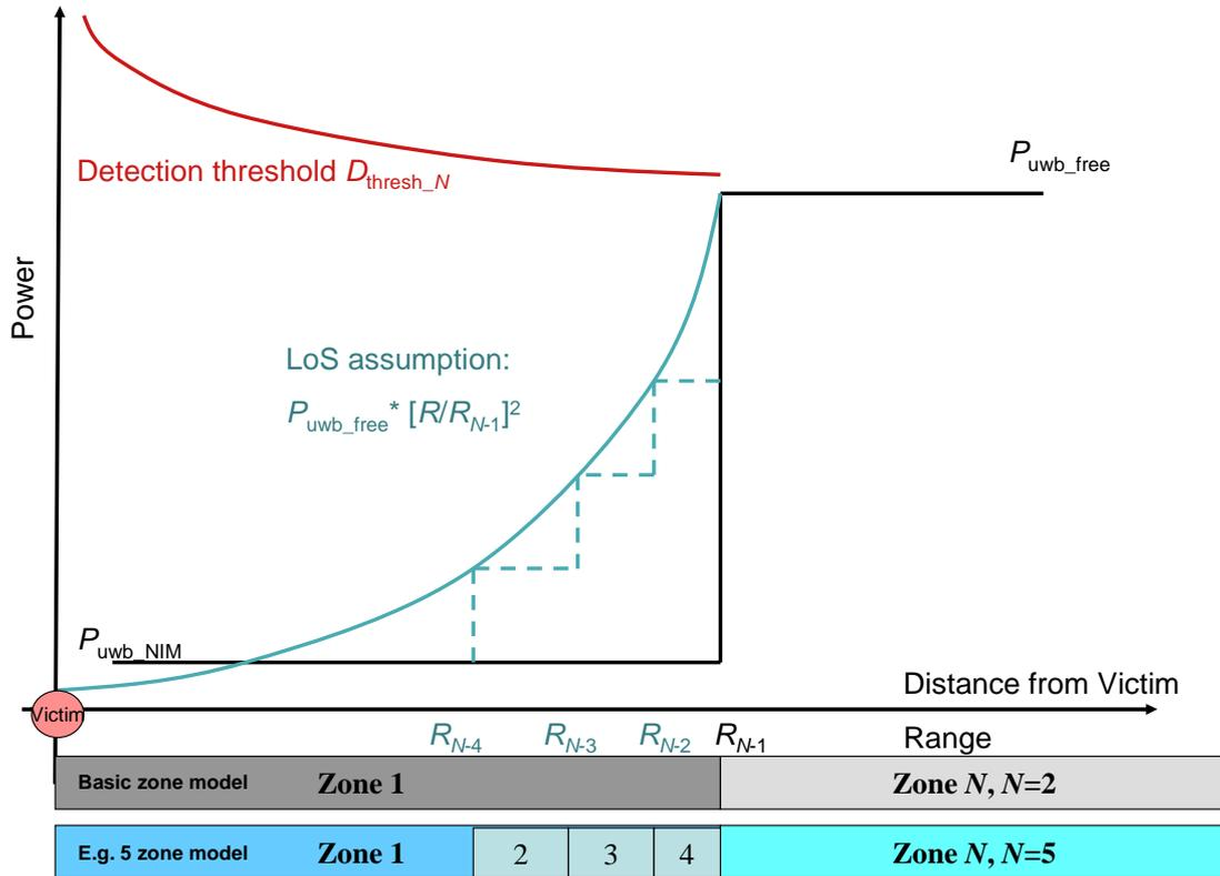
**Figure 6: Illustration of multi zone concept based on equivalent protection levels**
