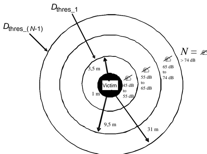
Figure 4: Zone model segmentation and corresponding path loss with LoS distance in meters for  $N = 4$
