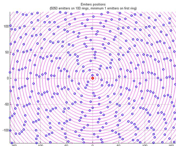
NOTE 1: Density of emitters is 1 device per 200 m<sup>2</sup>.
