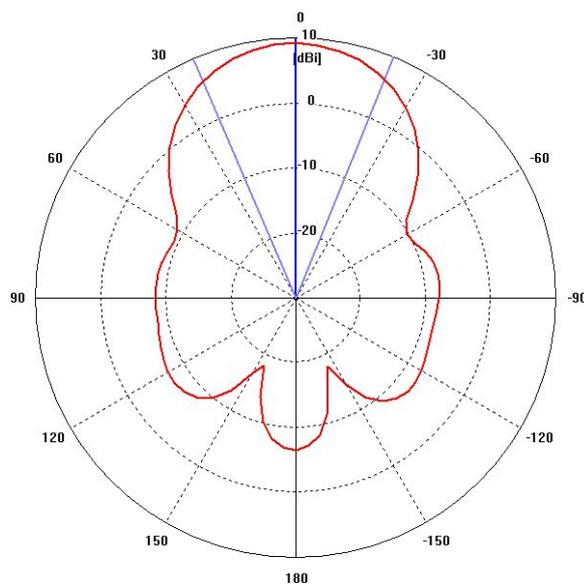
**Figure 15: Example radiation pattern of an antenna in free-space with a directivity of  $D = 9,3$  dBi**
