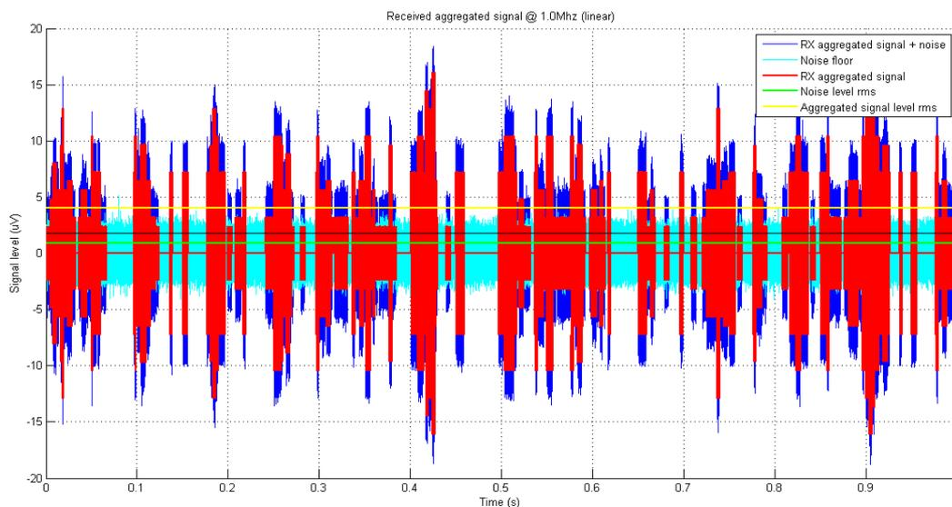
**Figure A.9: Example of aggregate transmission at 1,0 MHz victim receiver. Transmissions may occur when the aggregated signal (red) is below  $V_{guard}$  and they cannot occur in other time intervals**
