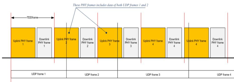
**Figure B.1: Example of distribution of UDP frames over PHY frames**
