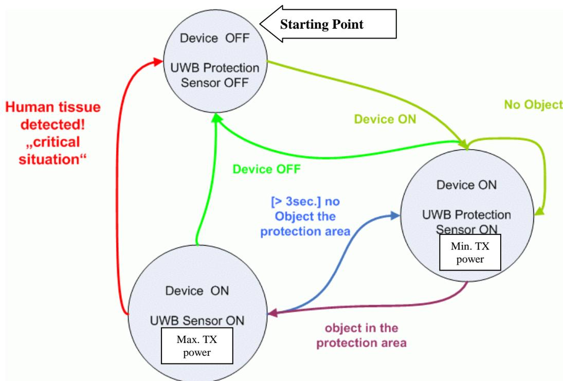
Figure 7: TPC - procedure (for Material Sensing device, fixed installations, from EN 302 498-1 [i.21])
