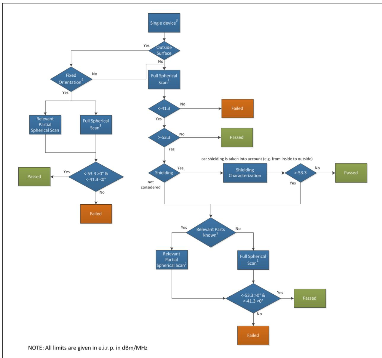
NOTE 1: Full spherical scan to obtain transmission pattern or common measurement method according to TS 102 883 [i.12].
