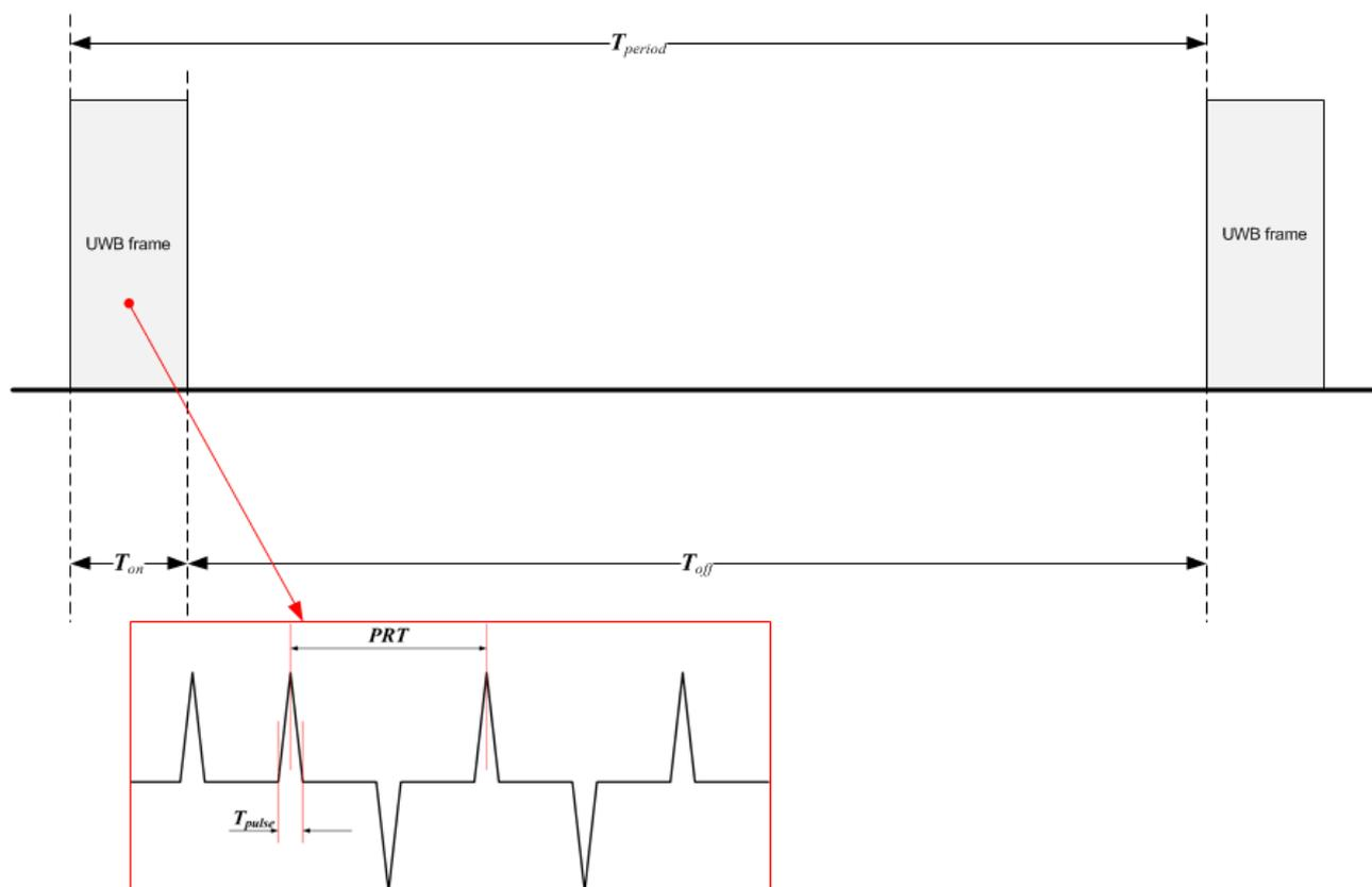
Figure 11: Duty Cycle parameters definition
