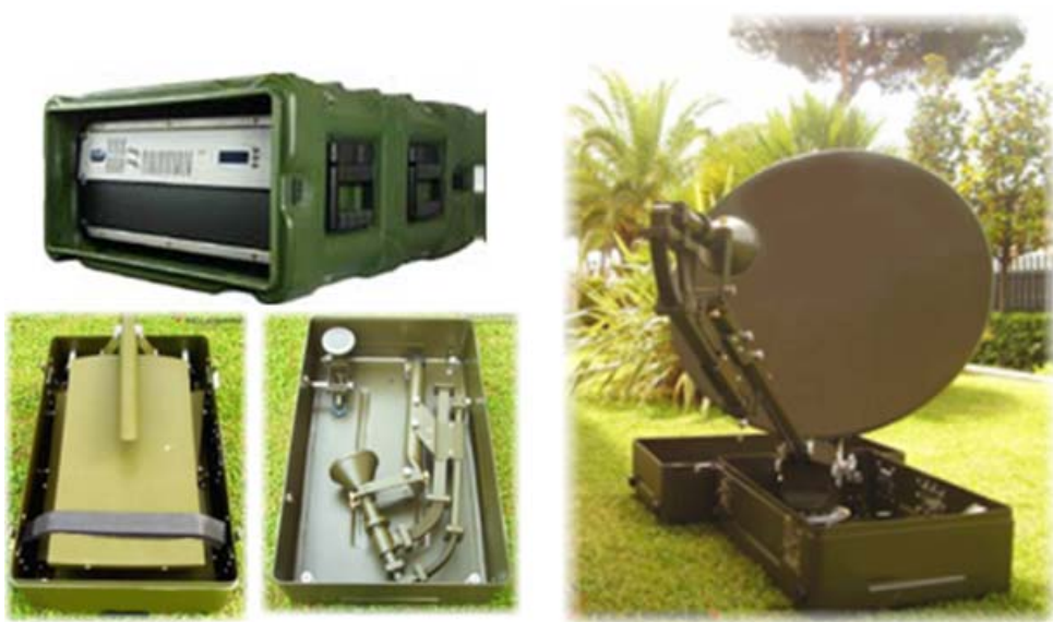
Figure A.13: EMERSAT fly-away satellite terminal
