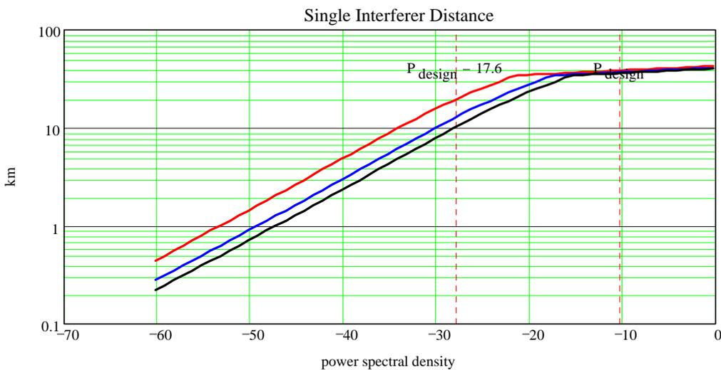
red: transmitter at 5 m above ground, blue, transmitter at 4 m above ground, black: transmitter 2 m above ground.
