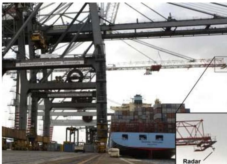
**Figure B.19: Anti-collision system for Ship to Shore cranes**
