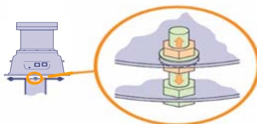
**Figure C.2: Levelling adjustment on threaded mounting bolts**
