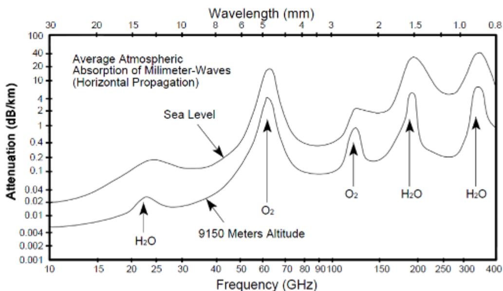
**Figure 4: Atmospheric absorption of millimetre waves**
