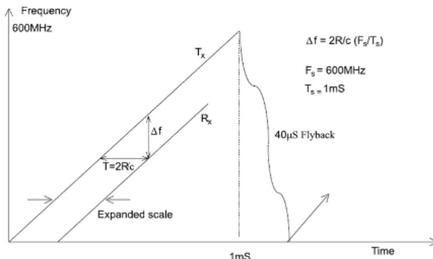
Figure A.2: Typical modulation scheme for a fixed infrastructure radar
