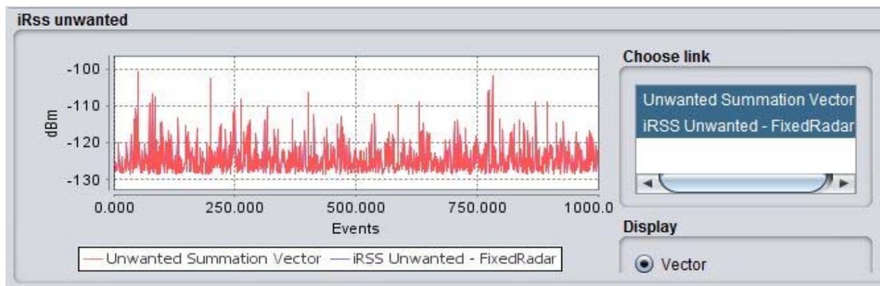
**Figure D.2: Simulated interfering signal from the fixed radar**
