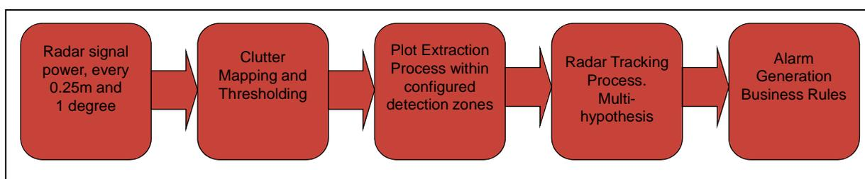
Figure A.1: Radar signal processing chain
