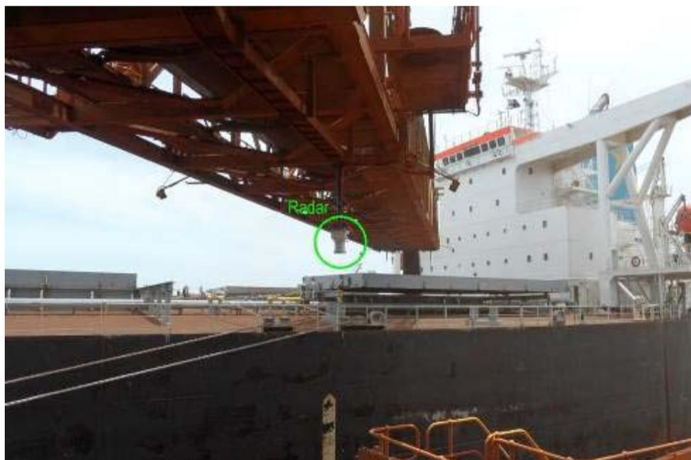
**Figure B.21: Anti-collision system for bulk loader**
