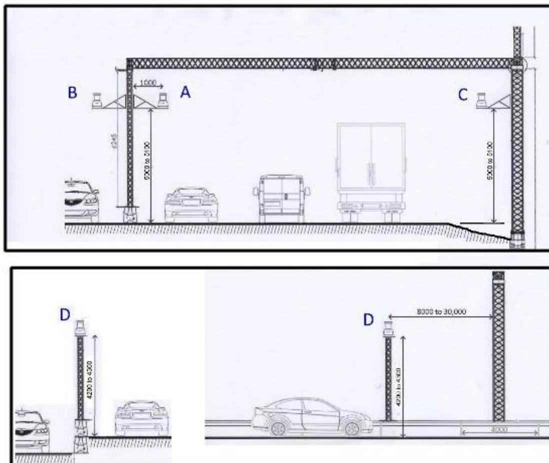
**Figure C.1: Example radar sensor locations,**
