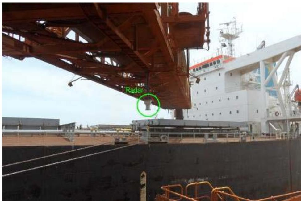
**Figure B.21: Anti-collision system for bulk loader**
