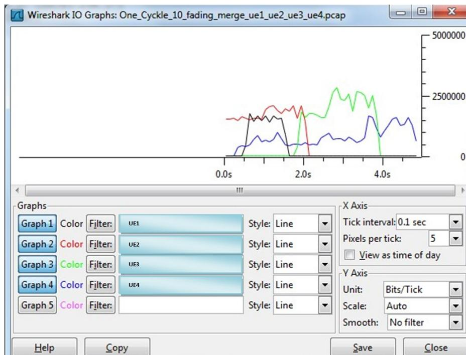
Figure 17: Received data at UEs with activity load 10 % and fading
