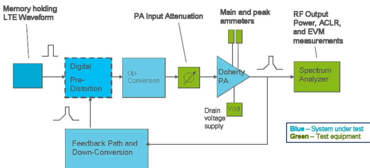
**Figure A.6: Lab setup**
