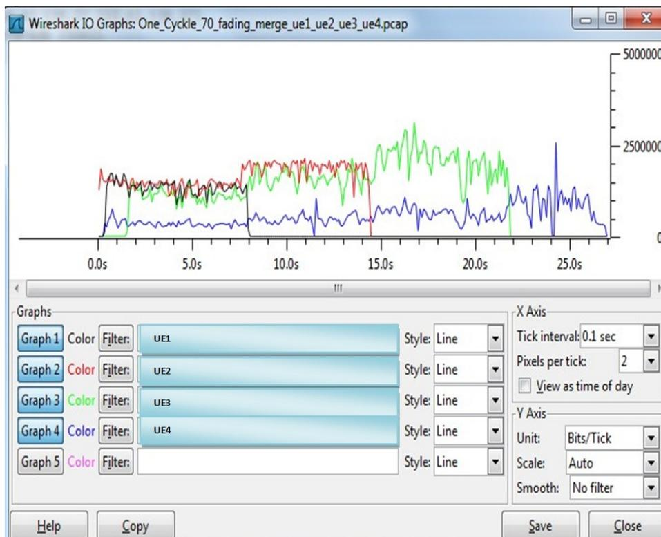
Figure 19: Received data at UEs with activity load 70 % and fading
