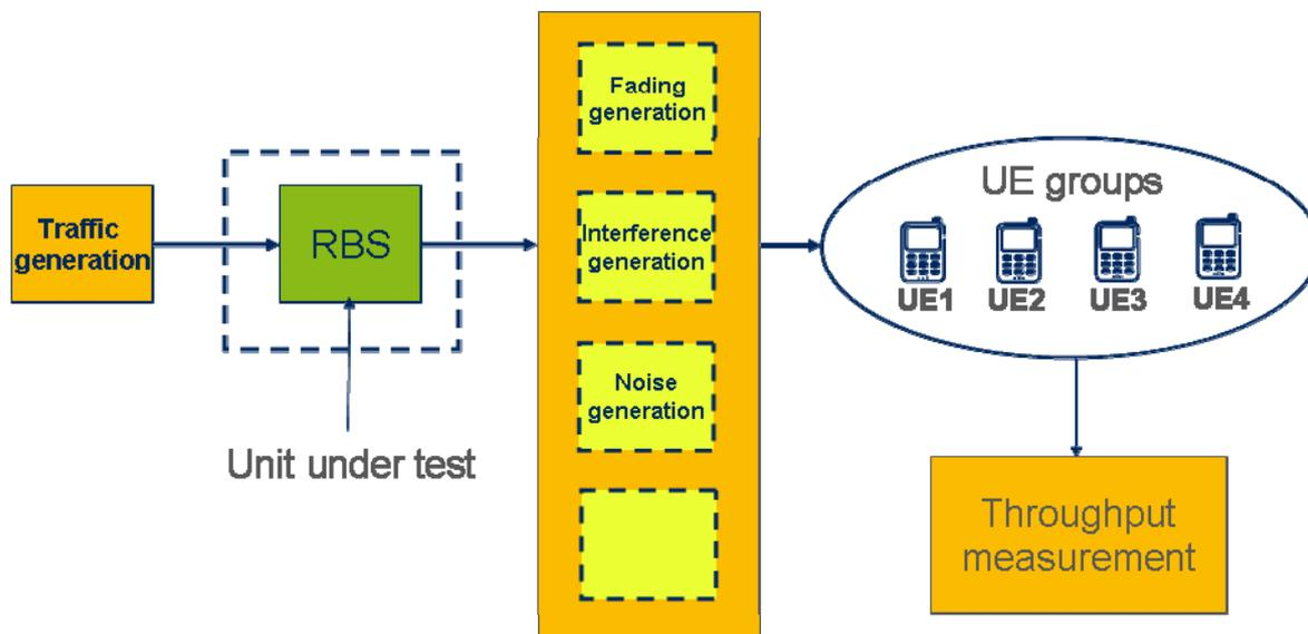
Figure A.8: Realistic test setup proposal
