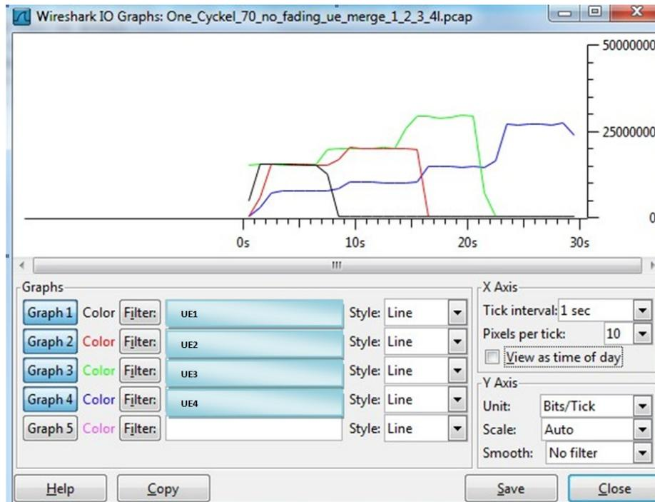
Figure 16: Received data at UEs with activity load 70 % and no fading
