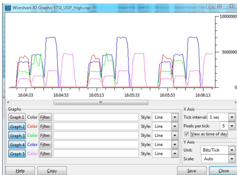
**Figure 11: Measured received data rate at 4 UEs placed in different positions in the cell without any fading present in the channel**
