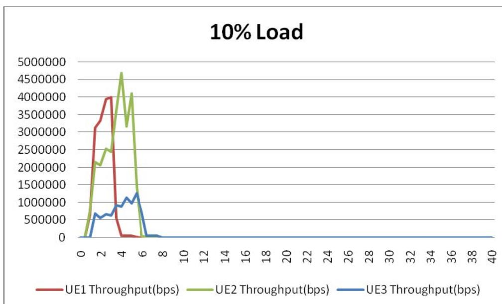
**Figure 2: Test results under 10 % load for WCDMA (Y axis: Throughput (bps) vs. X axis: Time (sec))**
