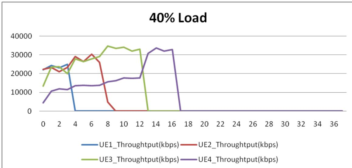
Figure 6: Test results under 40 % load for LTE (Y axis:Throughput (kbps) vs X axis:Time (sec))
