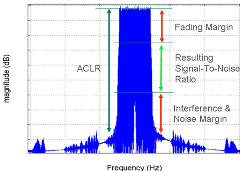
Figure A.5: Resulting signal-to-noise ratio by adding radio effects to the radio channel
