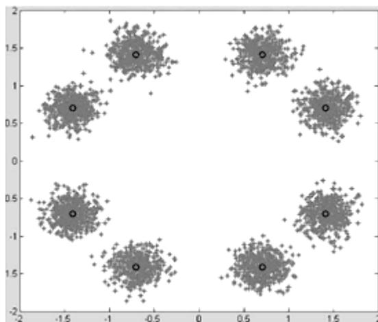
**Figure A.2: 8PSK ( $3\pi/8$ ) modulation, used in radio technologies such as GSM EDGE, showing ideal constellation points and the decoded constellation points within a noisy environment**
