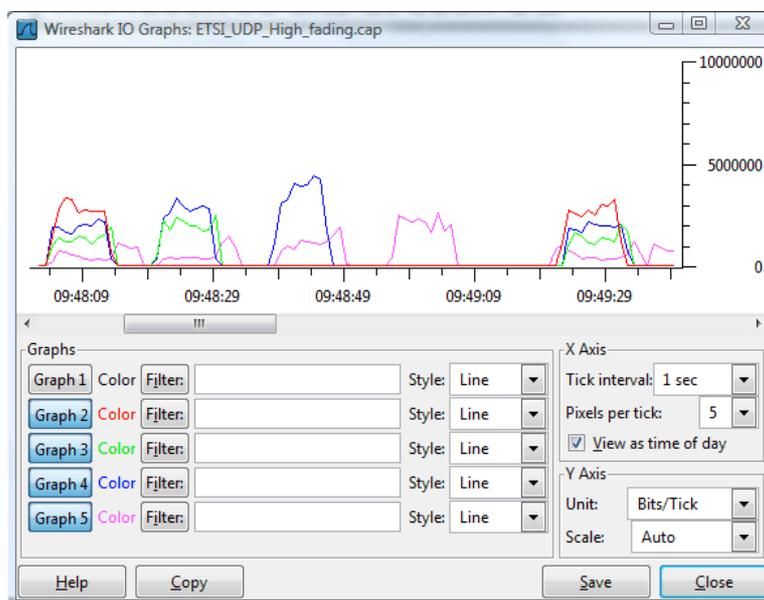
**Figure 12: Measured received data rate at 4 UEs placed in different positions in the cell with fading present in the channel**
