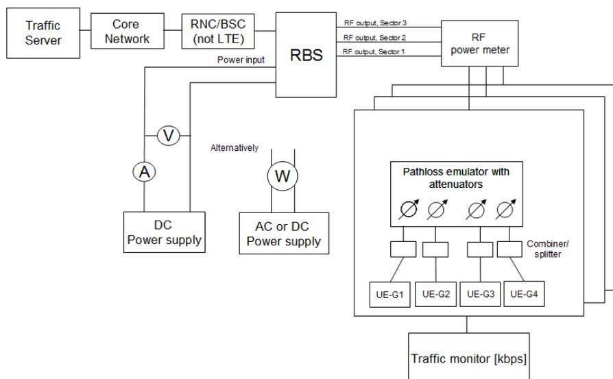
**Figure 1: Test setup for dynamic measurement with UEs (example for three sectors)**
