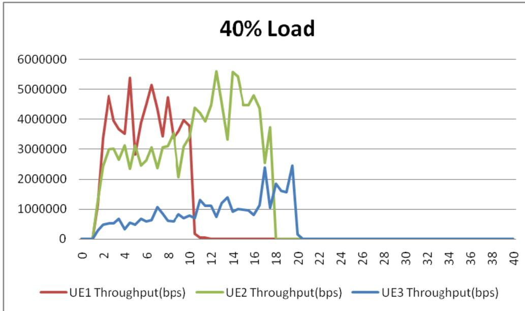
Figure 3: Test results under 40 % load for WCDMA (Y axis: Throughput (bps) vs. X axis: Time (sec))
