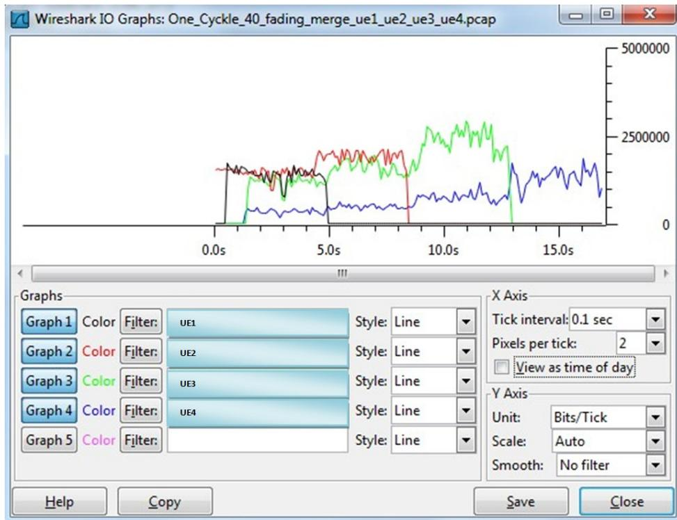
Figure 18: Received data at UEs with activity load 40 % and fading
