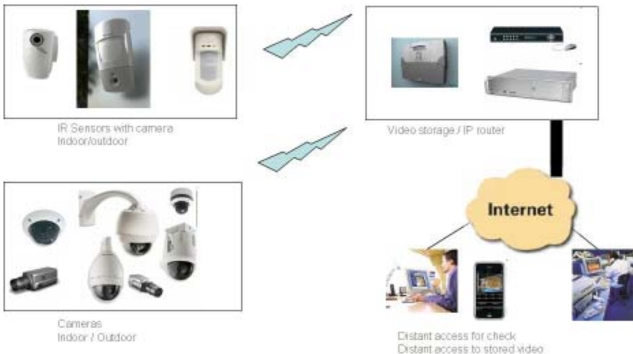
Figure A.4.1: Principle for a wireless image transmission system
