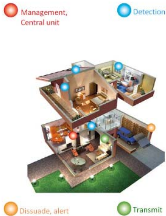
Figure 5.9: Principle of a private building intrusion / security system
