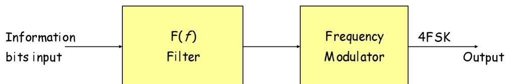
Figure 9.2: 4FSK Modulator
