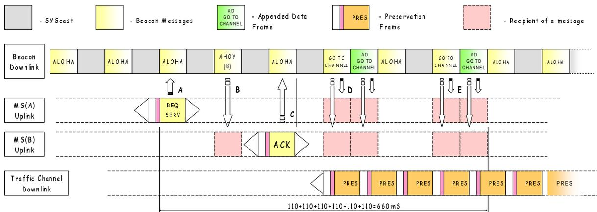
**Figure 6.5: Mode 3 Beacon Channel Individual Voice Call Set-up**
