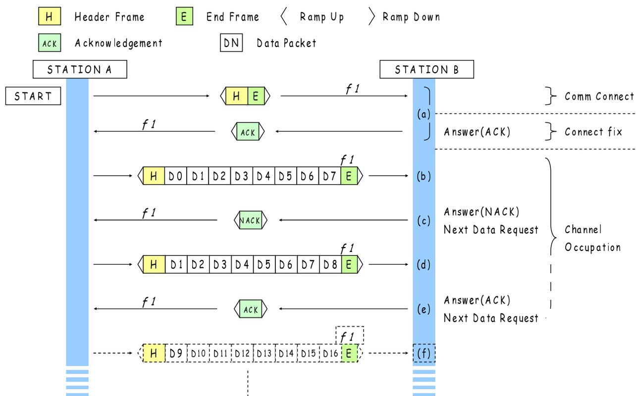
**Figure 6.10: Packet retransmissions**
