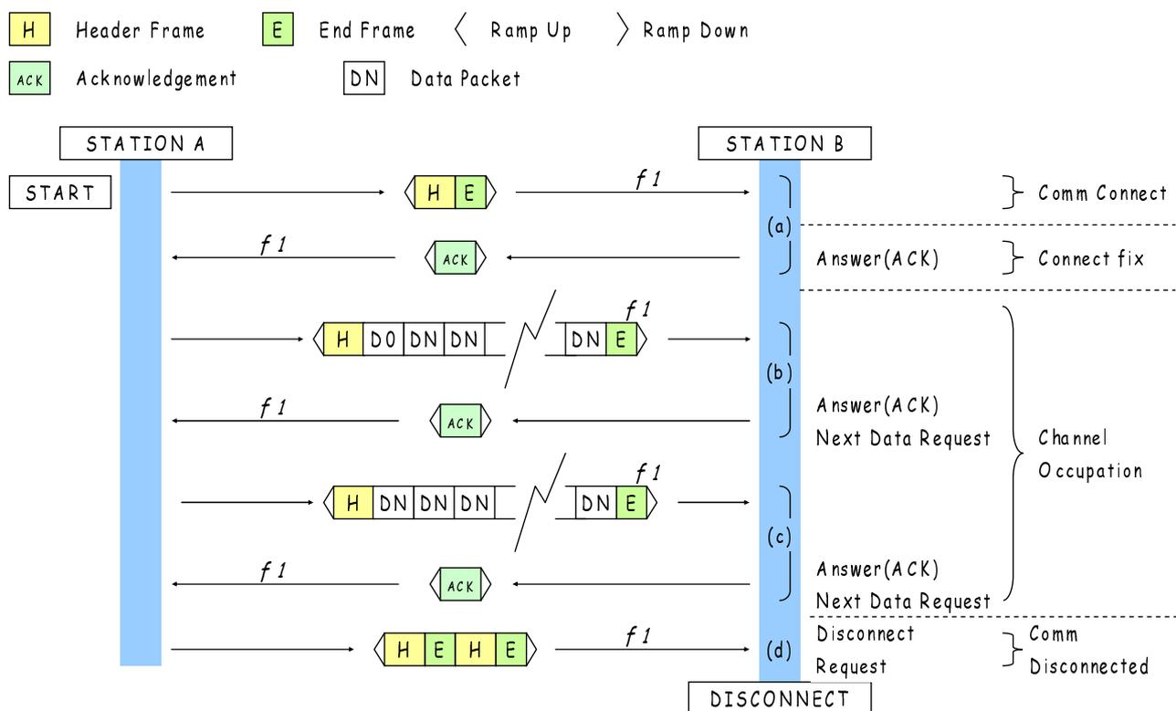
**Figure 6.9: Packet exchanges**
