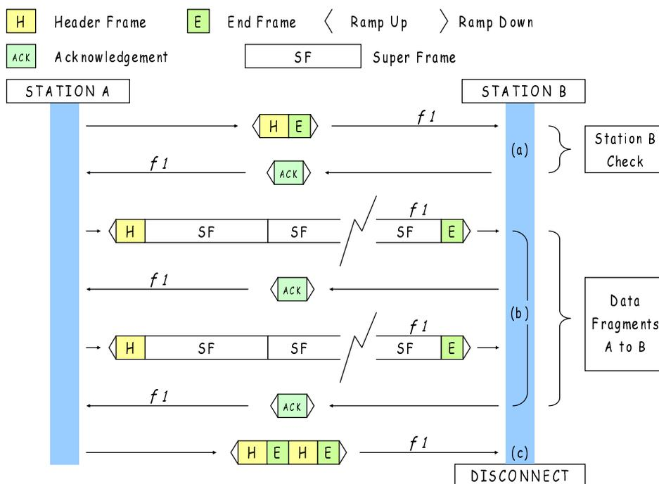
**Figure 6.3: Mode 1 Individual data call exchanges**
