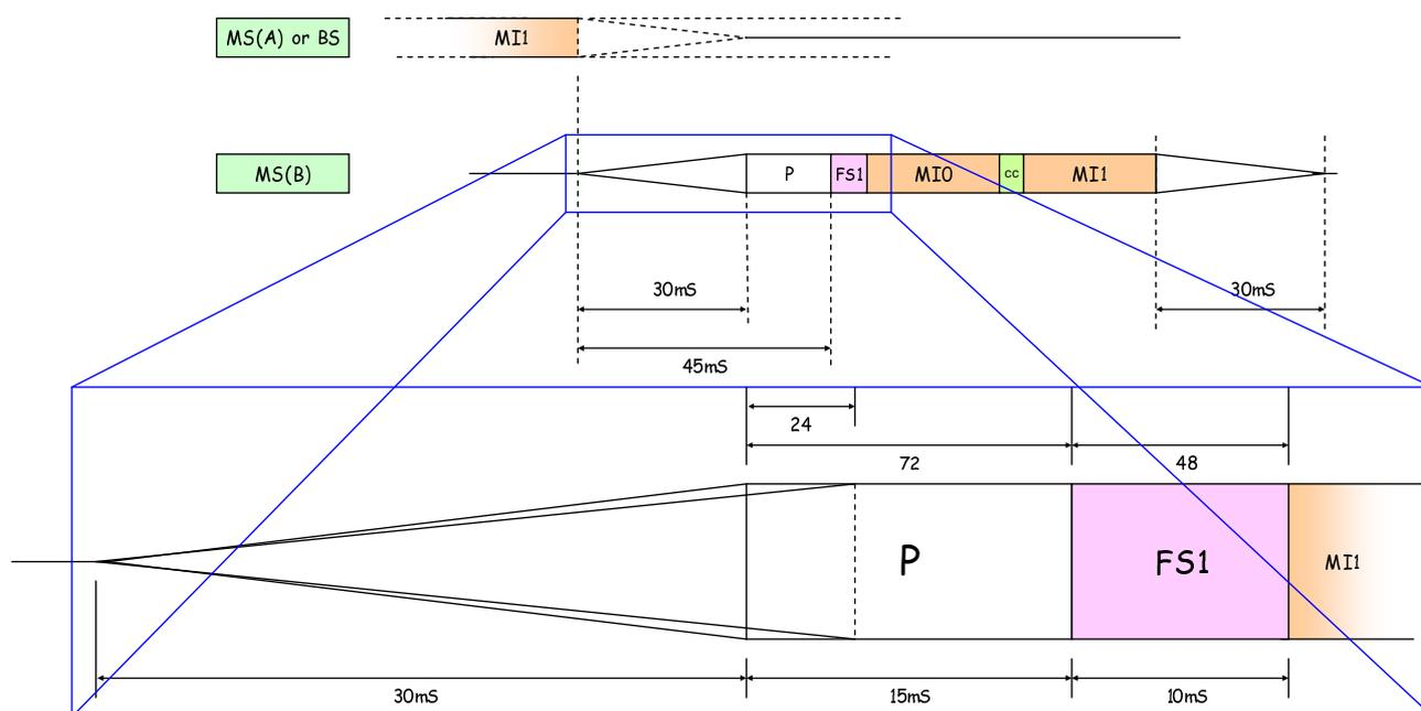
Figure 9.3: Preamble Timing
