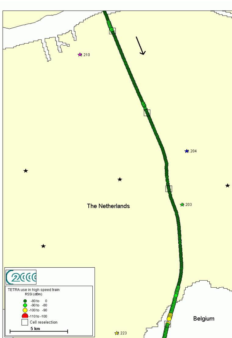
**Figure 13: Received Signal Strength Indication (dBm)**
