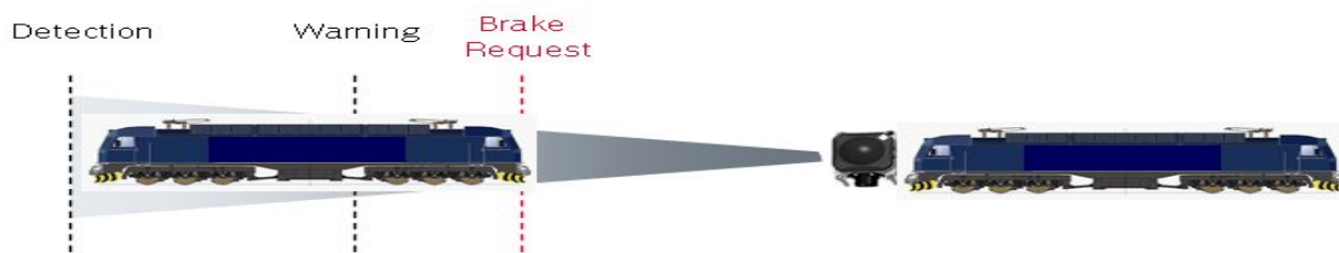
Figure A.2.1.1.7: Phases of track free detection, example for 2 locomotives and platooning
