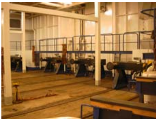
Figure A.2.1.1.5: Collision avoidance locomotive or wagon to crash element e.g. on a ferry
