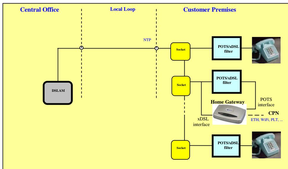
**Figure 4: Total replacement of PSTN by VoIP telephony (distributed filtering architecture)**
