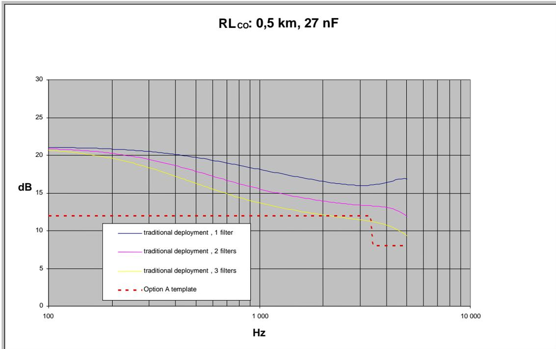
NOTE: Cable length: 0,5 km. Low capacity microfilters.
