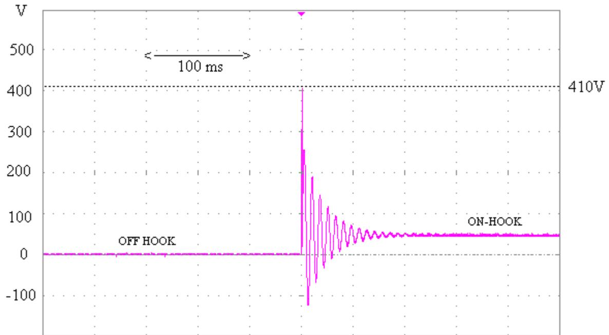
**Figure 28: On/off-Hook transients. Re-injection scenario. One microfilter.**
