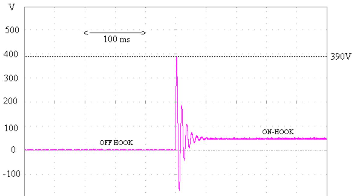
**Figure 28: On/off-Hook transients. Re-injection scenario. Two microfilters.**
