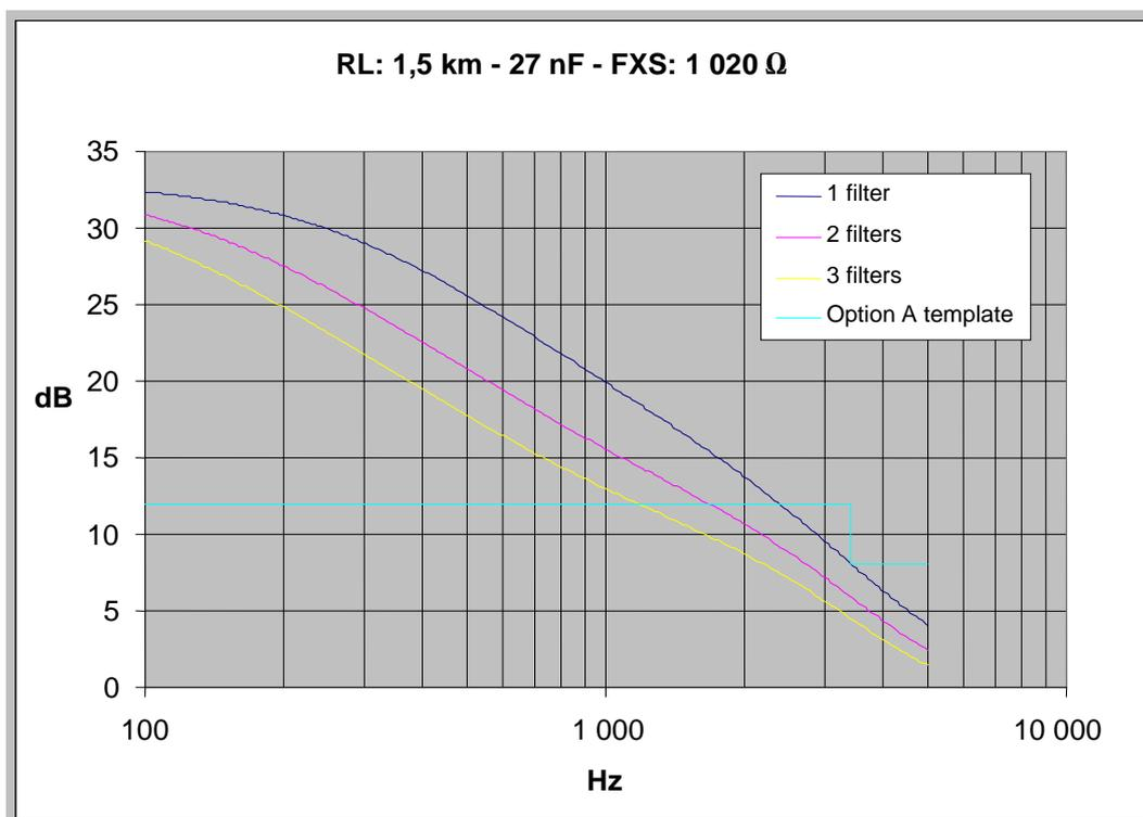
**Figure B.15: Return Loss (with respect to  $Z_R$ ) of impedances presented at the TE port (FXS = 1 020  $\Omega$ ) - 1,5 km local loop**
