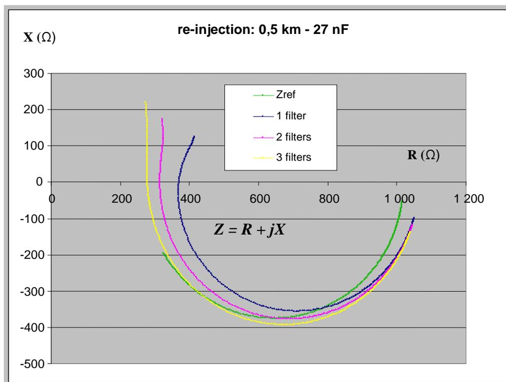
Figure B.1: Impedances presented at the FXS port - 0,5 km local loop
