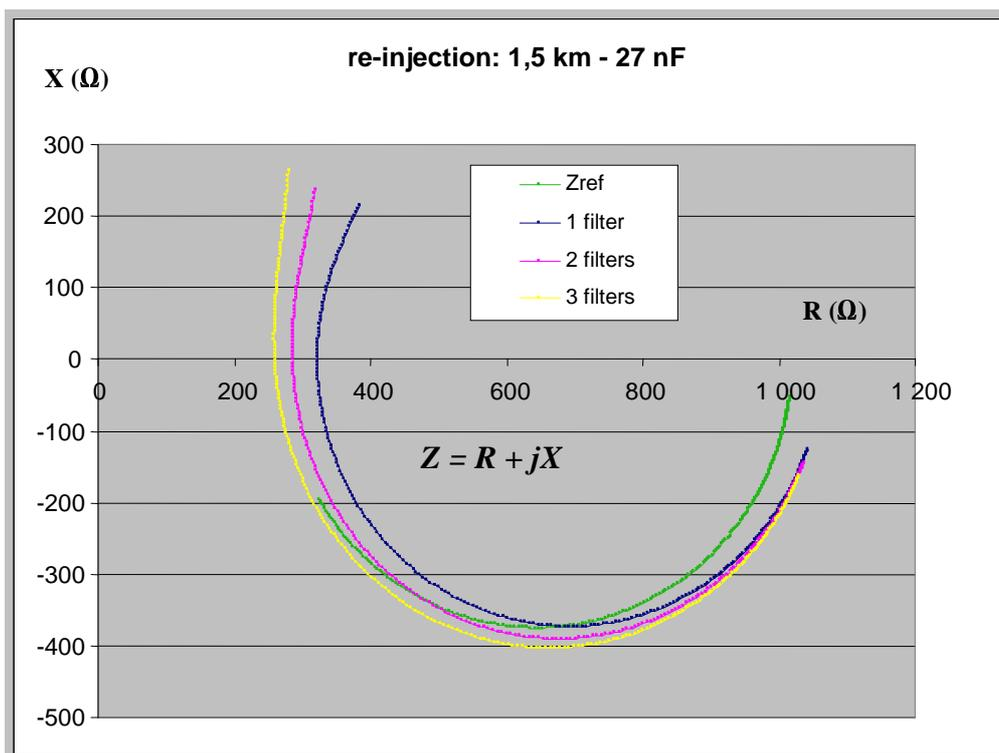
Figure B.11: Impedances presented at the TE port for  $FXS=Z_R$  - 1,5 km local loop
