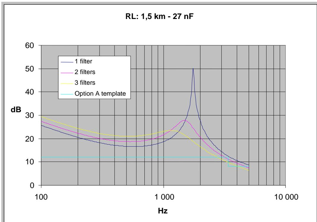
**Figure B.9: Return Loss (with respect to  $Z_{bal}$ ) of impedances presented at the FXS port - 1,5 km local loop**
