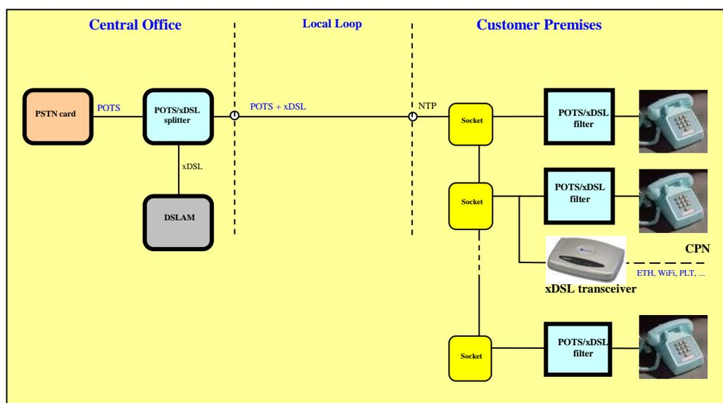
Figure 3: Functional diagram of a typical xDSL platform based on distributed filtering
