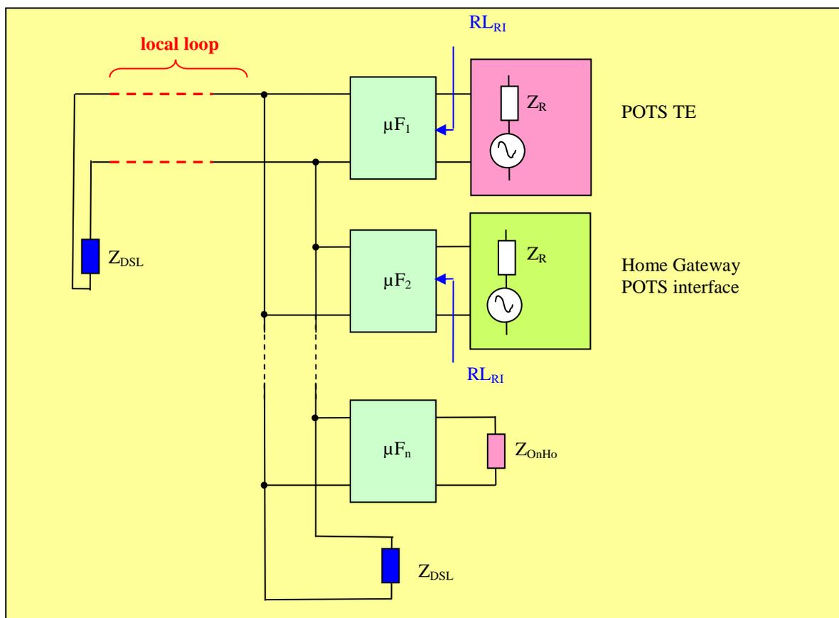
Figure 6: POTS transmission path of xDSL deployment with VoIP re-injection
