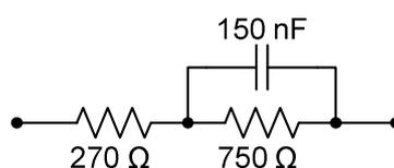
Figure A.2: Impedance  $Z_{\text{R}}$
