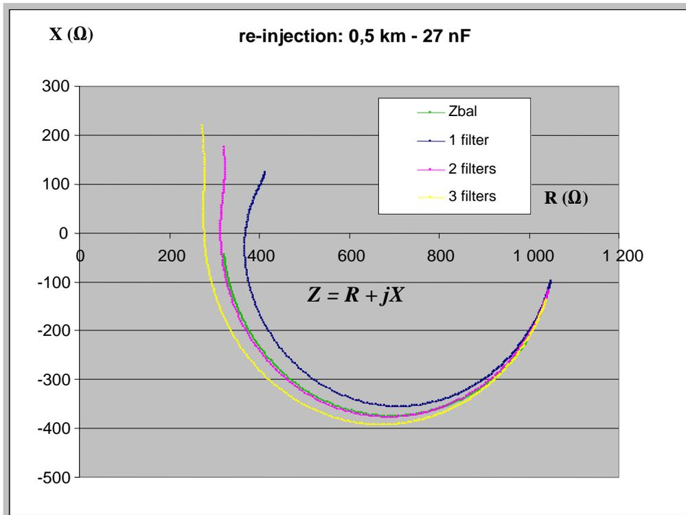
Figure B.6: Impedances presented at the FXS port, comparison with new balance impedance  $Z_{bal}$  - 0,5 km local loop
