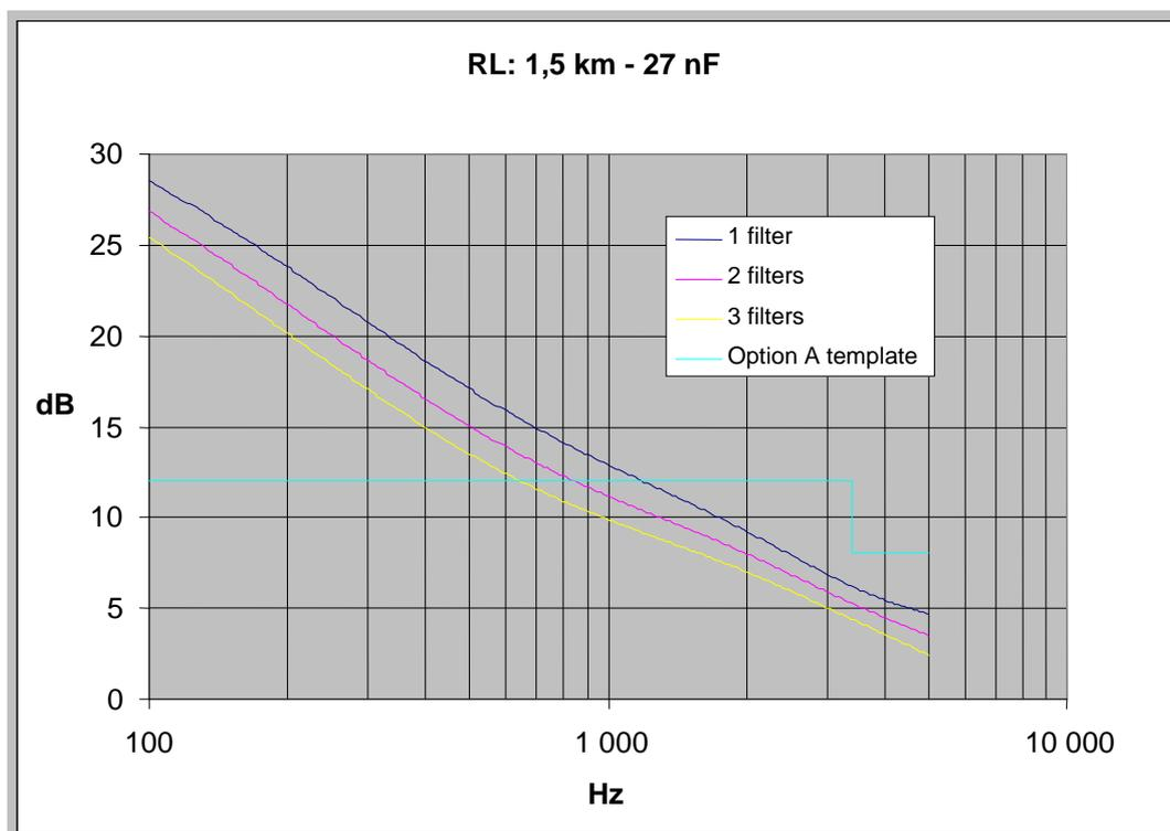
**Figure B.4: Return Loss (with respect to  $Z_R$ ) of impedances presented at the FXS port - 1,5 km local loop**
