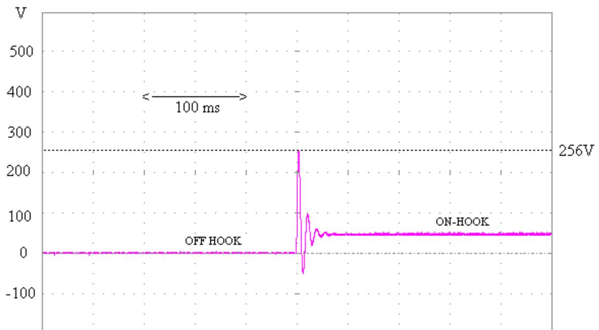
Figure 27: On-Hook transient. Traditional xDSL deployment. Three microfilters.
