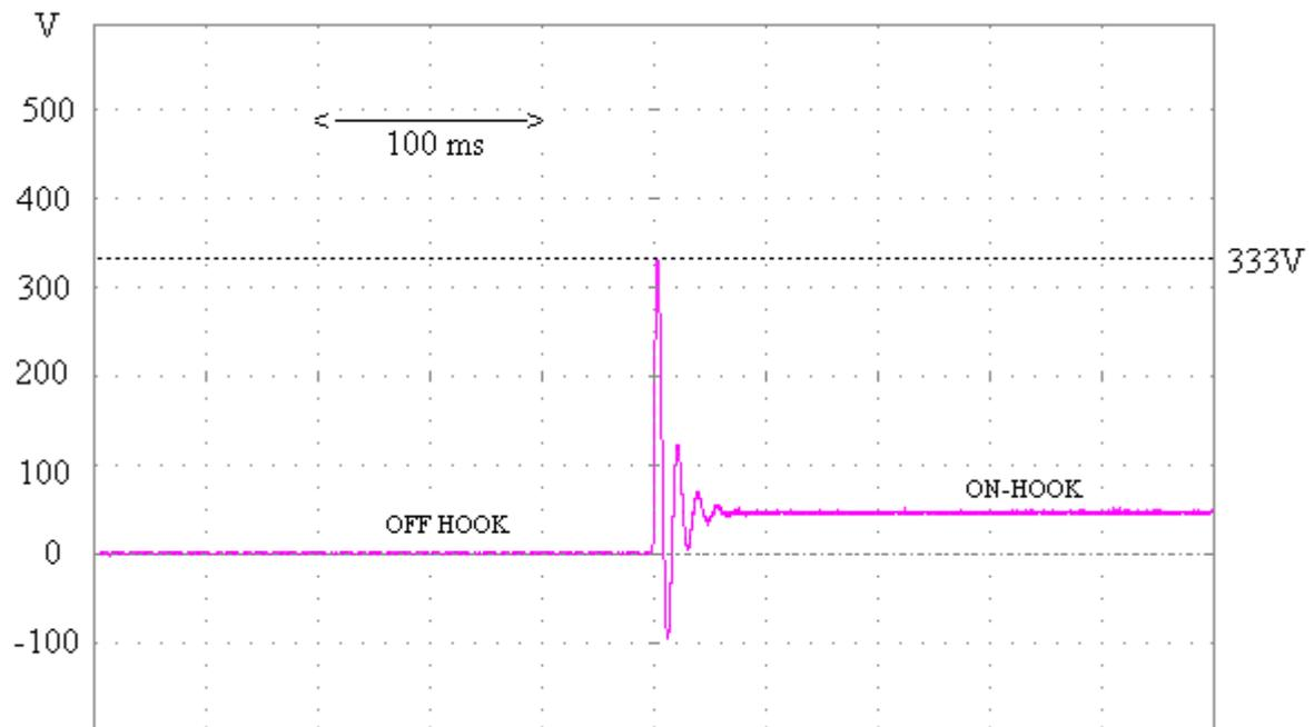
Figure 30: On/off-Hook transients. Re-injection scenario. Three microfilters.
