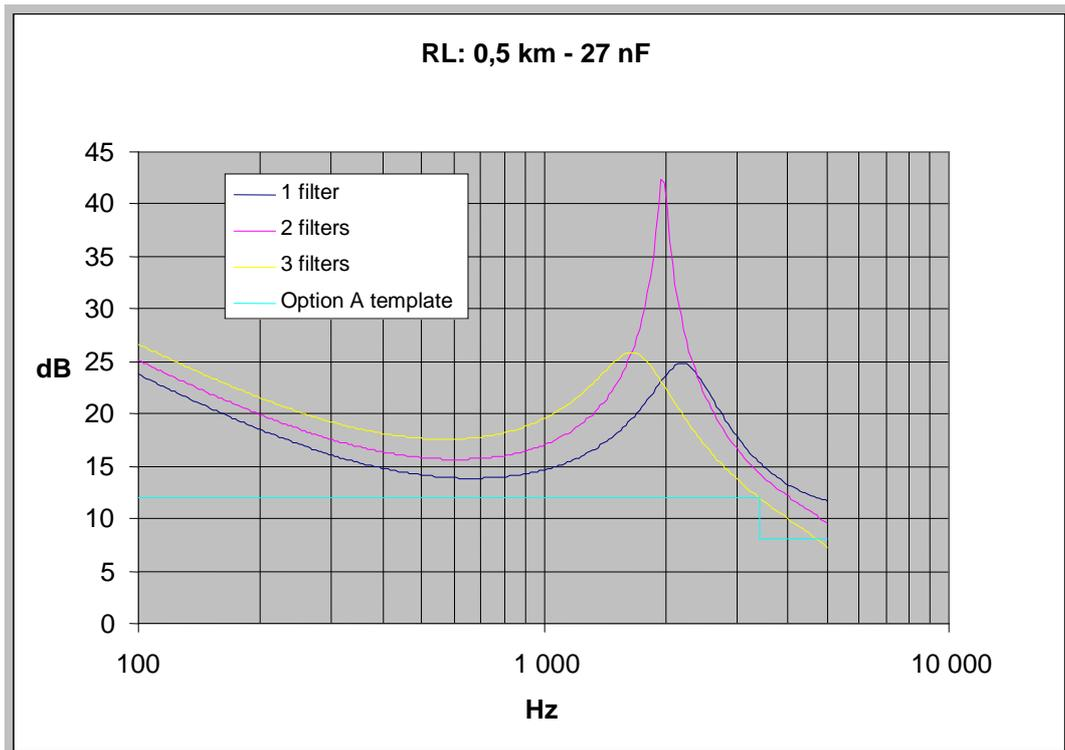
**Figure B.8: Return Loss (with respect to  $Z_{bal}$ ) of impedances presented at the FXS port - 0,5 km local loop**
