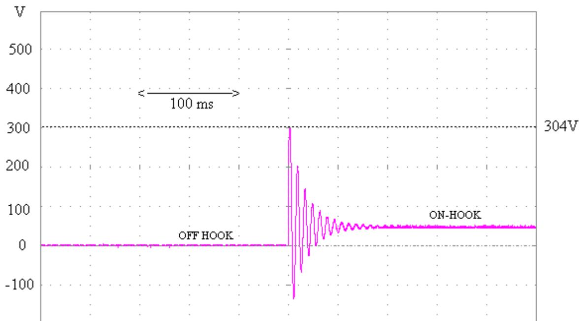
Figure 25: Off/on-Hook transients. Traditional xDSL deployment. One microfilter.
