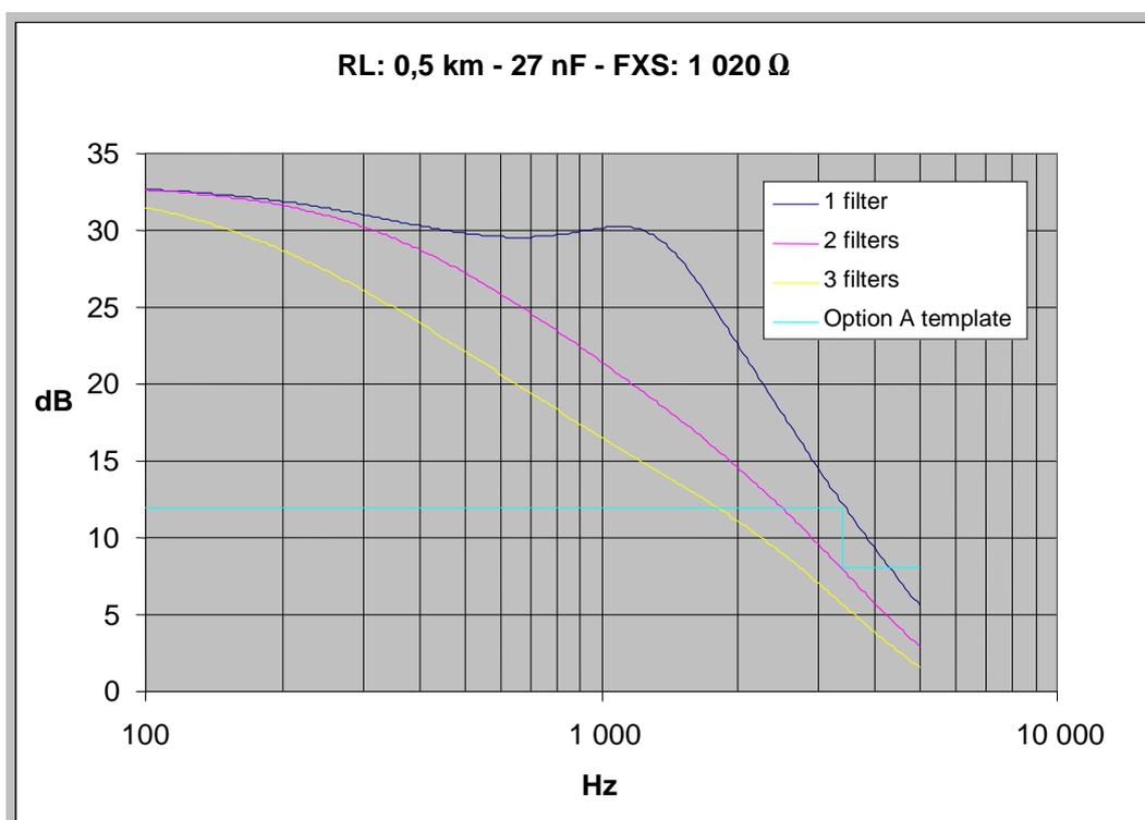
Figure B.14: Return Loss (with respect to  $Z_R$ ) of impedances presented at the TE port (FXS = 1 020 Ω) - 0,5 km local loop
