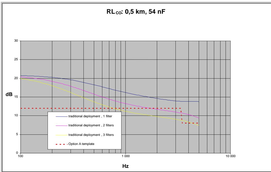
NOTE: Cable length: 0,5 km. High capacity microfilters.
