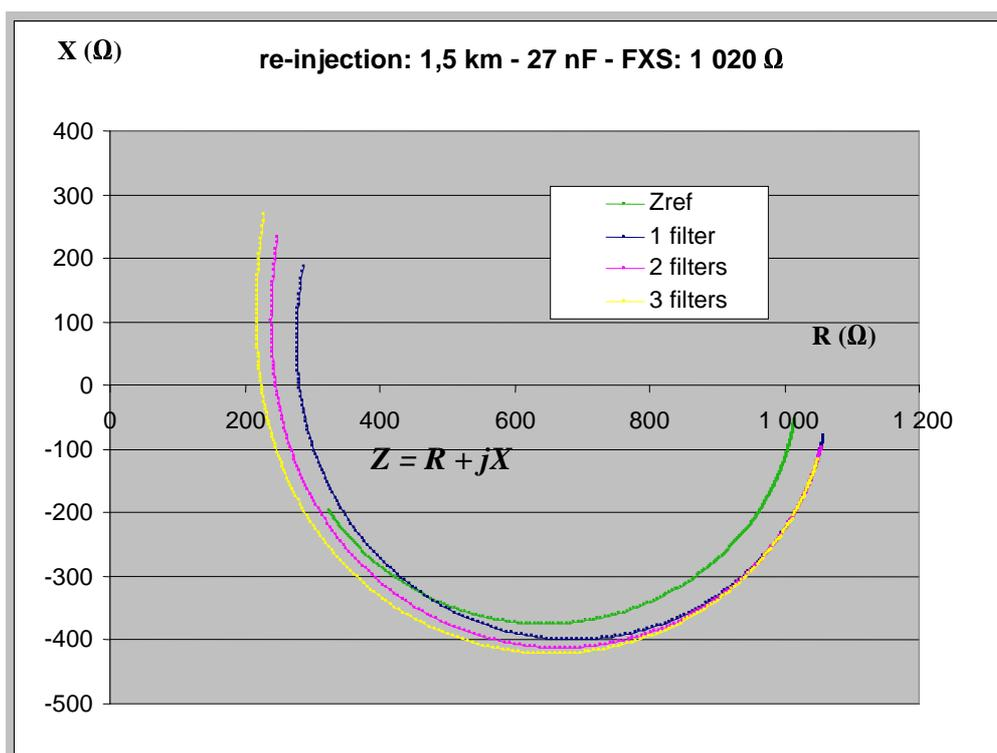
Figure B.13: Impedances presented at the TE port for FXS=1 020 Ω - 1,5 km local loop
