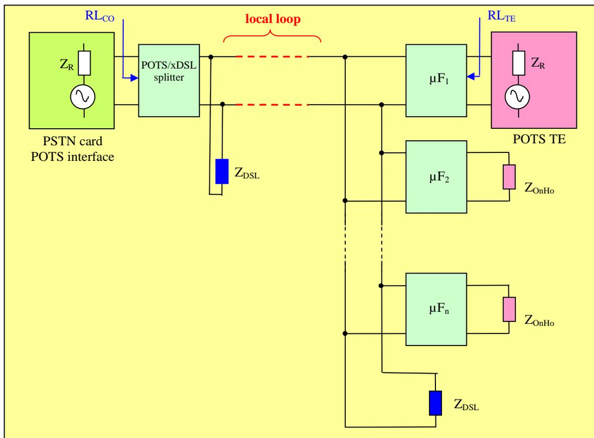
Figure 5: POTS transmission path of traditional xDSL deployment
