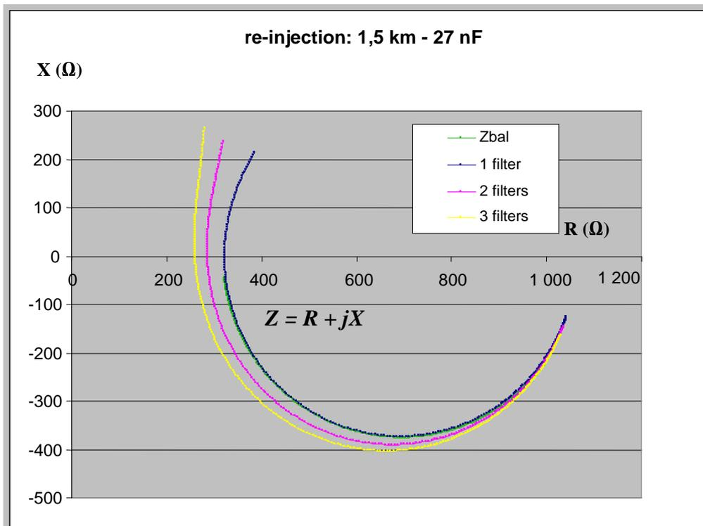
Figure B.7: Impedances presented at the FXS port, comparison with new balance impedance  $Z_{bal}$  - 1,5 km local loop
