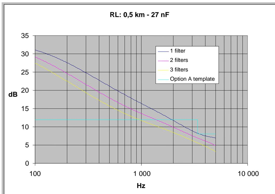
**Figure B.3: Return Loss (with respect to  $Z_R$ ) of impedances presented at the FXS port - 0,5 km local loop**
