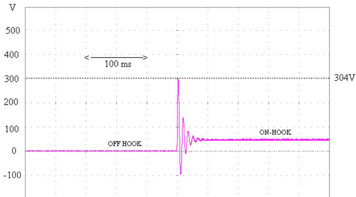
Figure 26: Off/on-Hook transients. Traditional xDSL deployment. Two microfilters.
