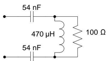
Figure A.1: Schematic diagram of the impedance  $Z_{\text{DSL}}$
