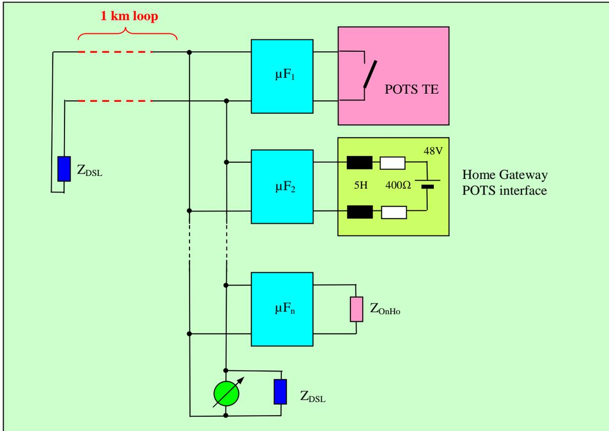
Figure 24: test of the on-hook/off-hook transients at the xDSL interface of the HG for the re-injection scenario
