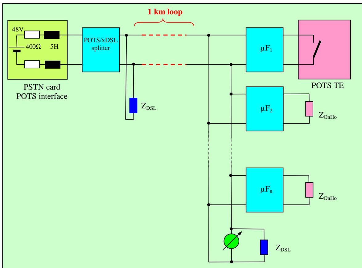
Figure 23: test of the on-hook/off-hook transients at the xDSL interface of the HG for the traditional xDSL deployment
