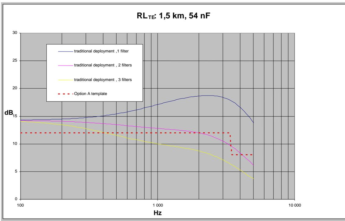
NOTE: Cable length: 1,5 km. High capacity microfilters.
