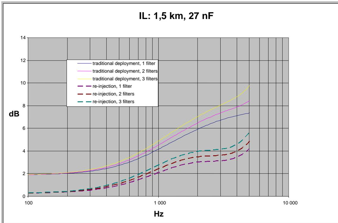
NOTE: Cable length: 1,5 km. Low capacity microfilters.
