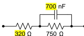
**Figure B.5: Alternative balance impedance  $Z_{bal}$  of the HG hybrid (for 2 wires/4 wires transition)**
