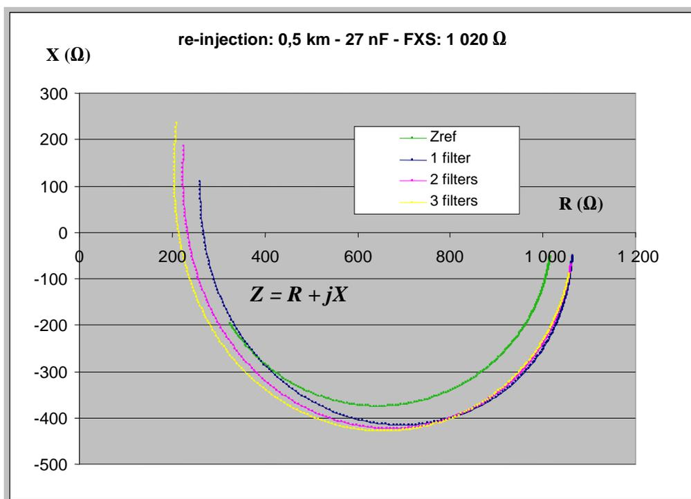
Figure B.12: Impedances presented at the TE port for  $FXS = 1\ 020\ \Omega$  - 0,5 km local loop
