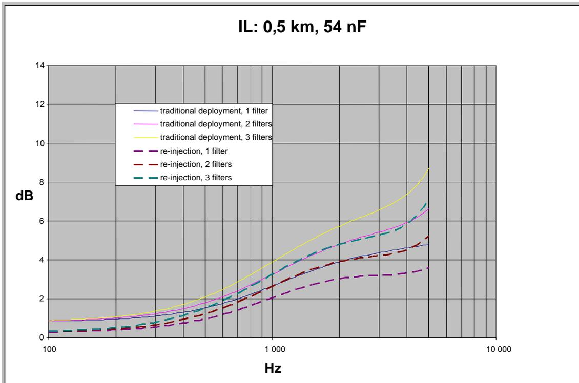
NOTE Cable length: 0,5 km. High capacity microfilters.
