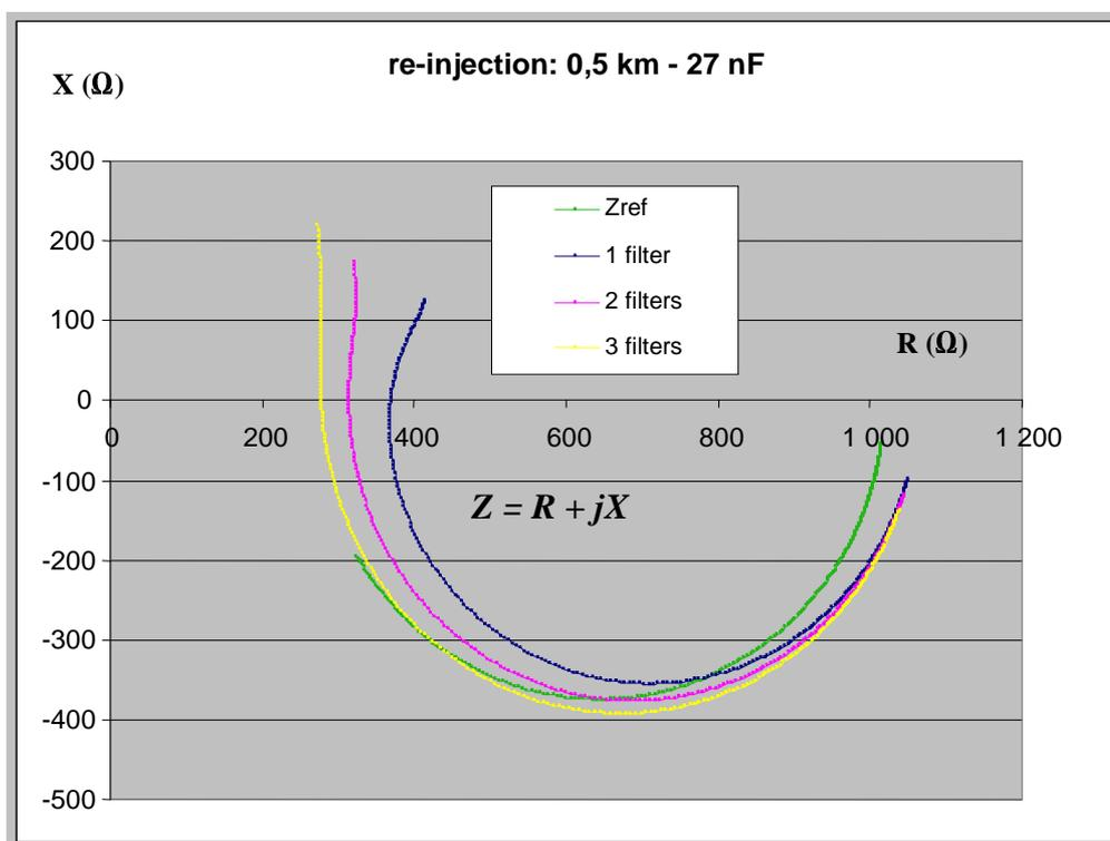
Figure B.10: Impedances presented at the TE port for FXS= $Z_R$  - 0,5 km local loop
