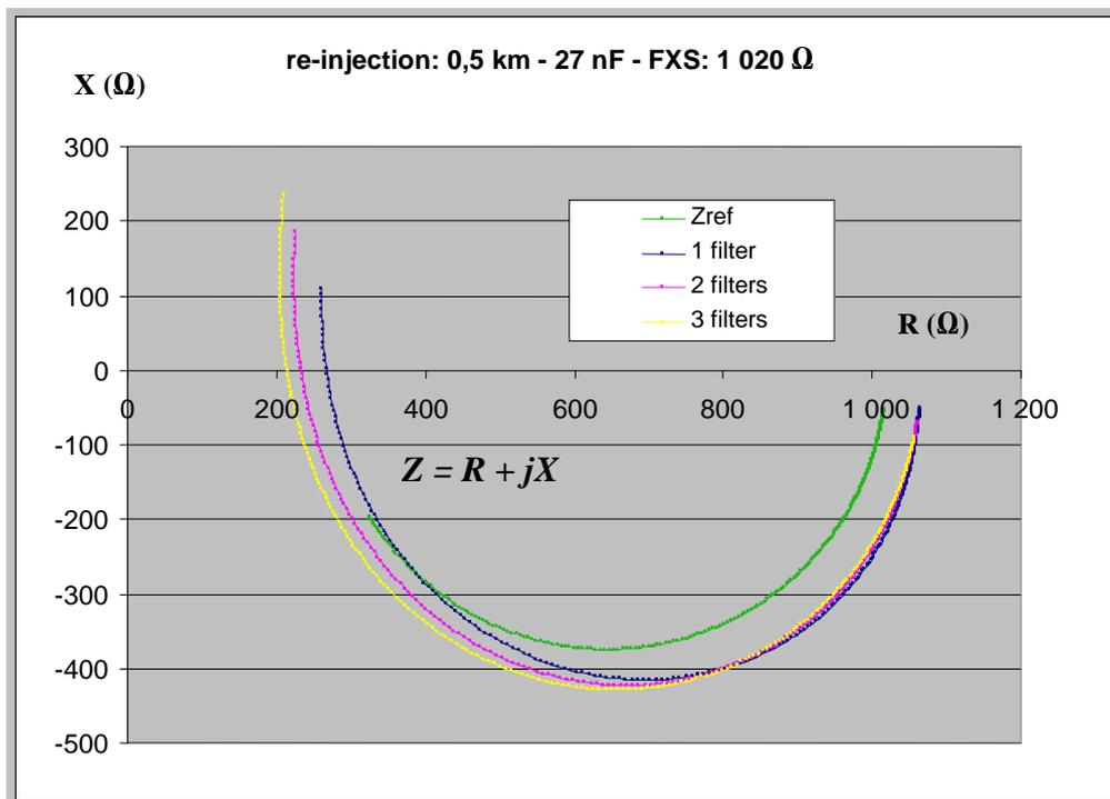
Figure B.12: Impedances presented at the TE port for  $FXS = 1020 \Omega$  - 0,5 km local loop
