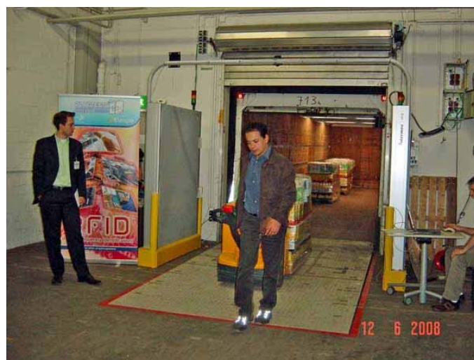
Figure E.5: Pallet tests at a dock door
