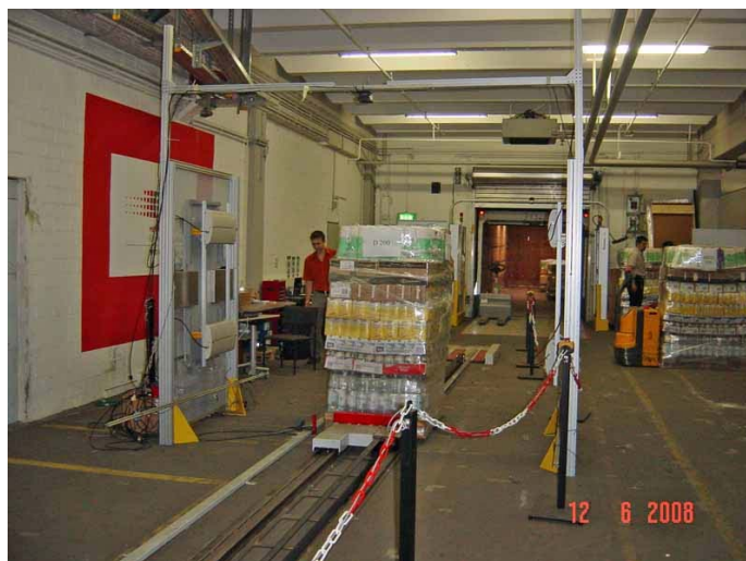
Figure E.6: Pallet tests using rail track system
