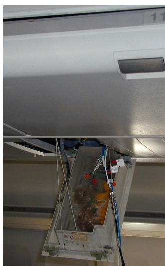
Antenna location in airplane in the same place the access point will be installed
