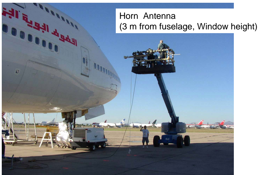
Figure C.4: Picture of measurements "Through Airplane"
