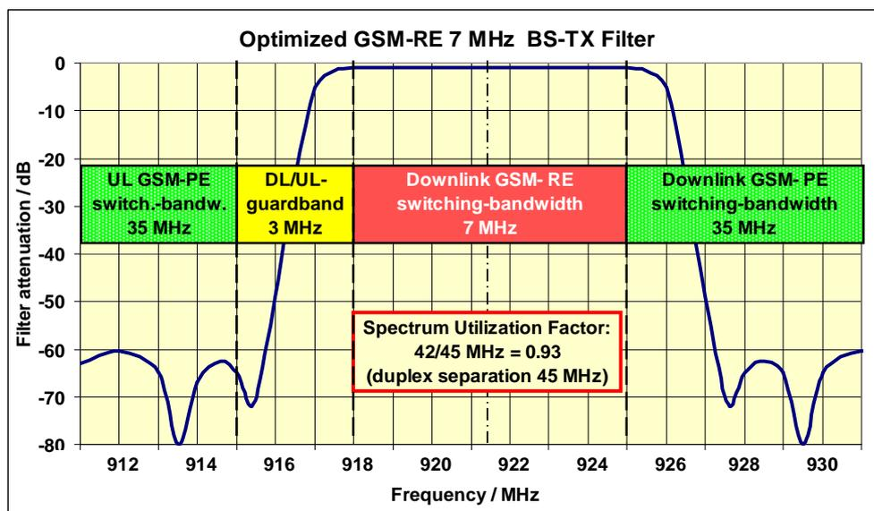
**Figure C.1: Shape of a typical optimized GSM-R TX filter with 60 dB out band suppression**
