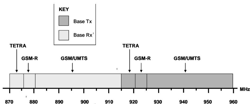
An important performance aspect of Mobile Stations (MSs) operating in any duplex band is their receiver selectivity. The chart below explains this in more detail.
