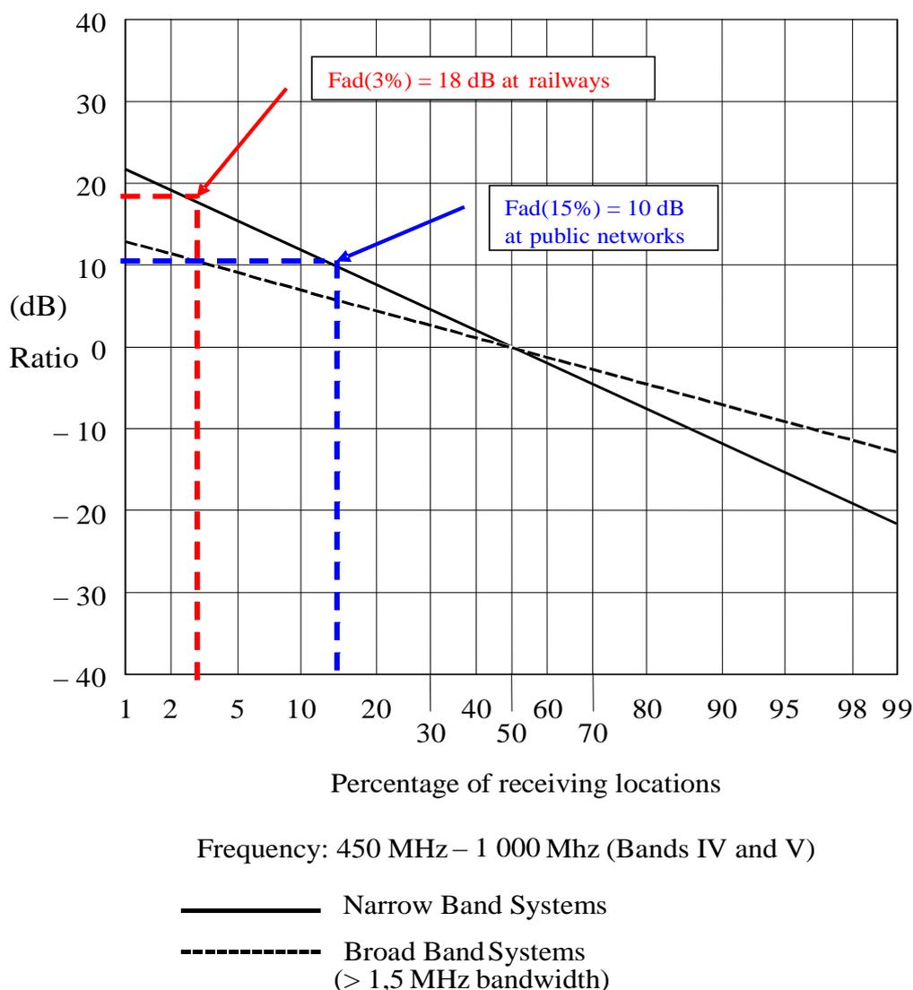
**Figure B.7: Ratio (dB) of the field strength for a given percentage of the receiving locations to the field strength for 50 % of the receiving locations**
