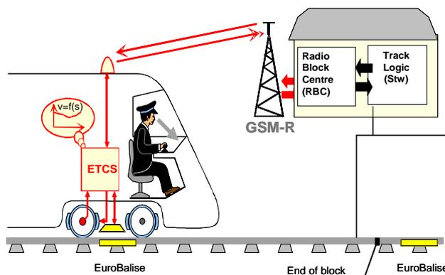
**Figure B.1: Diagram of ETCS level 2**
