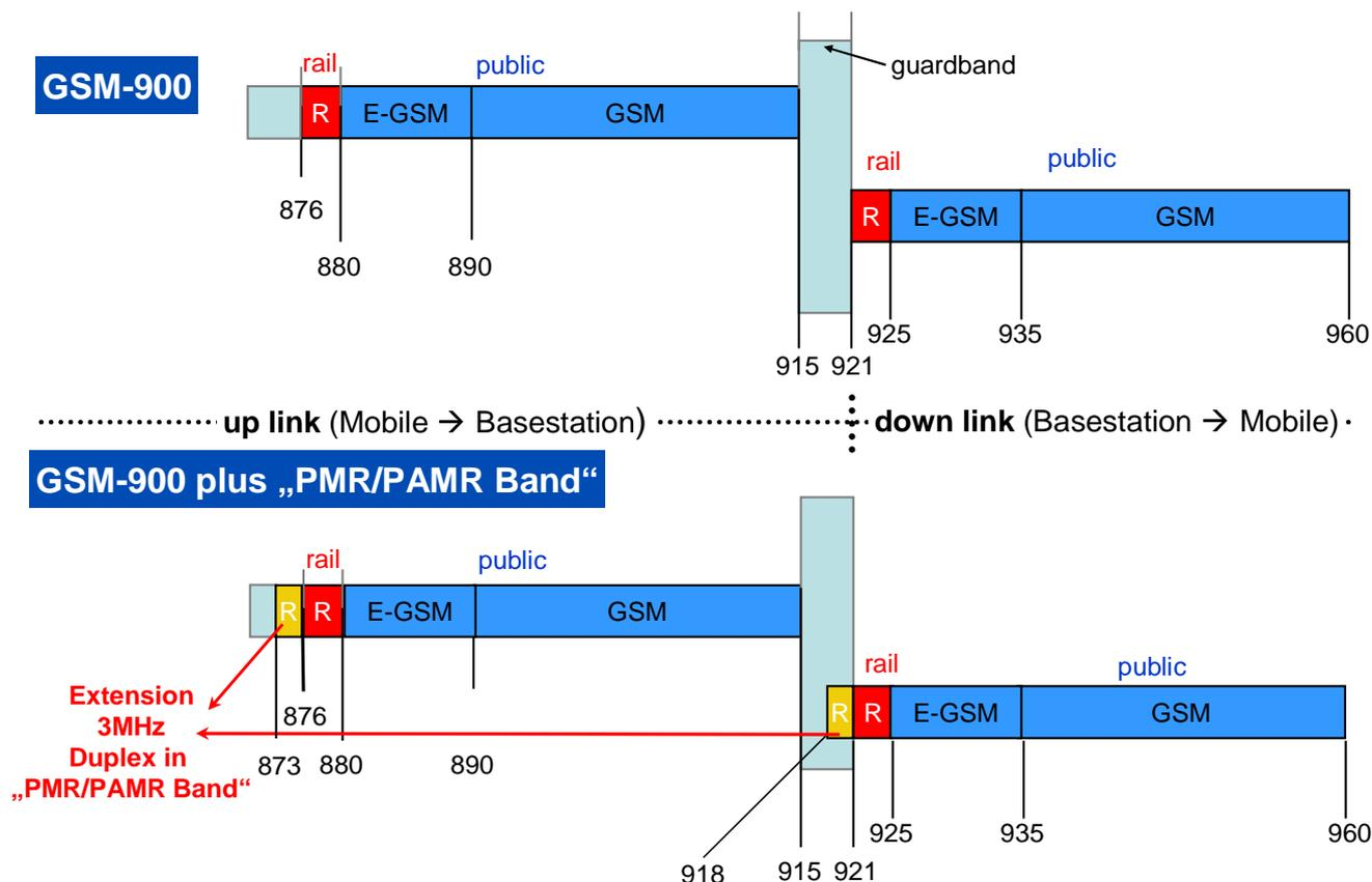
**Figure 1: Amendment for additional GSM-R frequencies**
