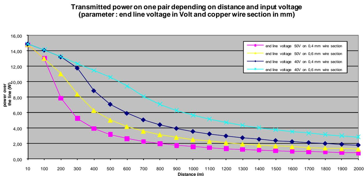
**Figure A.1: Back feeding power function of distance at 60 V injection**
