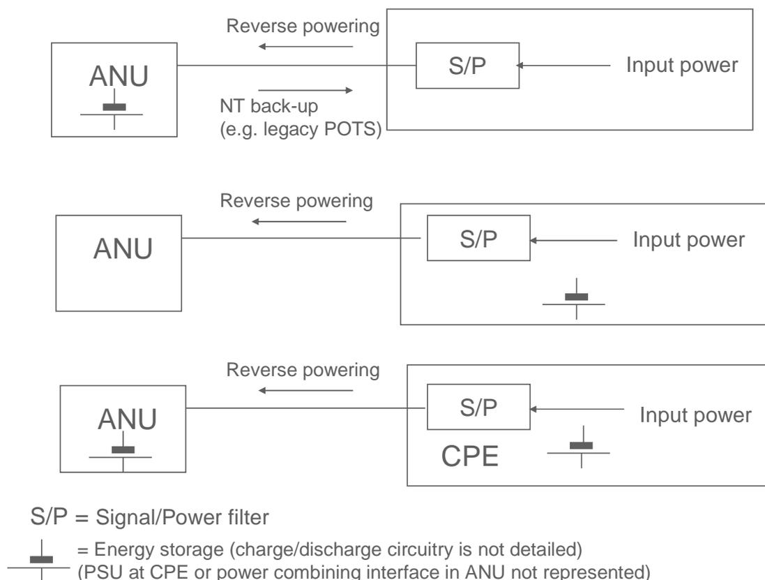
**Figure 2: Backup options (example of implementation in the case of an ONU)**
