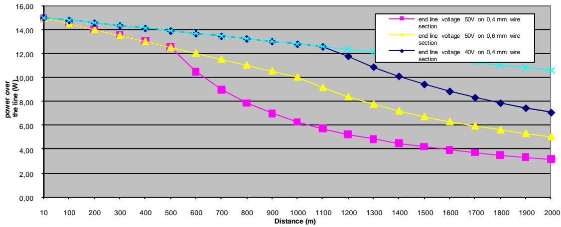
**Figure A.2: Back feeding power function of distance at 120 V injection (+60 V -60 V)**
