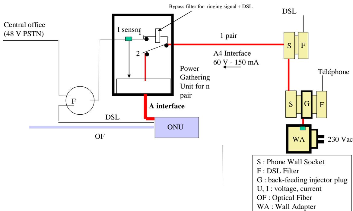
**Figure B.1: Principle to avoid central office PSTN DC voltage collision with back feeding DC**
