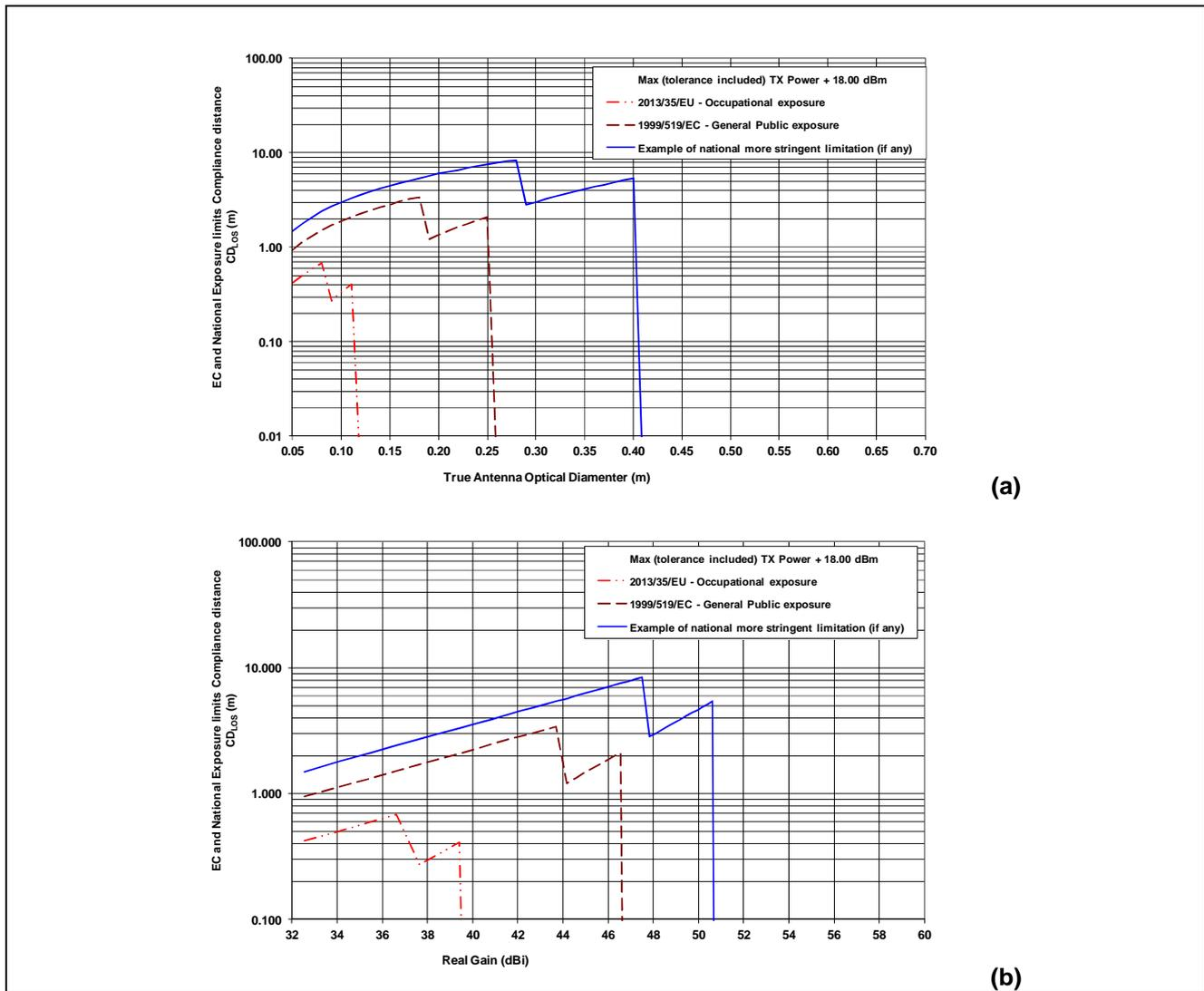
Figure 8.9: CD<sub>los</sub> versus inner antenna diameter (a), or real gain (b) for 81 GHz equipment at maximum nominal power; evaluation with various regulatory limits
