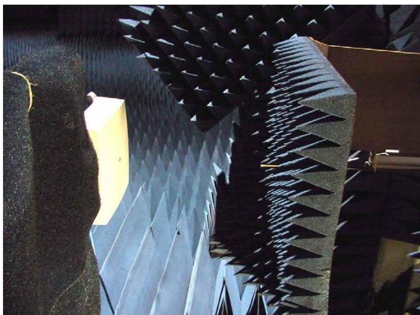
**Figure B.5: Antenna to the left and the WR28 rectangular waveguide probe to the right**
