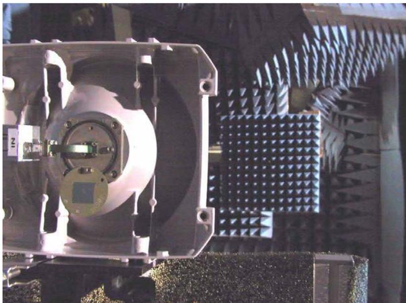
**Figure B.4: Rear side of the 38 GHz 24 cm reflector antenna with a rectangular waveguide interface**
