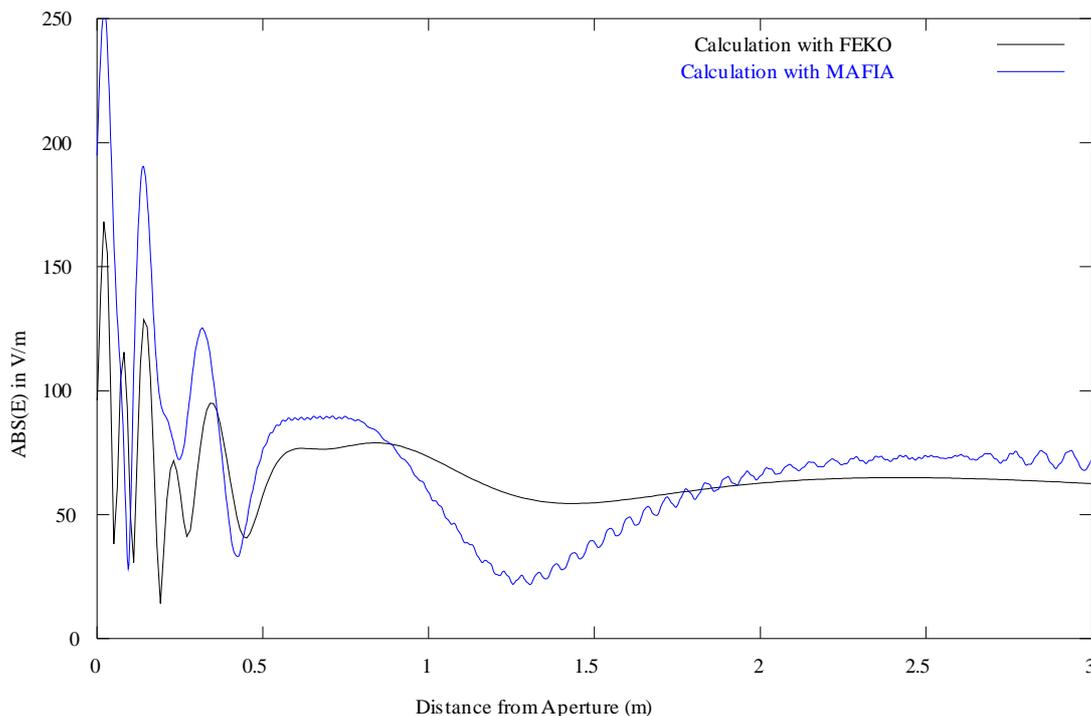
**Figure B.15: Electric field vs probe simulation with FEKO™ and MAFIA™ comparison**
