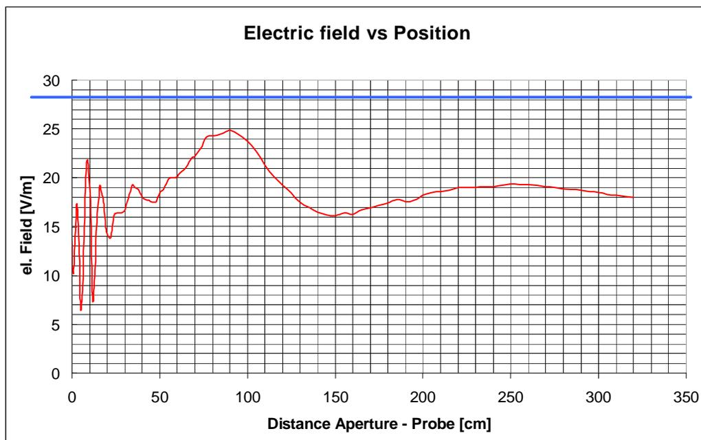
**Figure B.12: Electric field vs probe position (without absorber)**
