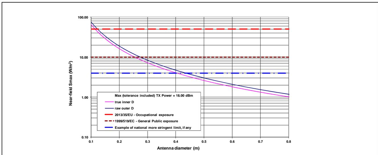
Figure 8.10: Near field Smax (peak value) versus antenna diameter for 81 GHz equipment at maximum nominal power; evaluation with various regulatory limits
