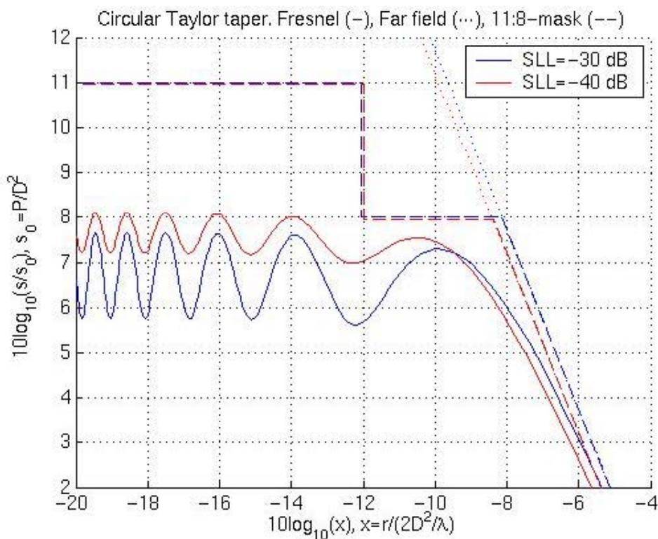
NOTE: The mask is valid also for the Taylor taper near fields depicted here. Note that for lower sidelobe levels the aperture efficiency and the effective area of the antenna decrease which yields an increase in the near field power density, especially close to the antenna.
