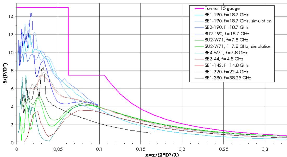
**Figure B.27: Power density measurement and simulation results with format F=15 envelope template using outer diameter**
