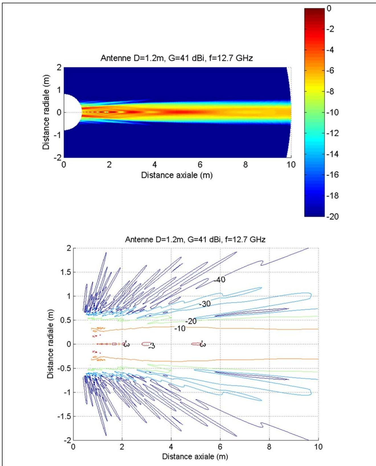
Figure B.32: Cross section of the power density distribution
