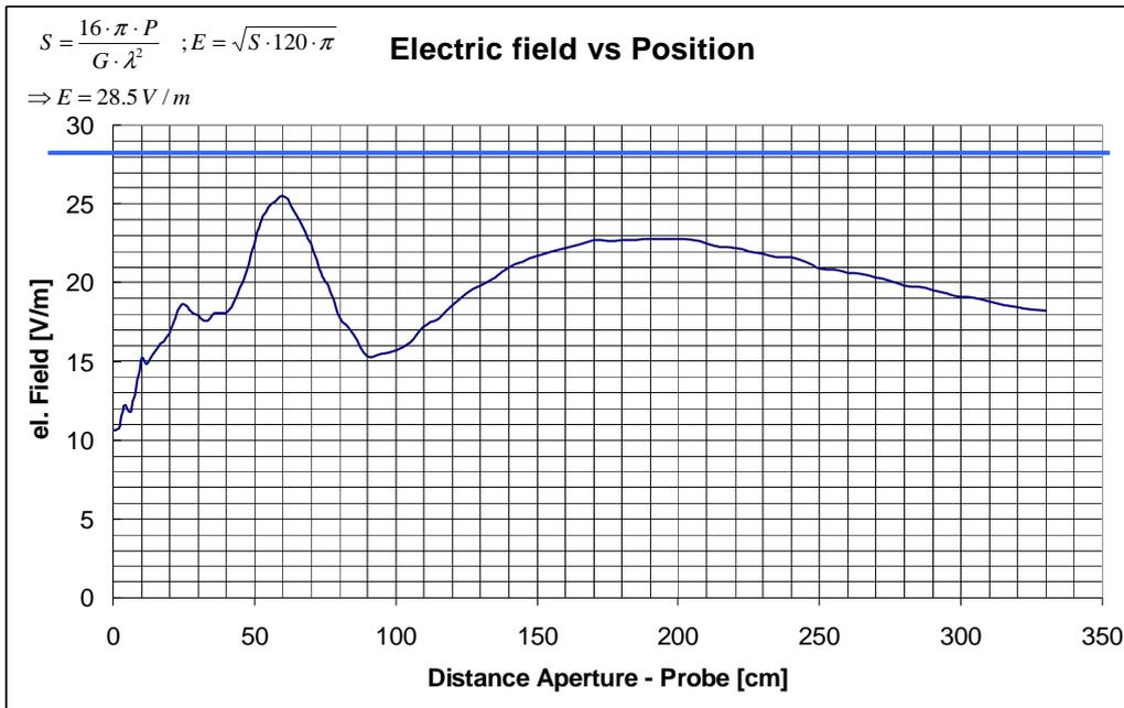
**Figure B.11: Electric field vs probe position (with absorber)**
