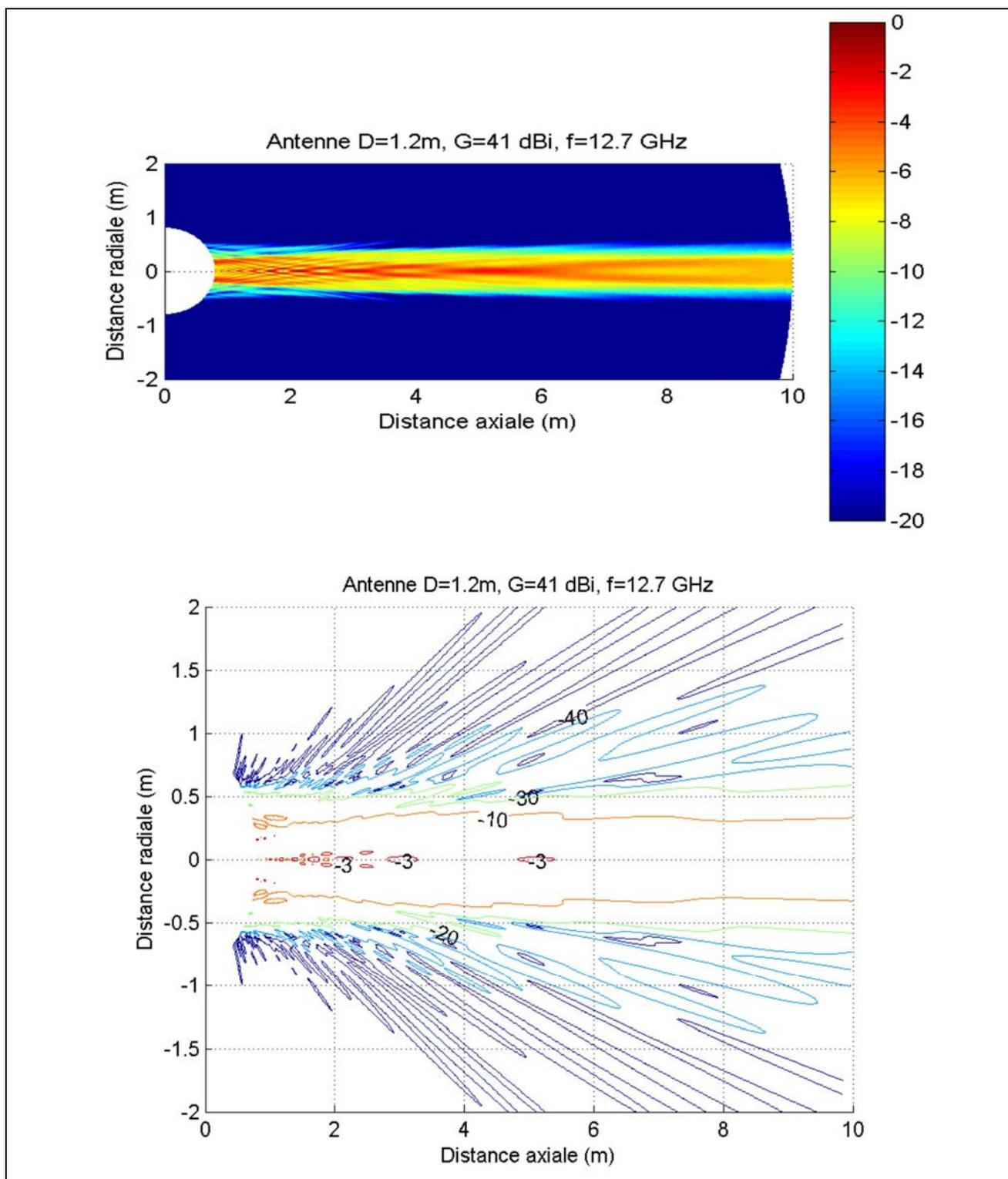
Figure B.31: Cross section of the power density distribution
