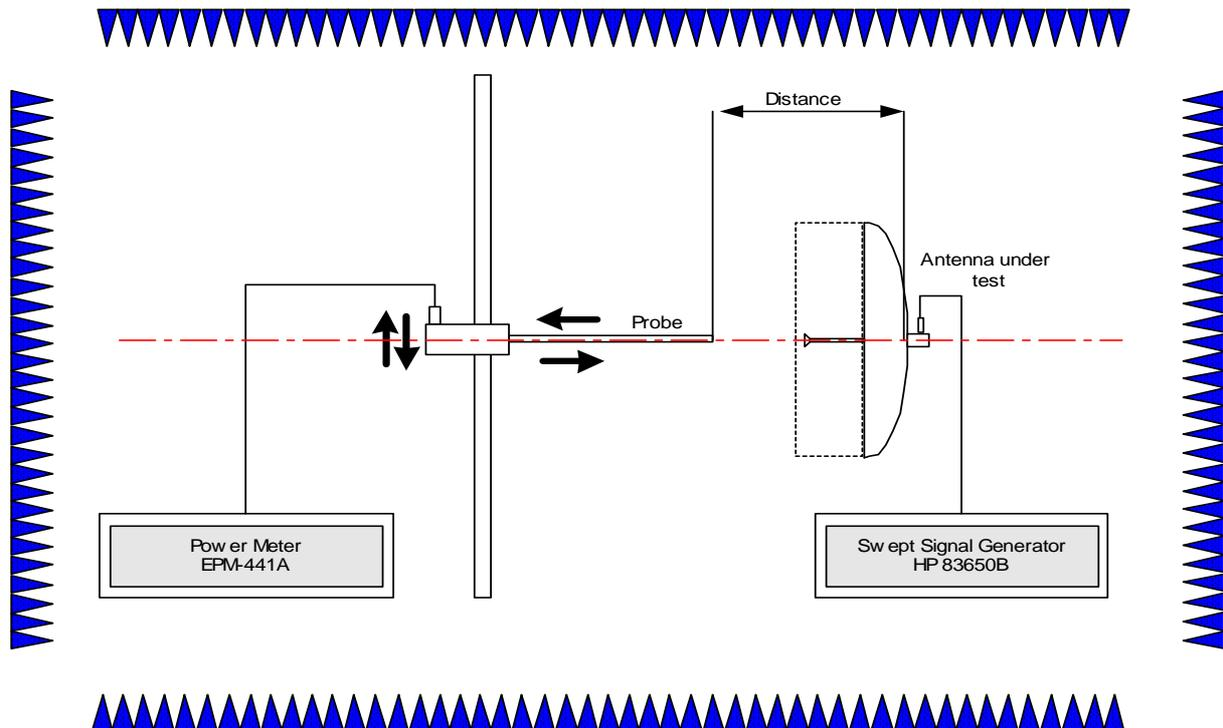
Figure B.22: Measurement setup for power density measurement
