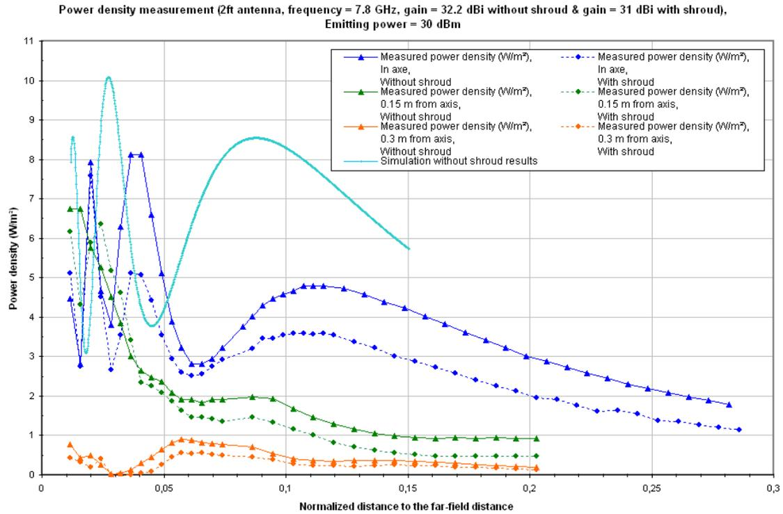
Figure B.23: Measurement results for antenna model SU2-W71A
