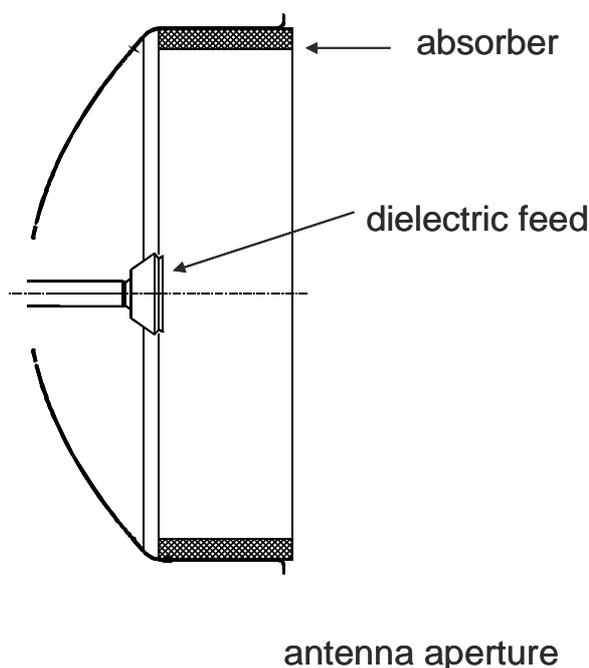
**Figure B.8: Antenna schematic picture**
