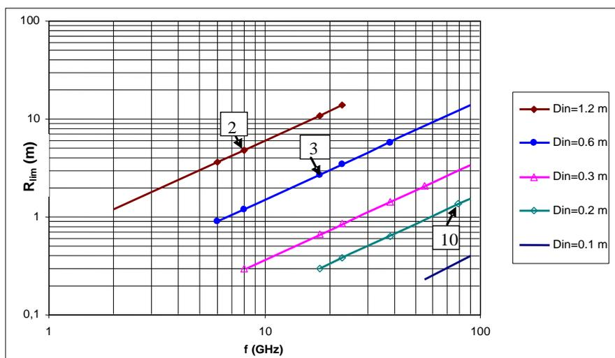
Figure 8.4: Limit distance versus frequency for 0,1 m to 1,2 m antennas
