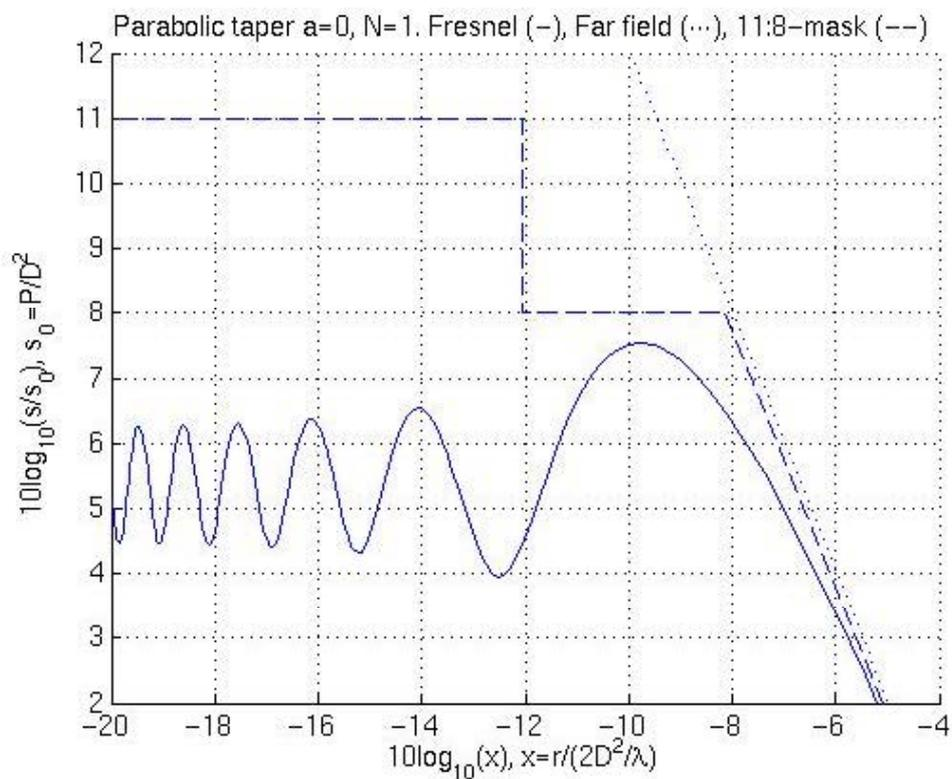
NOTE: The parabolic taper near field also complies with the proposed mask. However, it is not a realistic case, especially due to low power density levels close to the antenna  $x < 1/16$  (-12 on the scale).
