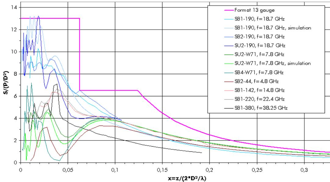
**Figure B.26: Power density measurement and simulation results with format F=13 envelope template using inner diameter (aperture)**
