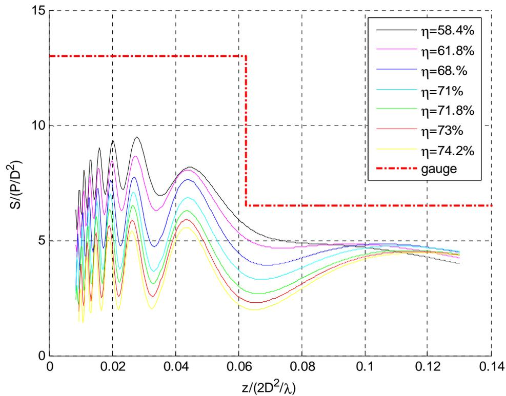
**Figure B.36: Normalized power density vs. efficiency (focal distances) and format F=13 envelope template @ 8 GHz**
