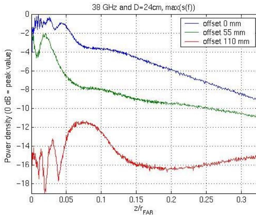
NOTE: At the rim (red curve), power densities 10 dB lower relative to the overall peak are found. The curves depict the maximum with respect to frequency as a function of distance.
