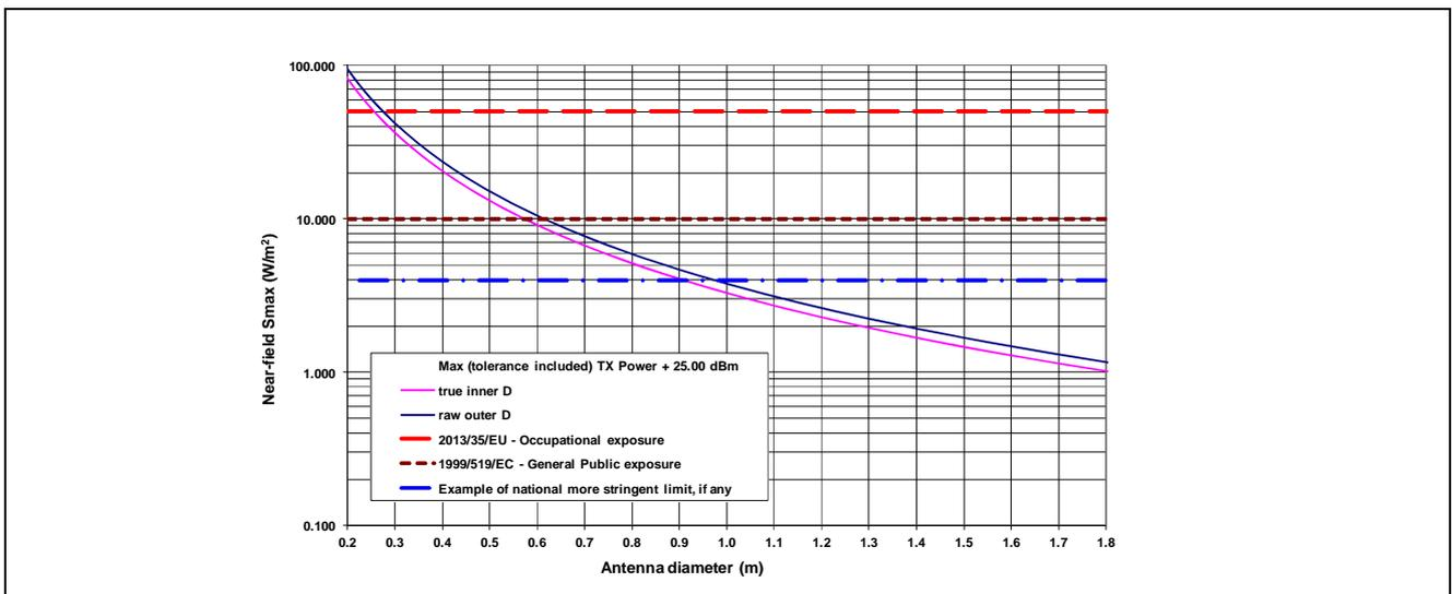
Figure 8.8: Near field  $S_{max}$  (peak value) versus antenna diameter for 23 GHz equipment at maximum nominal power; evaluation with various regulatory limits
