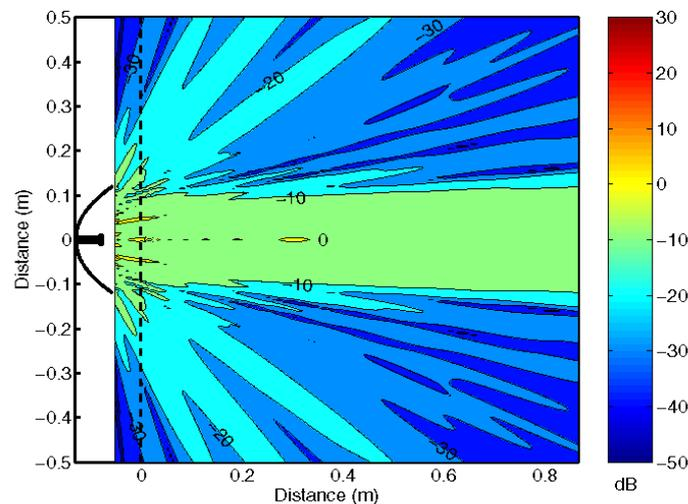
NOTE: A cross section of the power density distribution in a volume around the 38 GHz 24 cm antenna (to the left). The 0 dB level is the overall peak level. The power densities outside a circular tube along, and centered at, the main axis, are below -10 dB.
