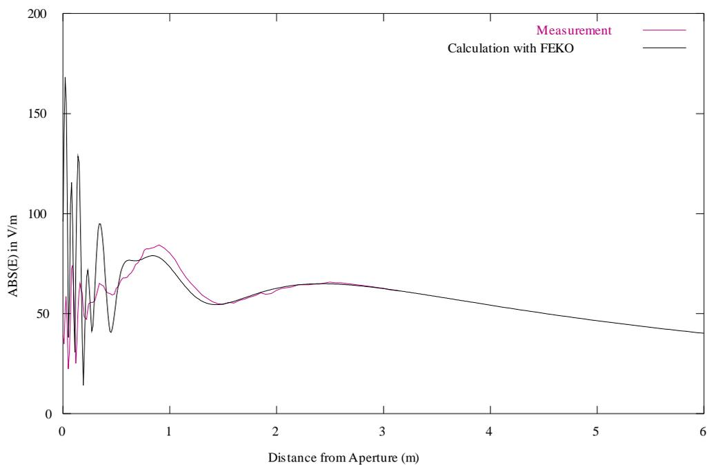
**Figure B.13: Electric field vs probe Measured and simulated with FEKO™**
