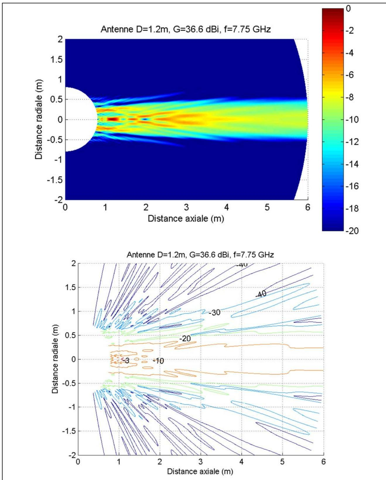
Figure B.29: Cross section of the power density distribution
