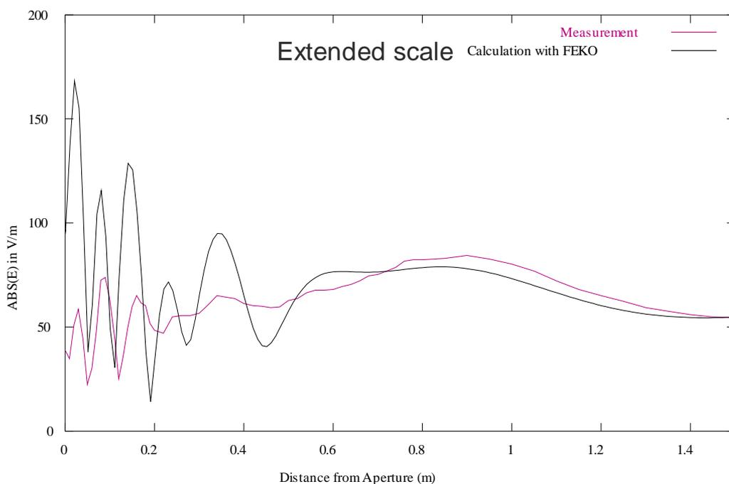
**Figure B.14: Electric field vs probe Measured and simulated with FEKO™**
