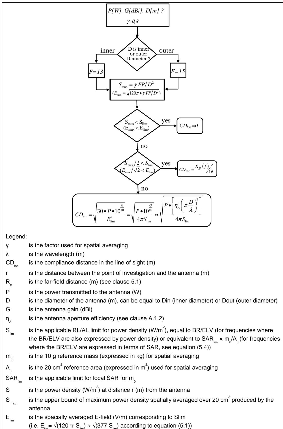
**Figure 8.2: Simplified method for assessment of the compliance distance in the line of sight of parabolic antennas above 1,3 GHz**
