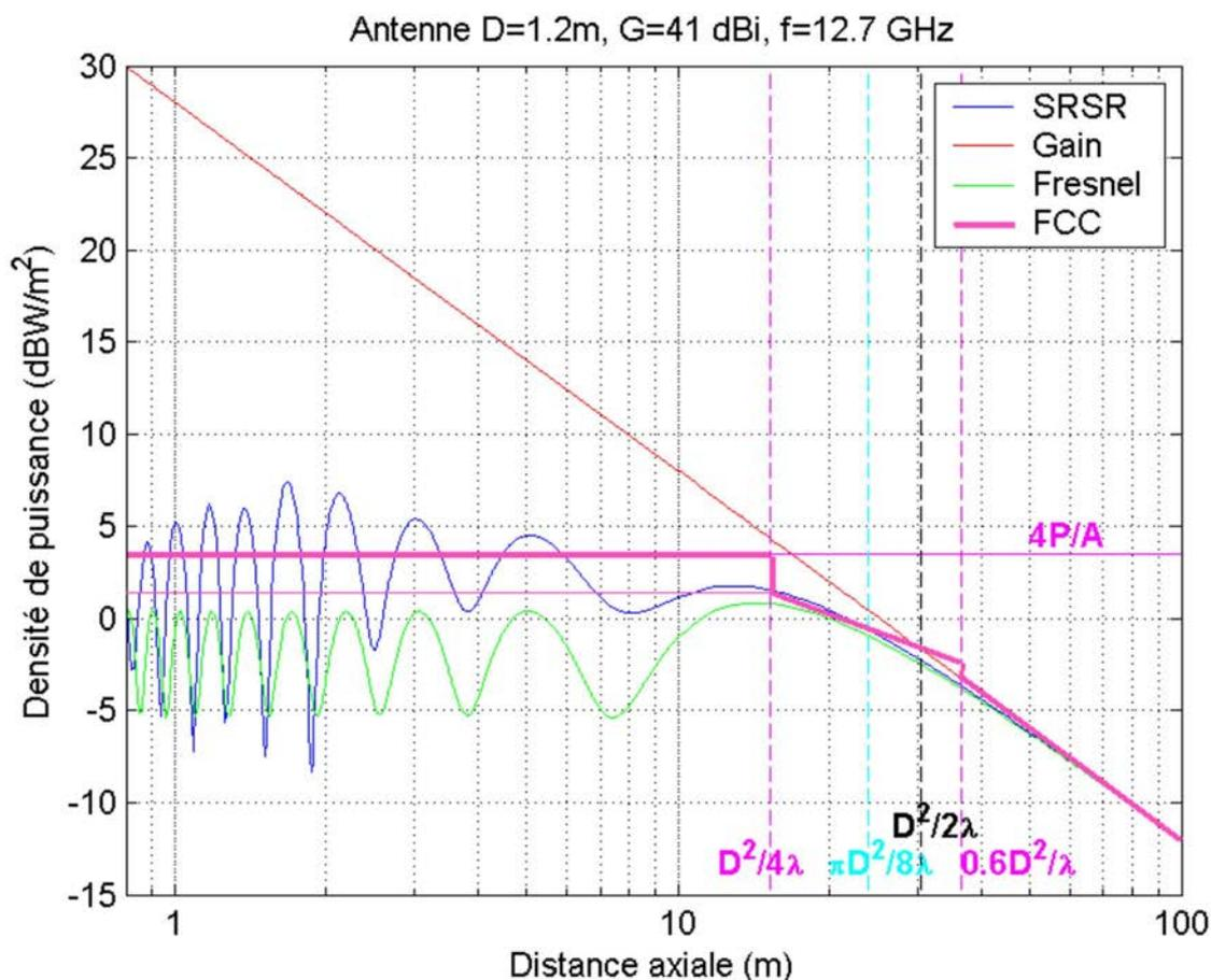
**Figure B.33: Power density measurement and simulation results with FCC envelope template**
