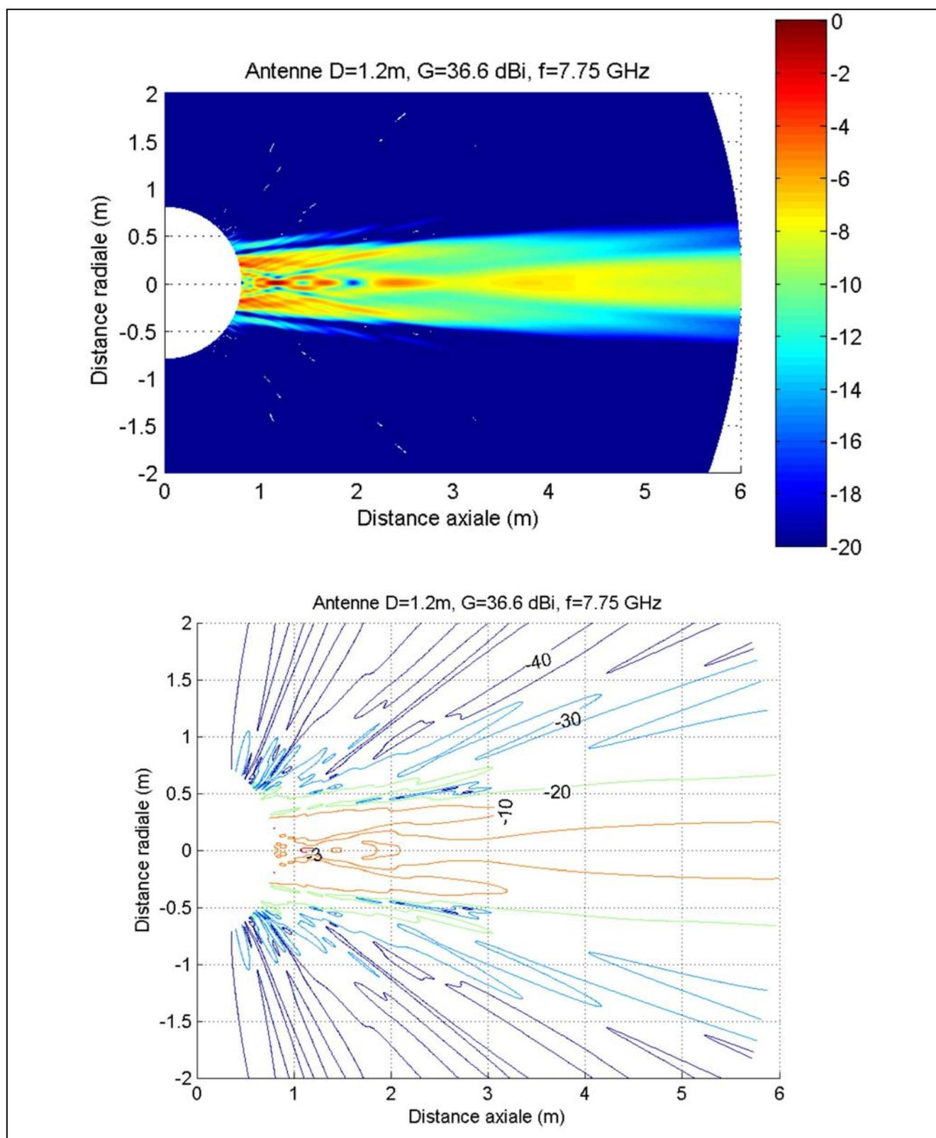
Figure B.28: Cross section of the power density distribution
