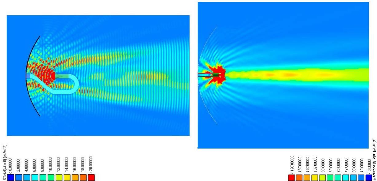
Figure B.21: Simulation results of power density on the main axis (radial pattern)
