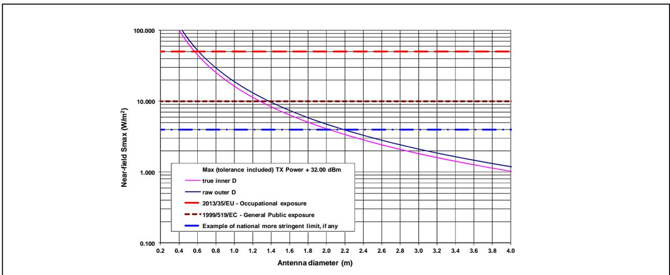
**Figure 8.6: Near field Smax (peak value) versus antenna diameter for 8 GHz equipment at maximum nominal power; evaluation with various regulatory limits**
