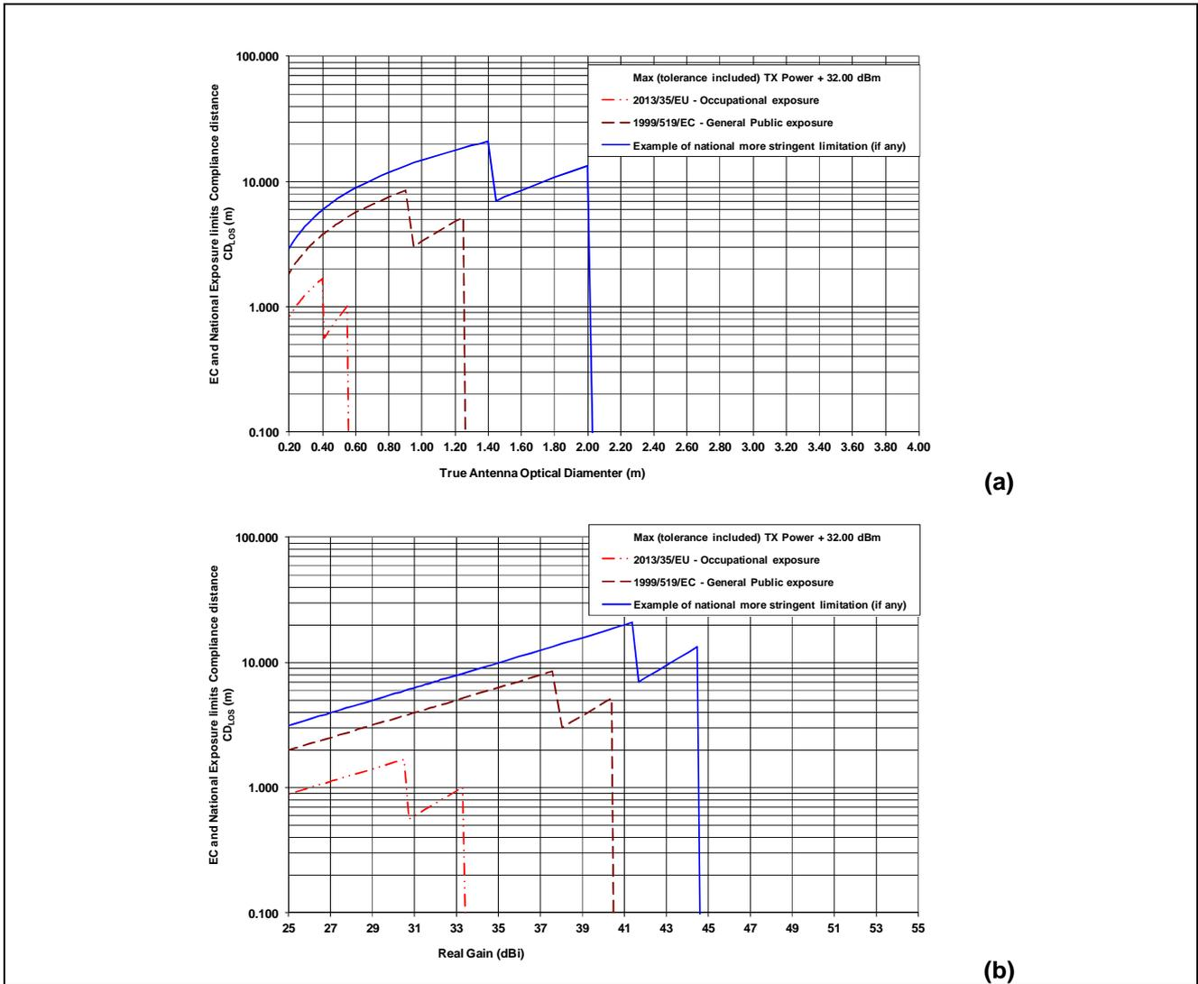
**Figure 8.5: CDlos versus inner antenna diameter (a), or real gain (b) for 8 GHz equipment at maximum nominal power**
