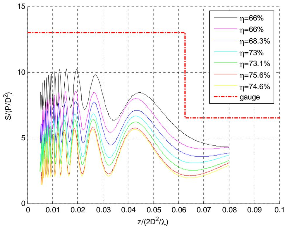
**Figure B.37: Normalized power density vs. efficiency (focal distances) and format F=13 envelope template @ 13 GHz**
