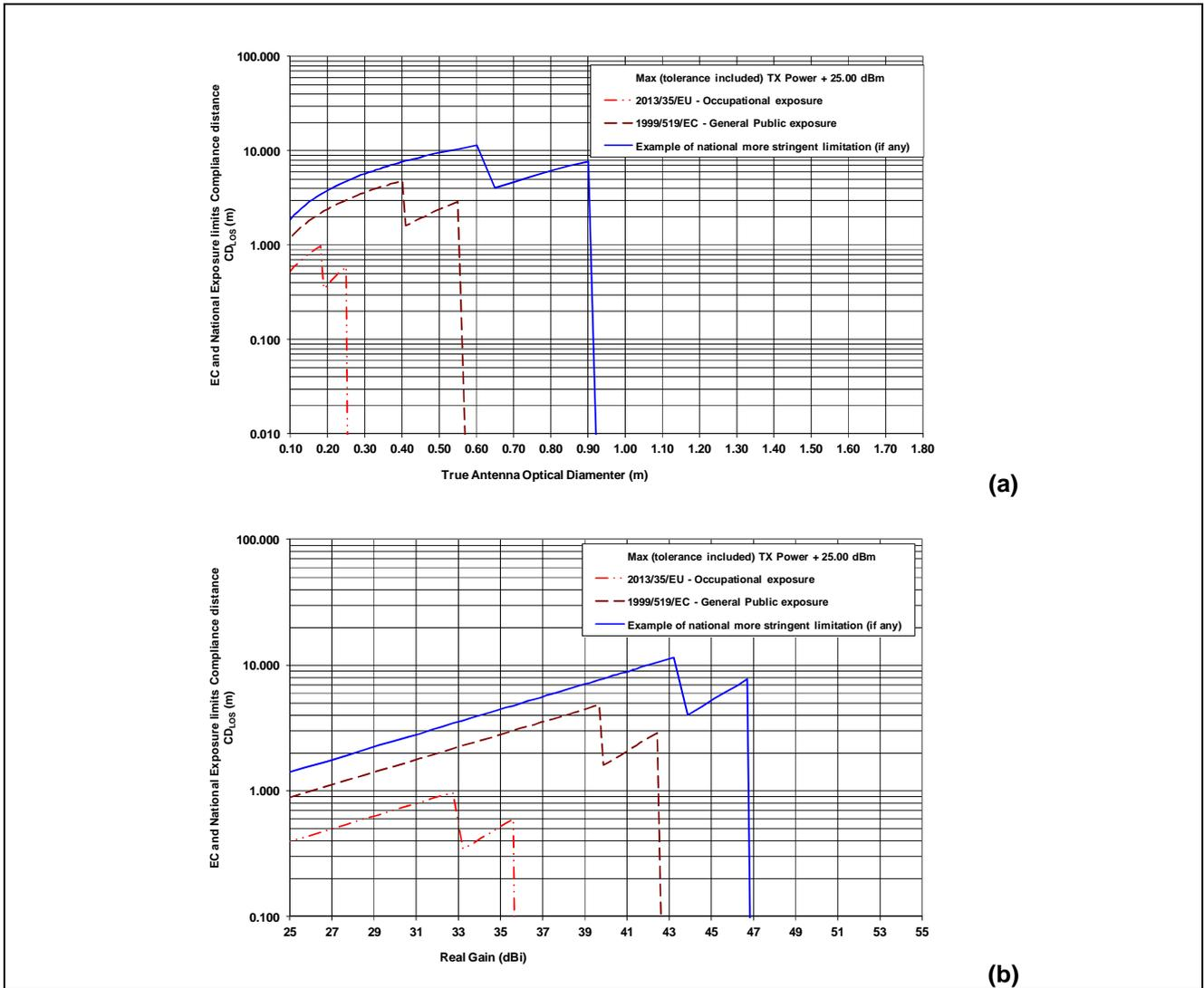
Figure 8.7:  $CD_{los}$  versus inner antenna diameter (a), or real gain (b) for 23 GHz equipment at maximum nominal power; evaluation with various regulatory limits
