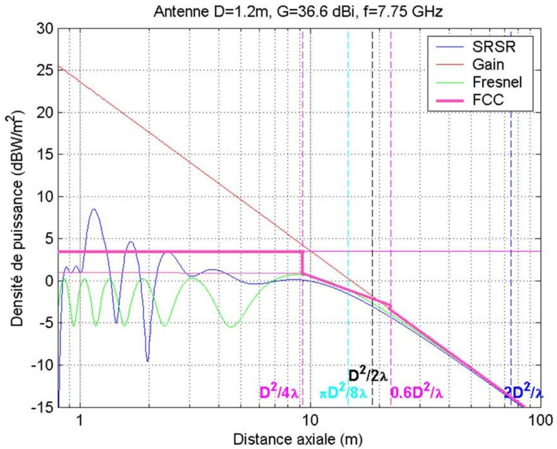
Figure B.30: Power density measurement and simulation results with FCC envelope template
