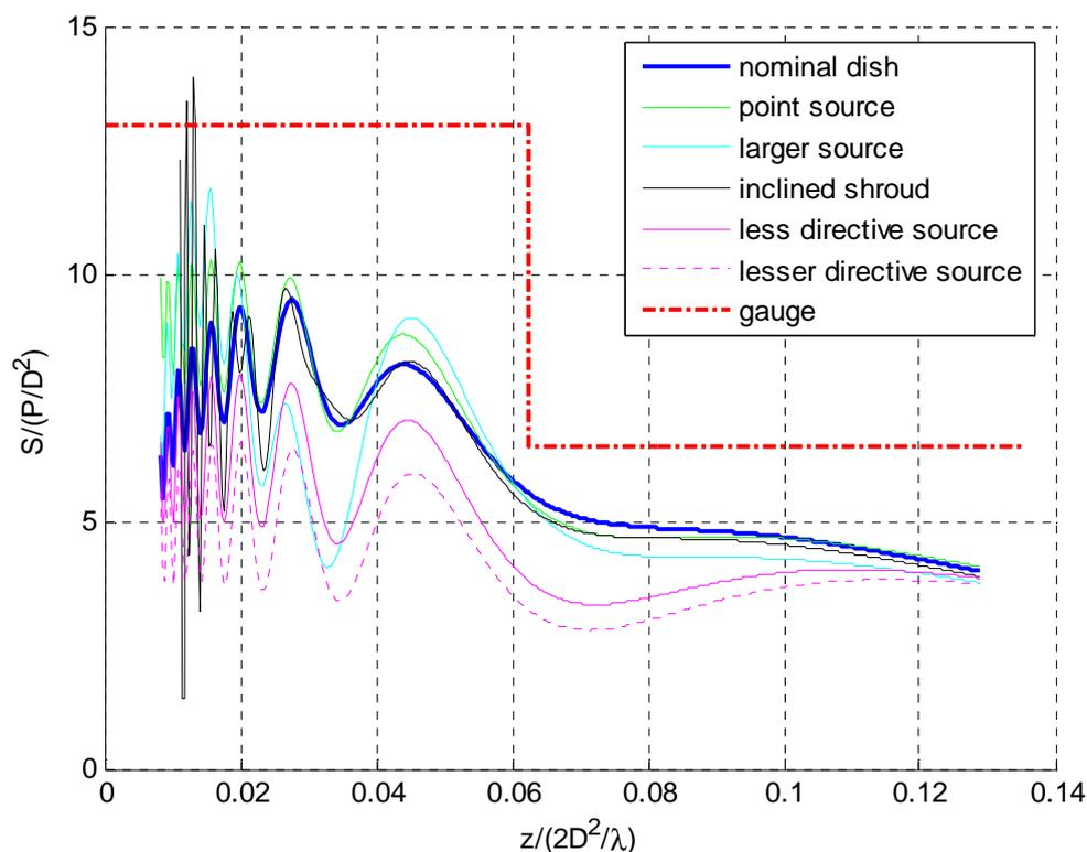
**Figure B.35: Comparisons of normalized power density vs. format F=13 envelope template**
