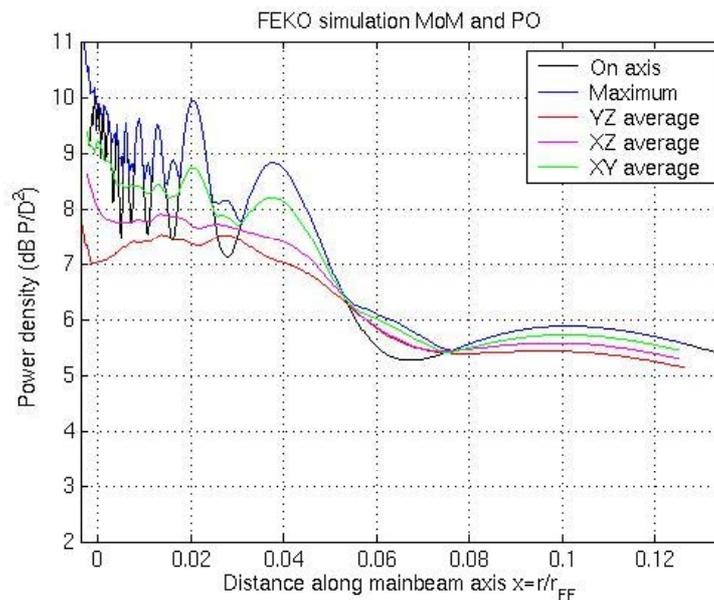
NOTE: The FEKO™ simulation reveals that the highest peaks are found on the axis, and that spatial averaging in xy-planes (perpendicular to the principal axis) yields the highest values. In this case spatial averaging lowers the power density values by approximately 1 dB near the antenna.
