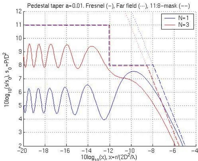
NOTE: The mask is clearly above the chosen test cases. The corresponding aperture efficiencies are 0,82 (N=1) and 0,62 (N=3), of which 0,62 or slightly lower is what is typically find in real products.
