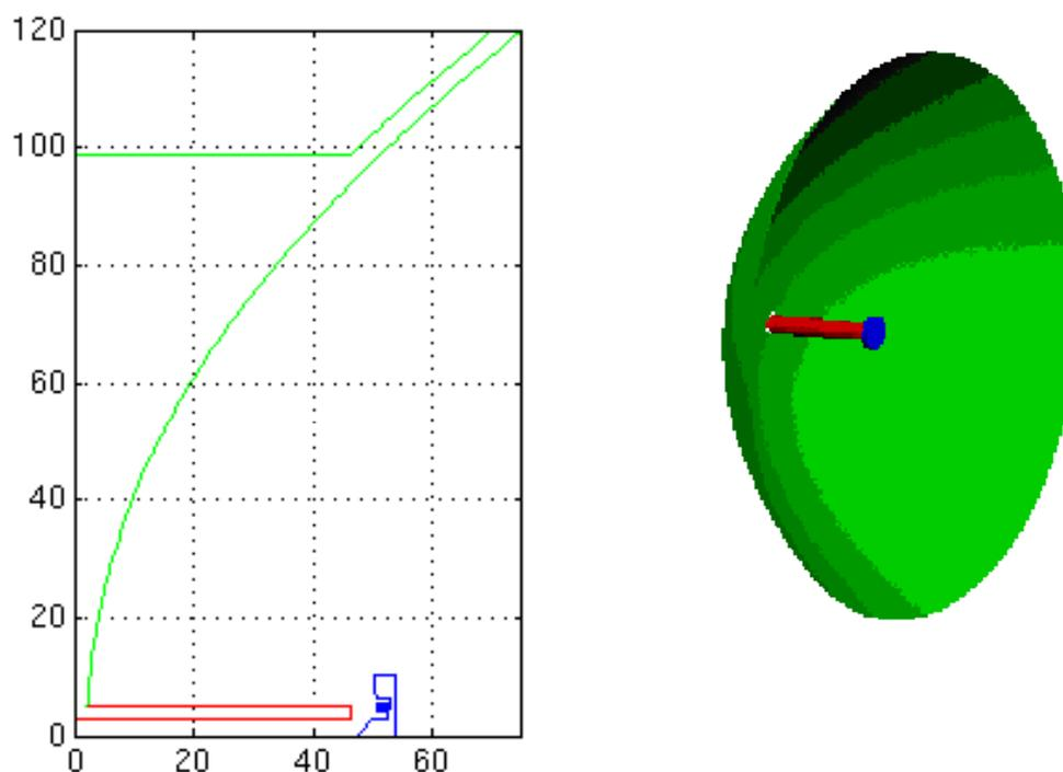
NOTE: The feeder is a circular waveguide (red) ended by a hat reflector (blue).
