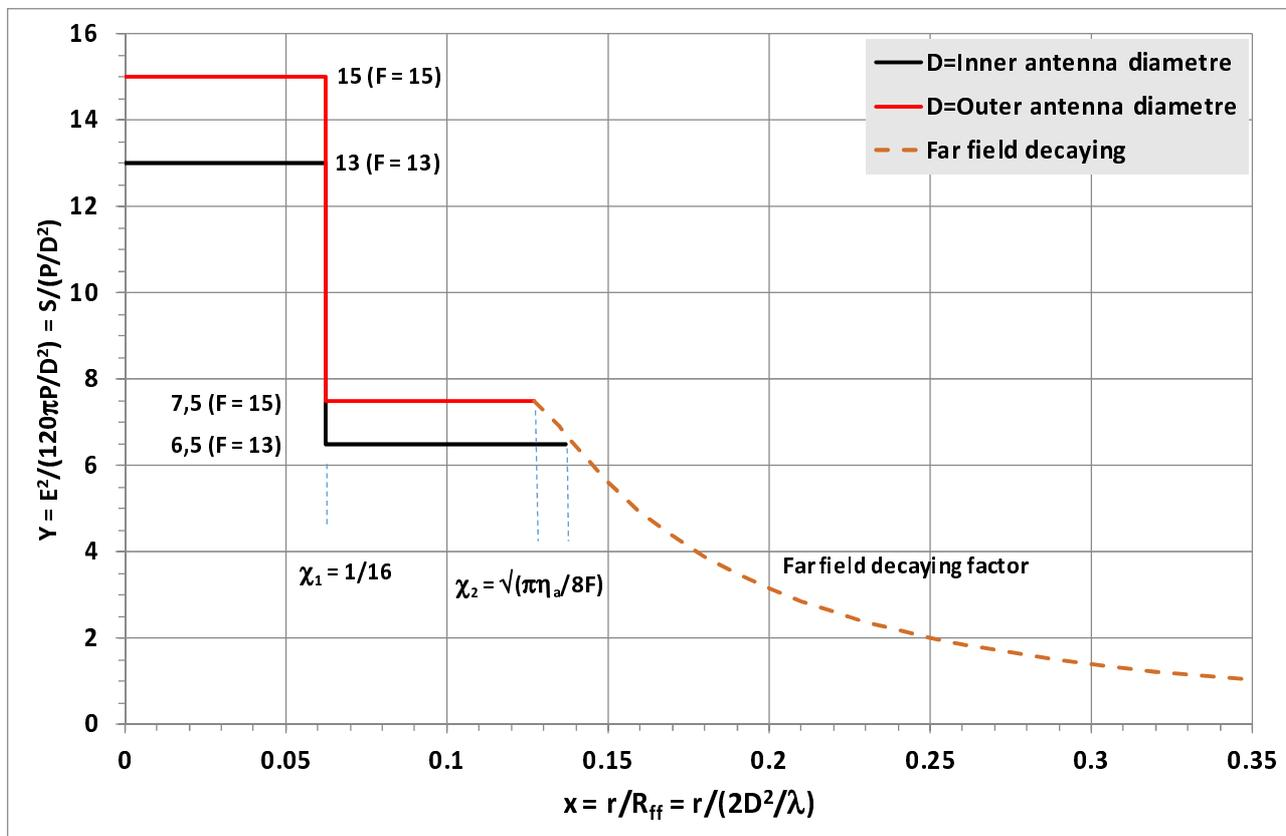
Figure 7.1: Envelope template for the power density in the main lobe of parabolic antennas
