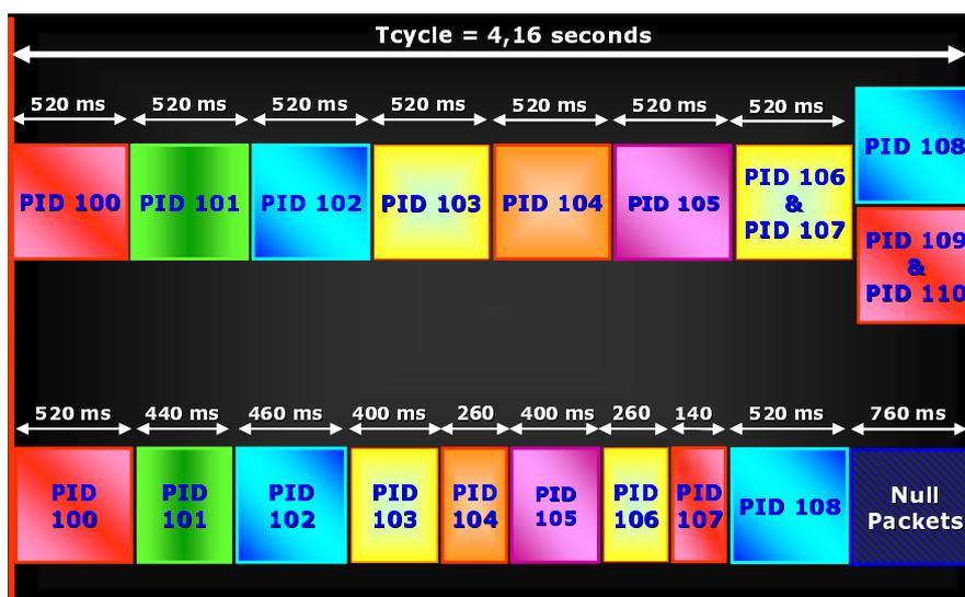
Figure 4: Burst shapes in reference Transport streams
