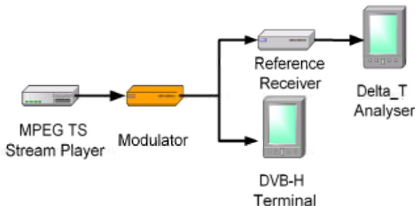
Figure 5: Basic verification of the recorded stream
