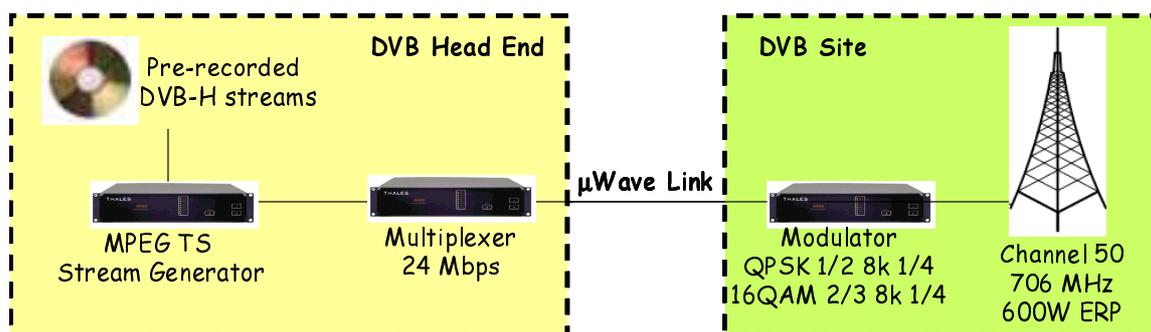
Figure 14: VTF field trials in Metz, transmission set-up
