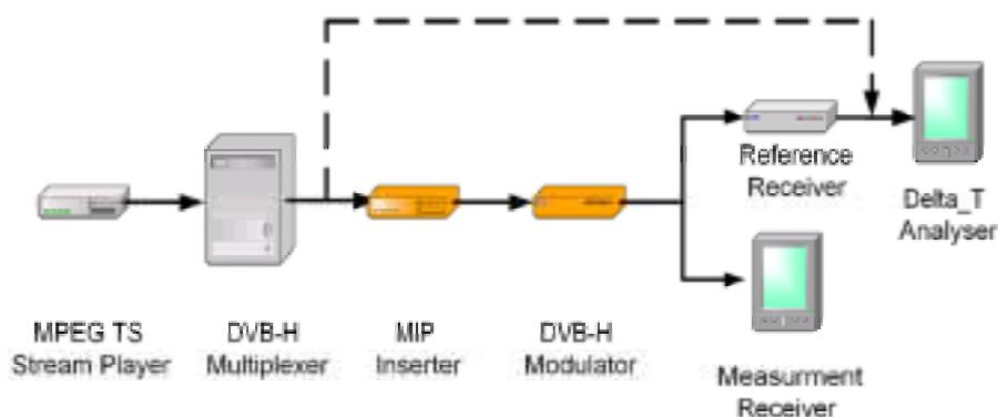
Figure 6: Recorded stream verification in the complete chain
