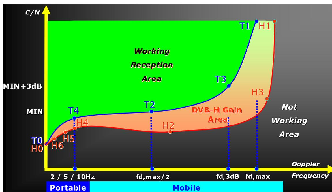
Figure A.3: C/N versus Doppler curve
