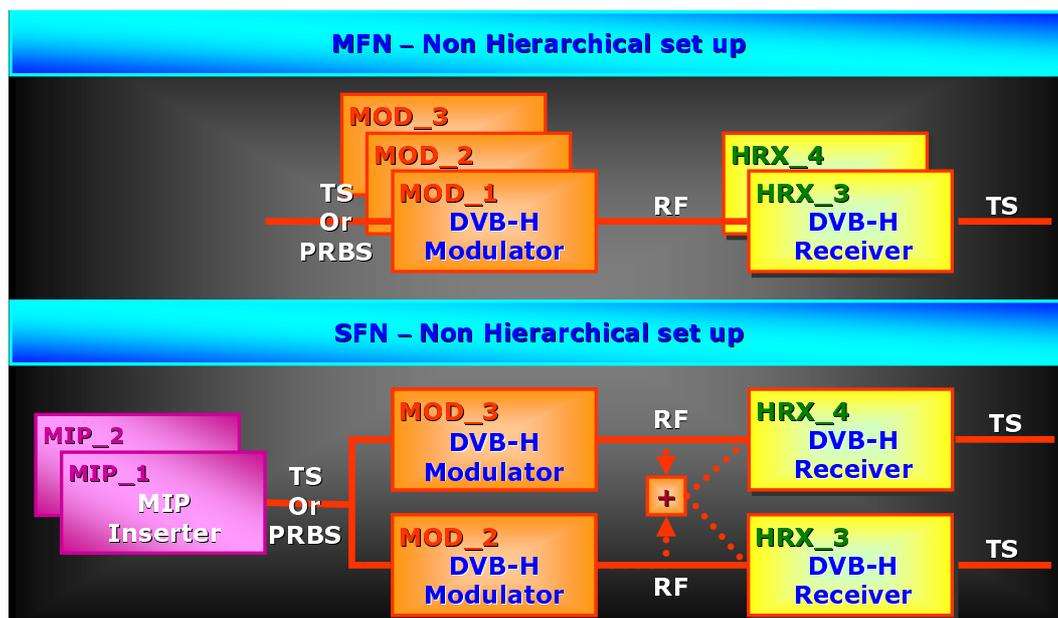
Figure 7: Interoperability at the Physical Layer level
