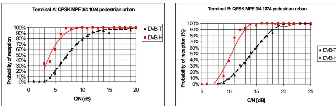
Figure 25: Pedestrian urban curves in QPSK 1/2 MPE-FEC 3/4
