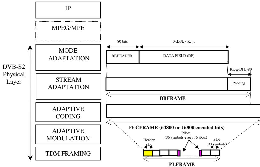
**Figure 23: Air interface architecture of the DVB-S2 using ACM**
