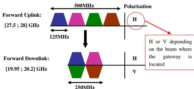
Figure D.4: Forward link frequency plan
