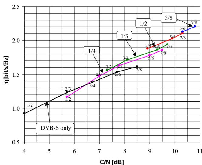
NOTE: Lines are drawn connecting points with the same configuration on the LP branch. HP configuration is also indicated.
