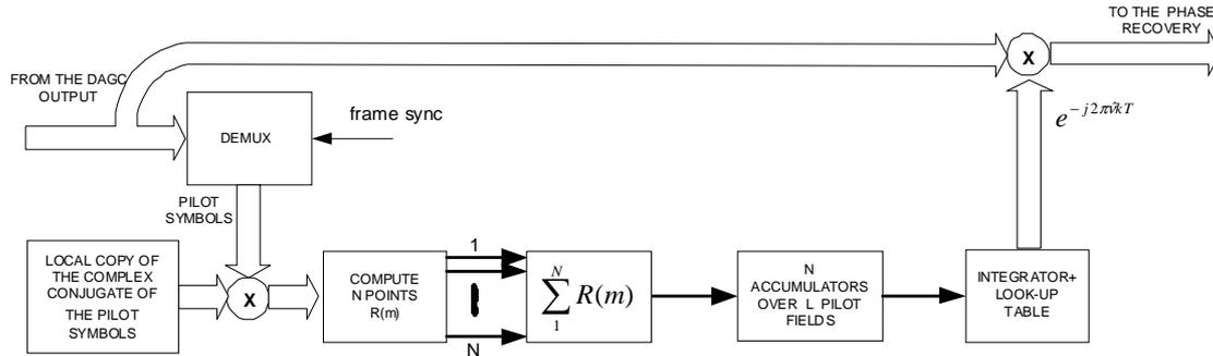
**Figure C.5: Block diagram of the fine frequency estimator**
