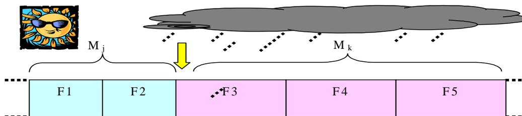
Figure 40: PLFRAMEs changing protection during a rain fading
