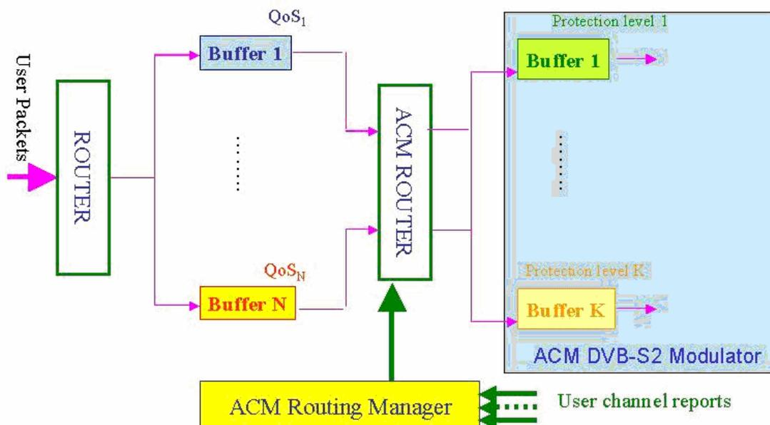
**Figure 22: Block diagram of a possible system architecture with multiple DVB-S2 input streams (one per protection level)**
