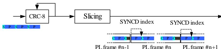
**Figure 28: Slicing process with padding and SYNCND index value**
