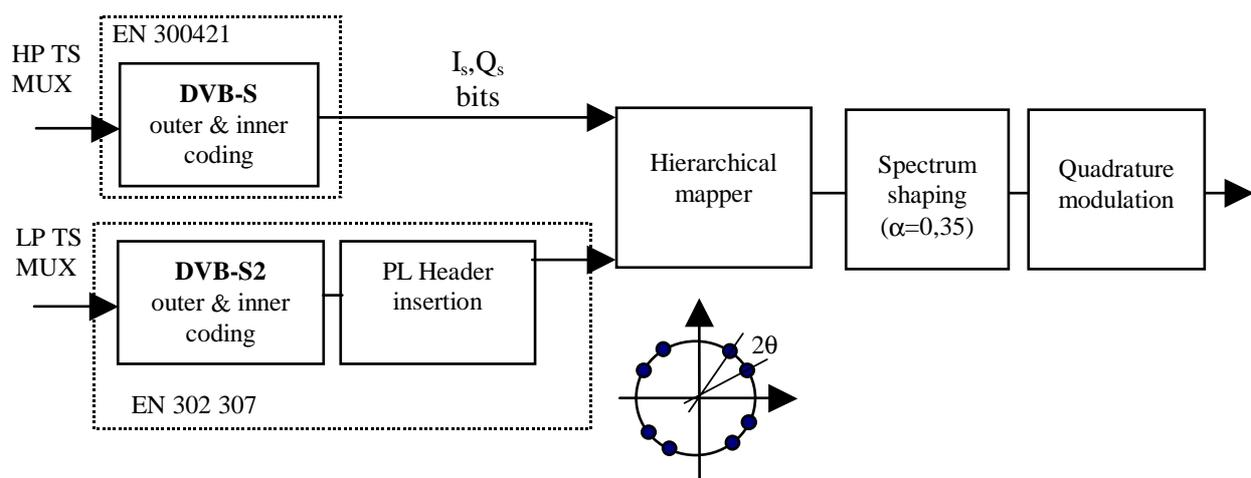
Figure 10: Functional block diagram of hierarchical backward compatible DVB-S2 system
