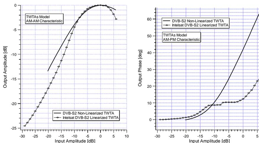
Figure 7: AM/AM and AM/PM characteristic of DVB-S2 linearized (LTWTA) and non linearized TWTA (NL-TWTA) models
