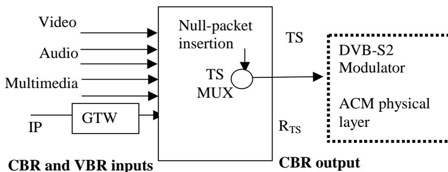
**Figure 14: MPEG TS multiplexing scheme**
