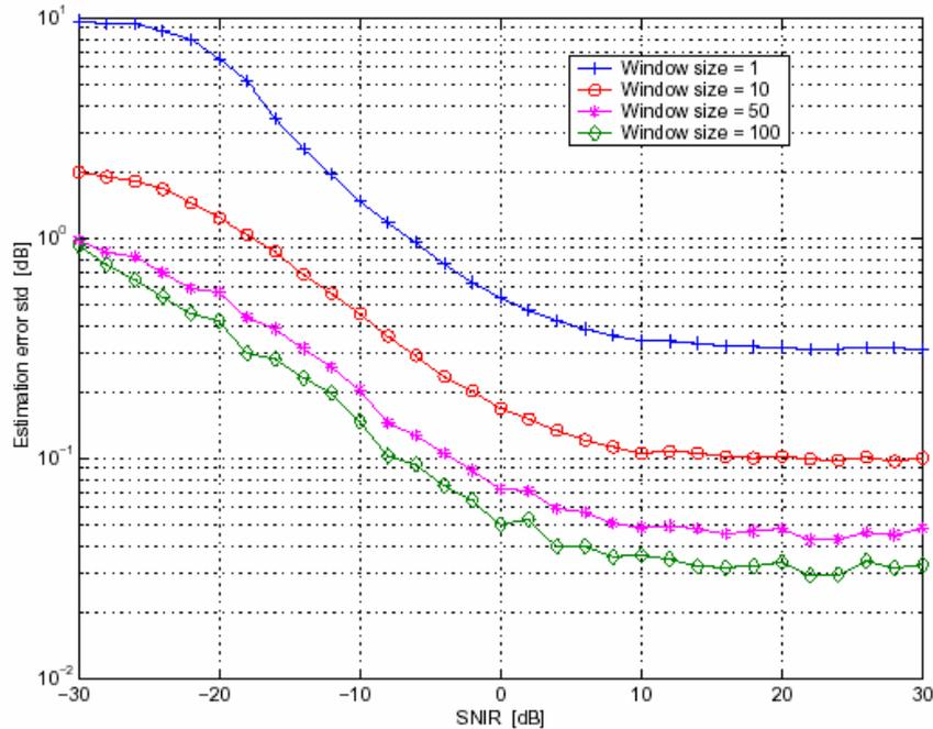
Figure E.2: SNORE channel estimator simulated standard deviation:  $N_p = 202$ ,  $N_{slot} = 2\ 204$  chips
