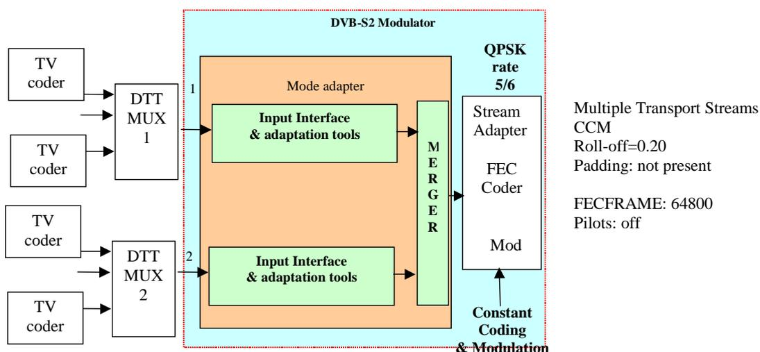
Figure 29: Example of DVB-S2 configuration for multiple DTT multiplexes distribution
