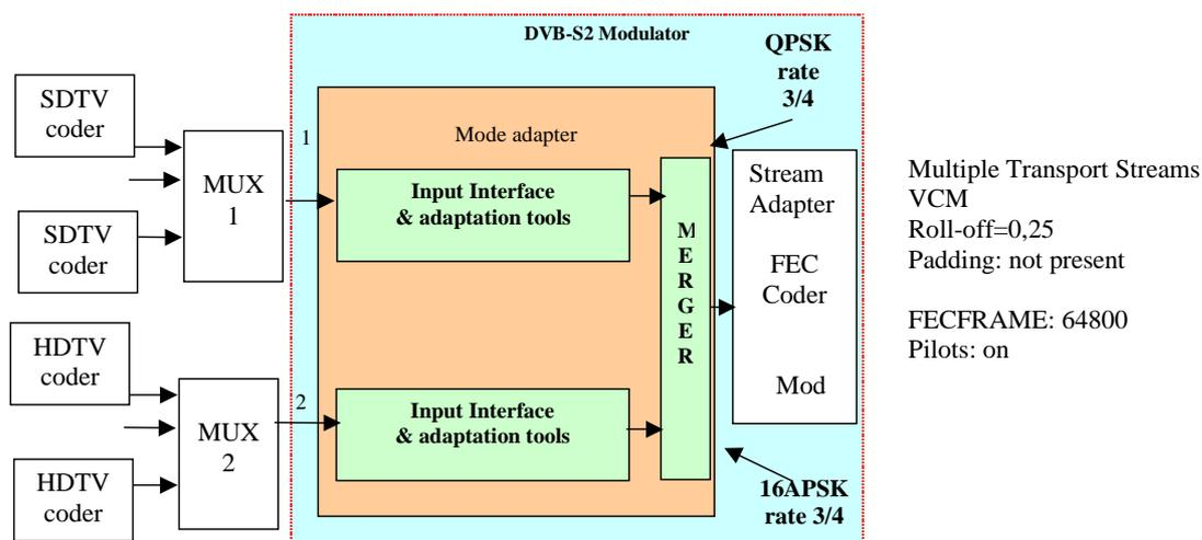
**Figure 17: Example DVB-S2 configuration for TV and HDTV broadcasting using VCM**
