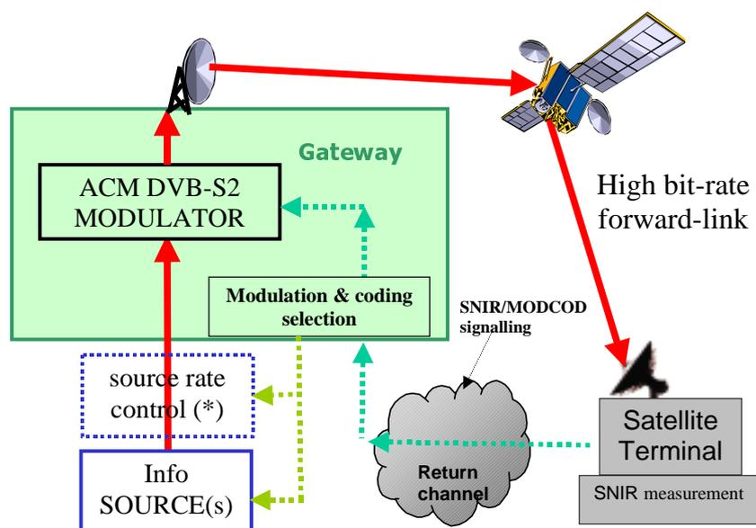
(\*) Source rate control may be directly applied to source(s) or locally at the GTW input or via network traffic control
