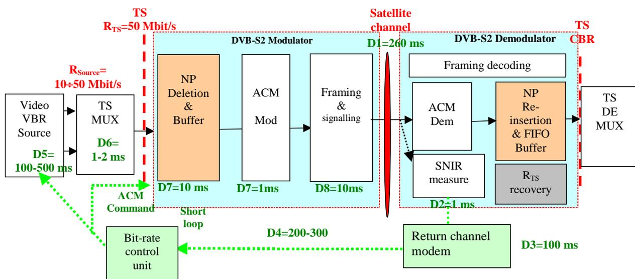
Figure 41: Single TS - uniform protection for long periods: transmission and receiving schemes
