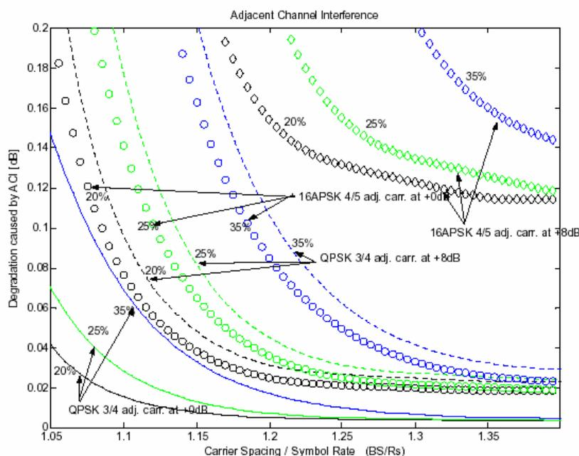
NOTE: Curves are shown for all roll-off factors and for an interfering carrier level +0 dB and +8 dB above the carrier under test. Use this figure with caution if the assumptions listed in the main text are not satisfied.
