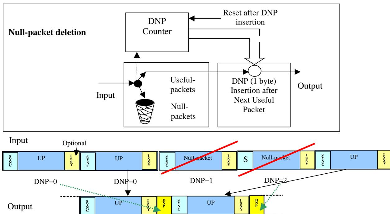
Figure 15: Null-packet deletion and DNP field (1 byte) insertion
