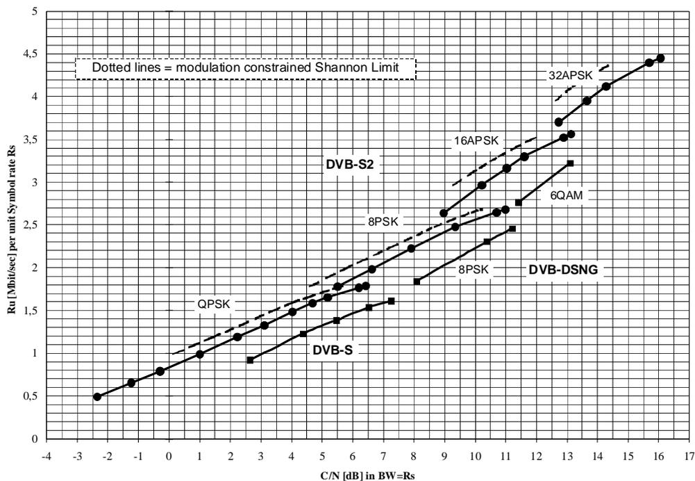
**Figure 3: Required C/N versus spectrum efficiency, obtained by computer simulations on the AWGN channel (ideal demodulation) (C/N refers to average power)**
