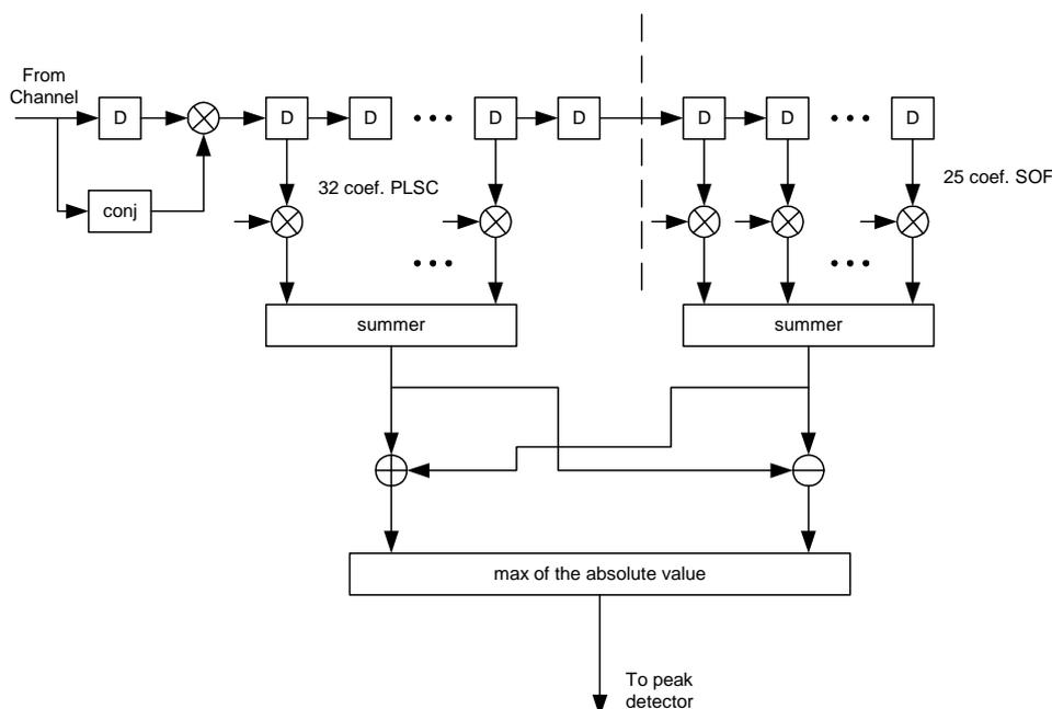
**Figure C.2: Differential detection of the SOF and PLSCODE**
