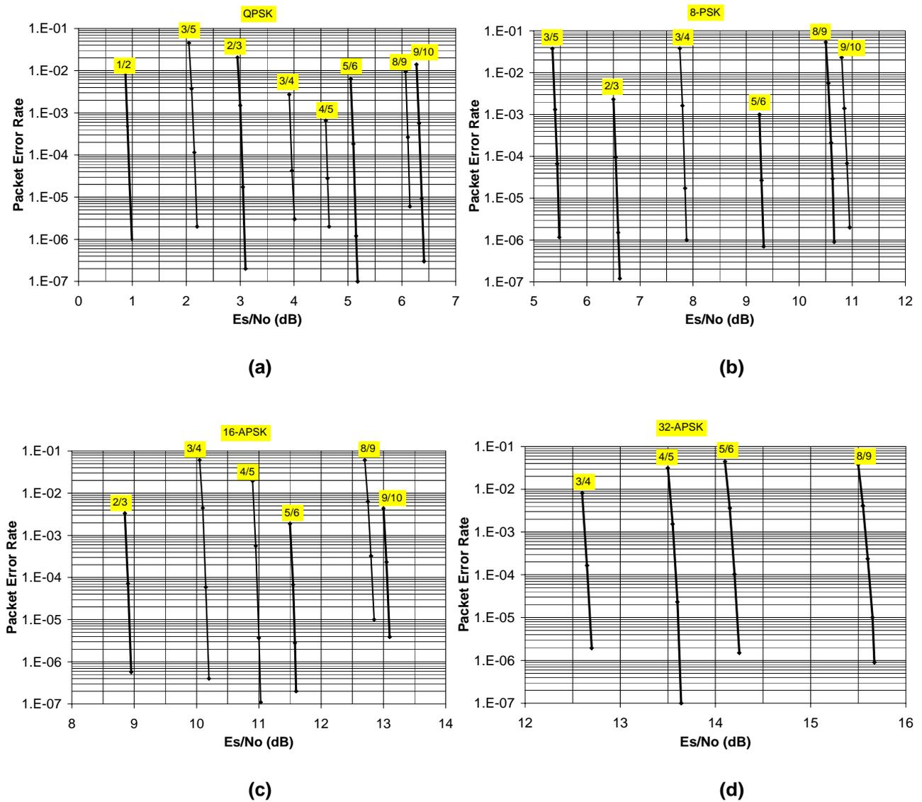
Figure A.3: Performance of LDPC+BCH Codes over AWGN Channel,  $N = 64\ 800$  bits,
