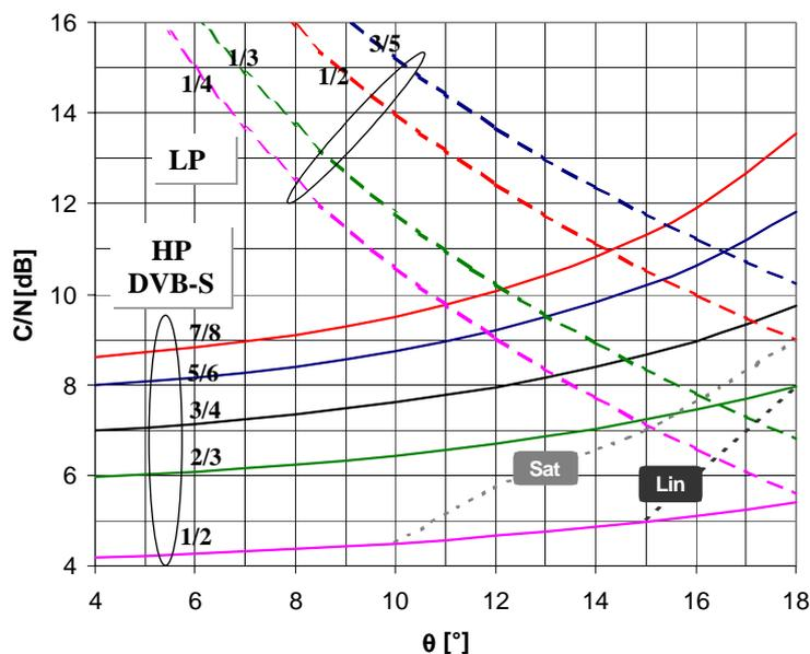
**Figure 11: required CNR of the HP and LP bit-stream versus the non uniform 8PSK constellation angle  $\theta$  on the AWGN channel, for the different code rates of DVB-S on the HP stream and DVB-S2 on the LP stream. Grey dashed lines indicate the cycle slip limits**
