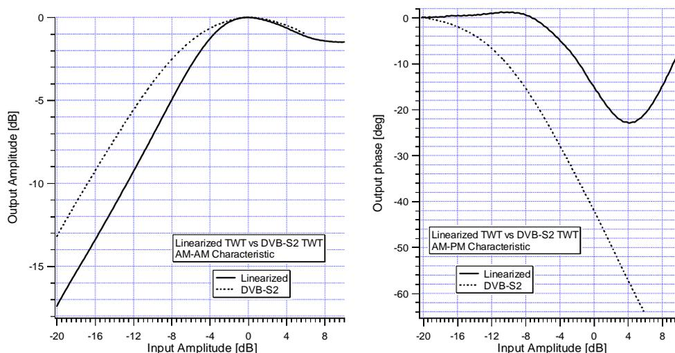
Figure 8: AM/AM and AM/PM Characteristic of linearized TWTA LTWTA2
