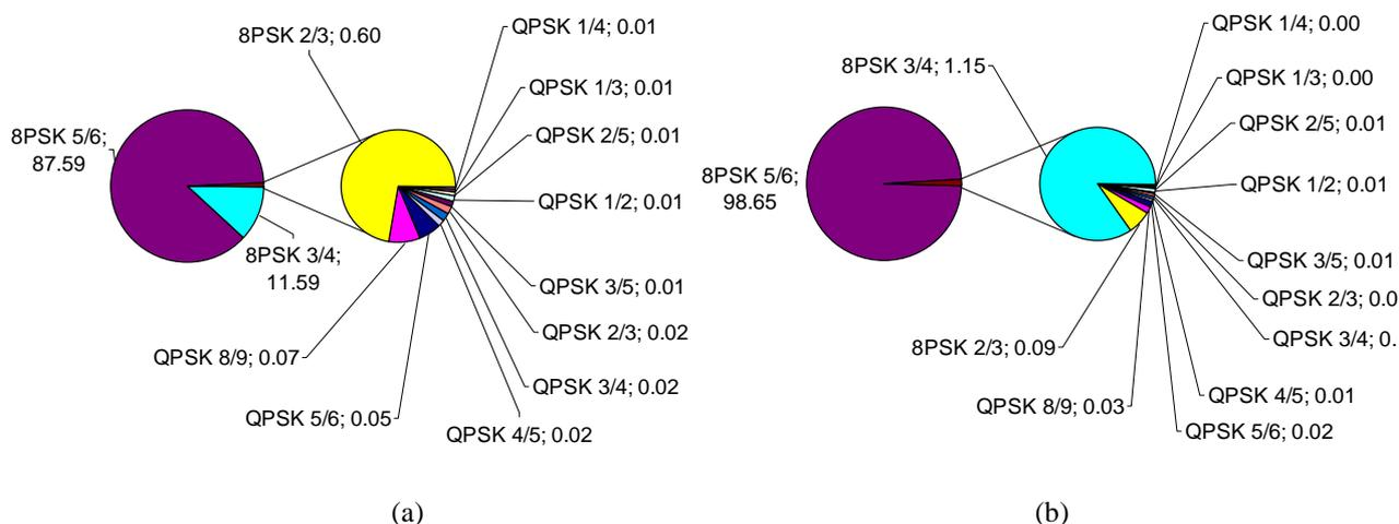
**Figure D.6: Distribution of Modulation and coding usage for the reference system (a) with reduced satellite HPA EIRP (57,8 dBW satellite EIRP EOC) and (b) with full power (60,5 dBW satellite EIRP EOC) implementing only QPSK and 8PSK**
