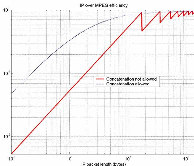
**Figure 24: IP over MPEG encapsulation efficiency**
