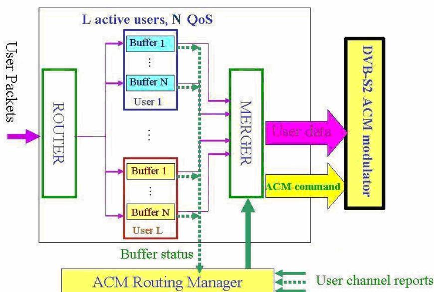
**Figure 20: Block diagram of a possible system architecture with single generic stream input to the ACM DVB-S2 modulator**
