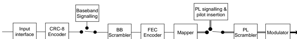
**Figure 16: Simplified block diagram of the DVB-S2 system for the broadcast profile, single transport stream and CCM configuration**
