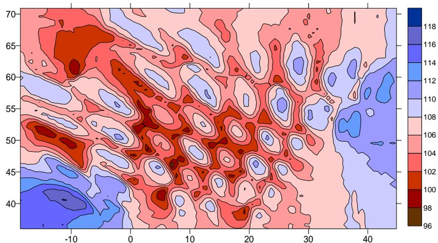
Figure D.3: Contour-plot of the C/I<sub>0</sub> for the down-link of the transparent Forward-Link scenarios
