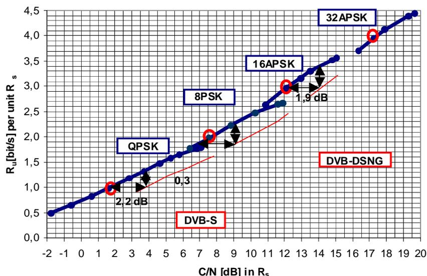
**Figure 6: Examples of  $R_U$  versus required C/N by satellite, in single carrier per transponder configuration**
