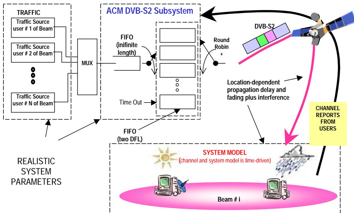
Figure 26: Block diagram of the jointly time and event driven simulator
