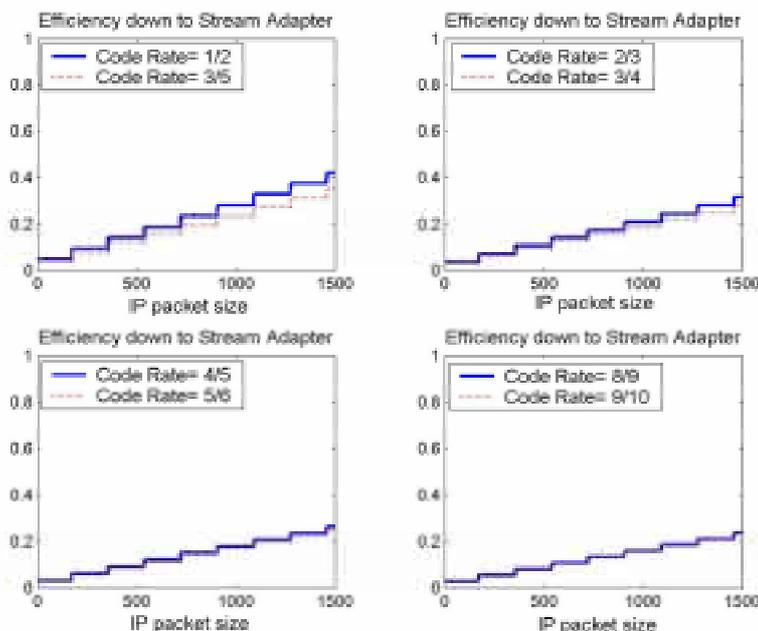
NOTE: Encapsulation efficiency ( $\psi_{MS}(\eta, L)$ ) for a single IP packet: large efficiency may be achieved only for multiple IP packets encapsulation.
