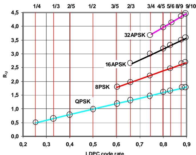
Figure 5: examples of useful bit rates  $R_u$  versus LDPC code rate per unit symbol rate  $R_s$
