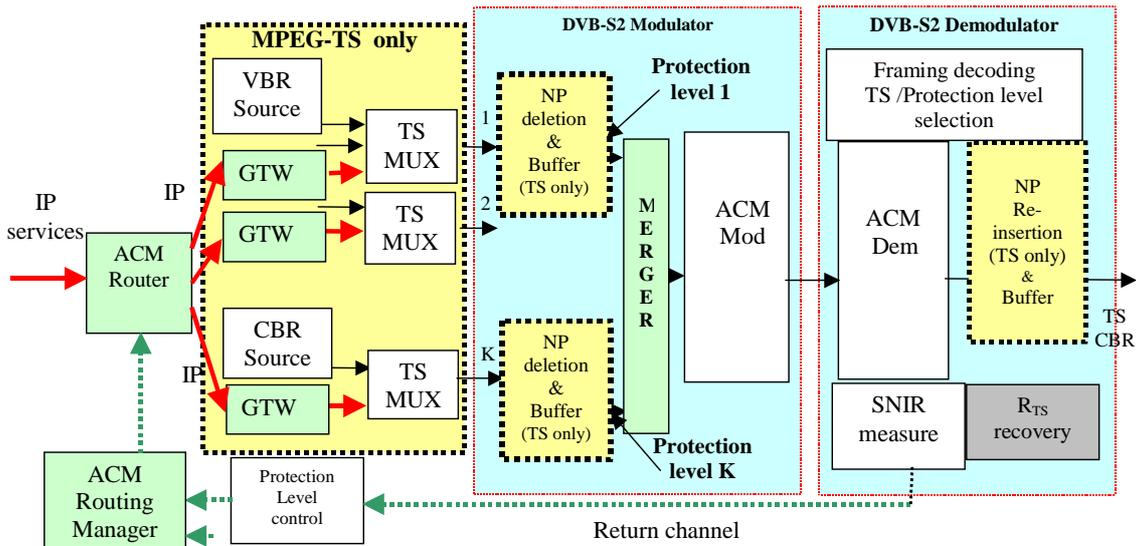
NOTE: For Generic input Streams, GTWs, TS Muxes and null-packet deletion are not required.
