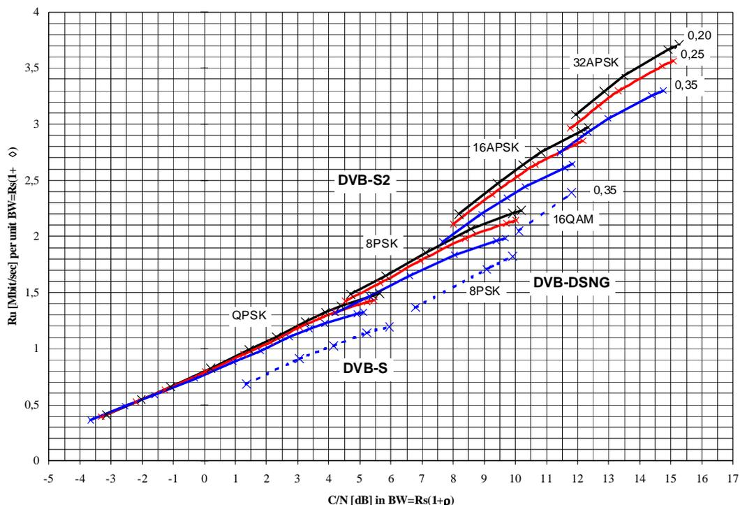
**Figure 4: Required C/N versus spectrum efficiency for constant satellite bandwidth  $BW = R_S(1+\rho)$  on the AWGN channel (ideal demodulation) (C/N refers to average power)**
