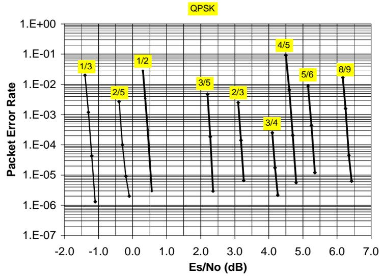
Figure A.4: Performance of LDPC+BCH Codes over AWGN Channel, N = 16 200 bits
