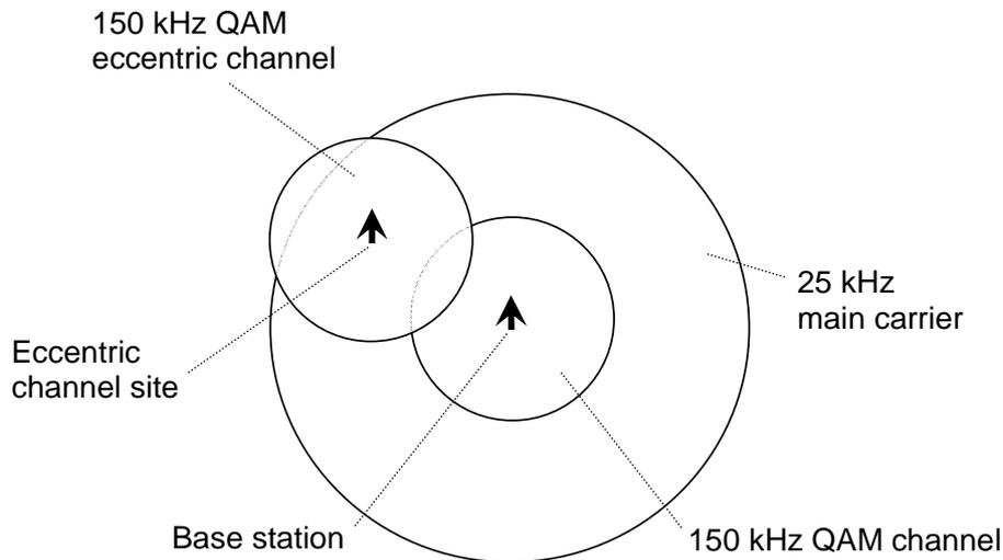
Figure 7.22: Example of a cell using an eccentric channel
