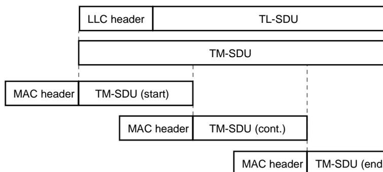
**Figure 7.7: MAC fragmentation of a long TM-SDU**
