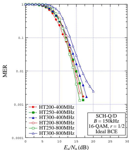
**Figure C.2:** MER vs.  $E_b/N_0$  for  $B = 150$  kHz ,
