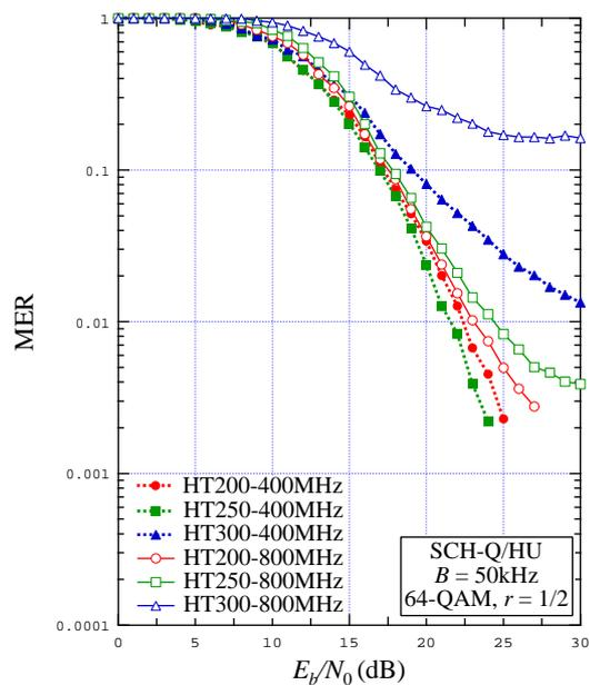
Figure 8.7: MER vs.  $E_b/N_0$  for  $B = 50$  kHz ,
