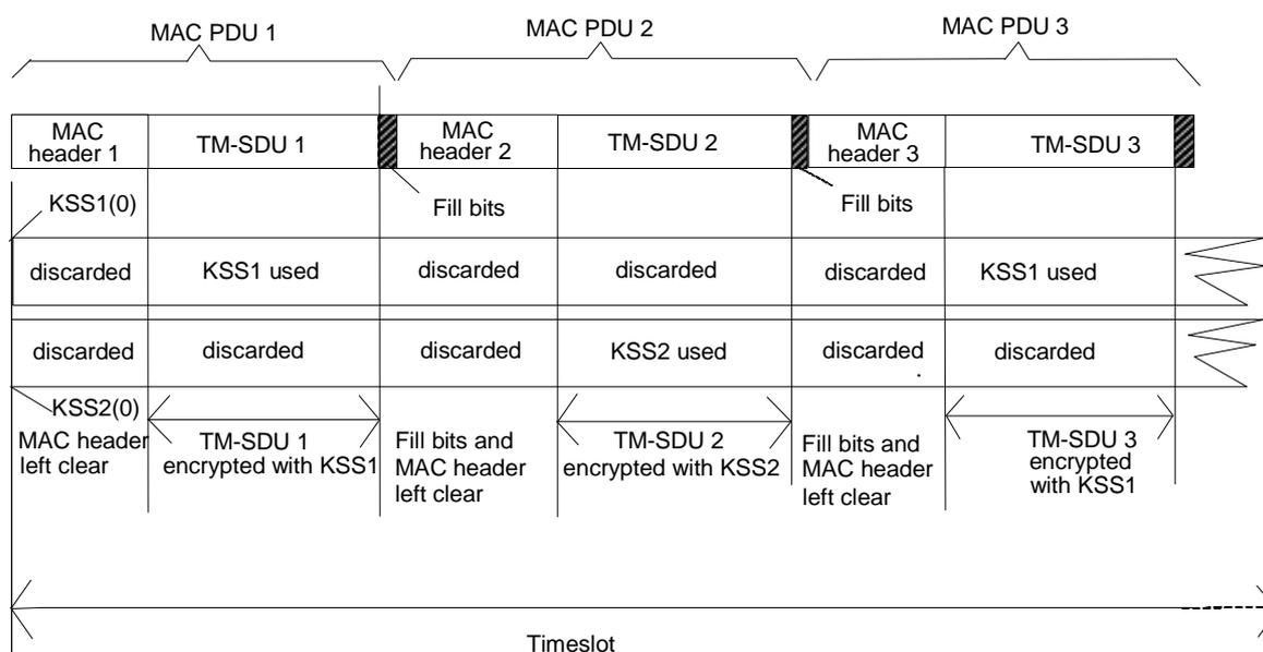
NOTE: In this example, TM-SDU 1 and TM-SDU 3 use the same cipher key but TM-SDU 2 uses a different cipher key.
