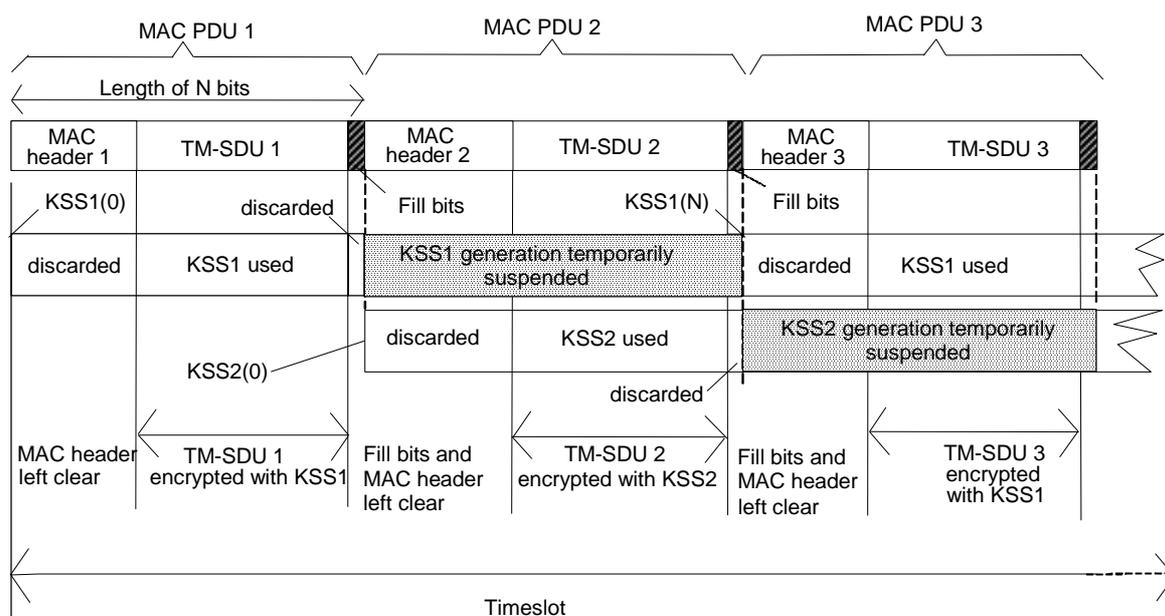
NOTE: In this example, TM-SDU 1 and TM-SDU 3 use the same KSS but TM-SDU 2 uses a KSS derived from a different DCK.
