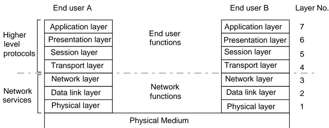
**Figure 4.1: OSI reference model for communication architectures**
