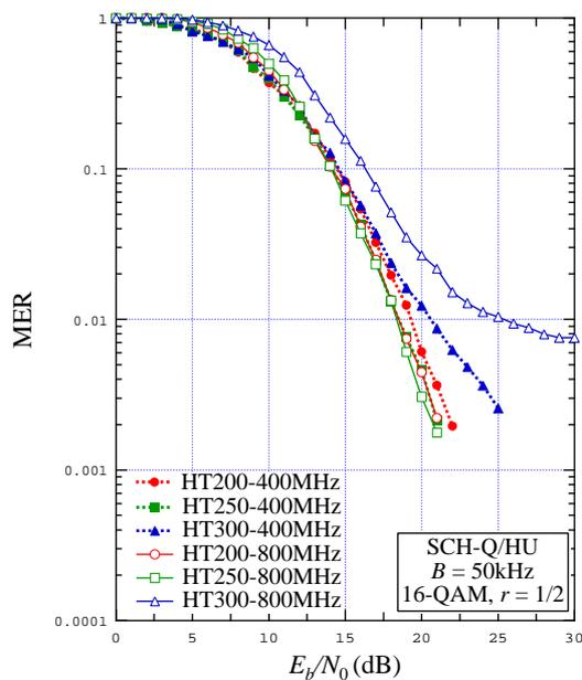
Figure 8.6: MER vs.  $E_b/N_0$  for  $B = 50$  kHz ,
