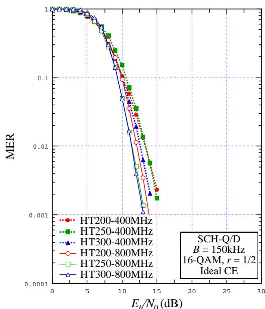
**Figure C.1:** MER vs.  $E_b/N_0$  for  $B = 150$  kHz ,
