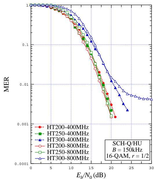
Figure 8.9: MER vs.  $E_b/N_0$  for  $B = 150$  kHz ,
