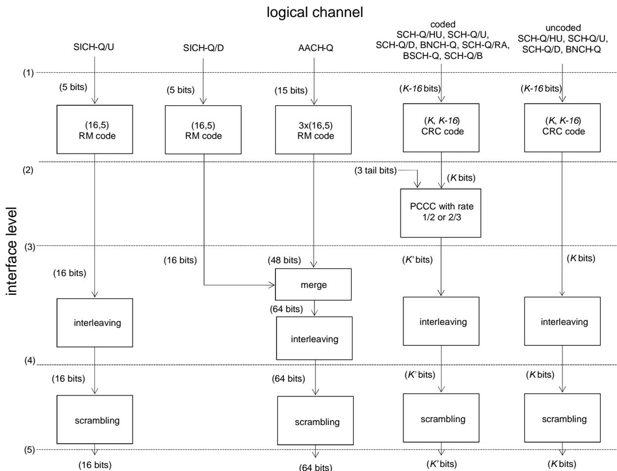
**Figure 6.14: Error control structure for QAM logical channels**
