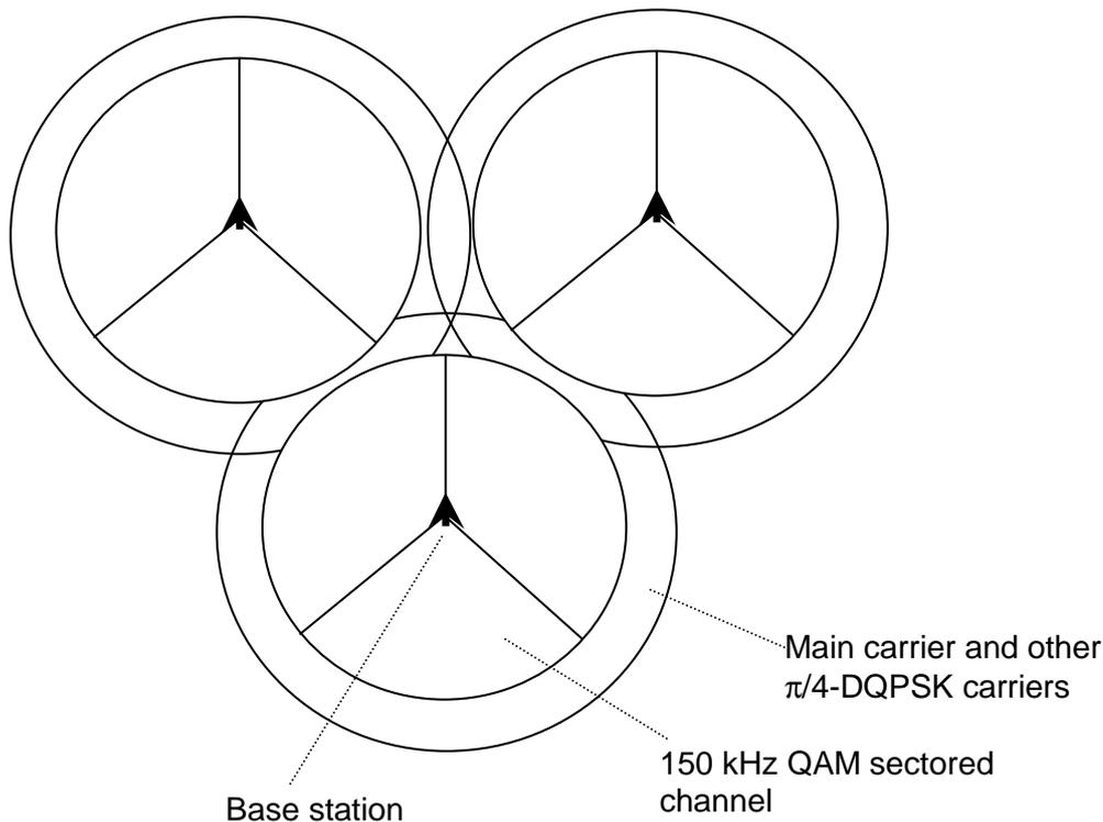
**Figure 7.19: Example of CA cells using sectored channels**
