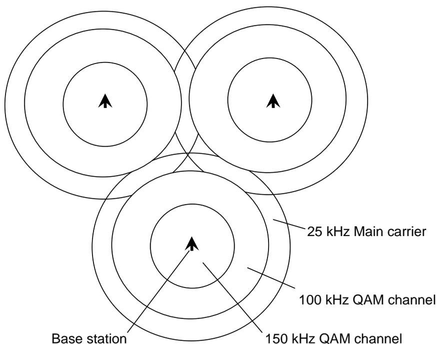
**Figure 7.18: Example of cells using non-conforming concentric channels**
