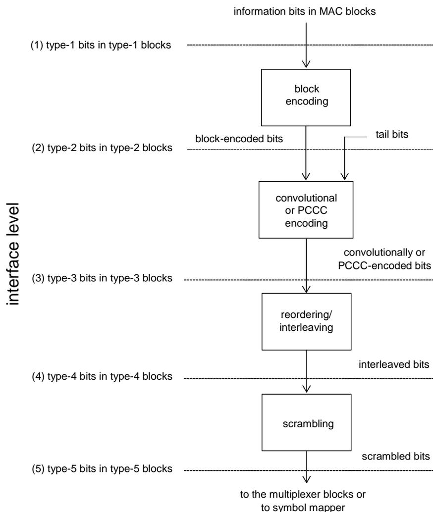
**Figure 6.13: Interfaces in the error control structure**
