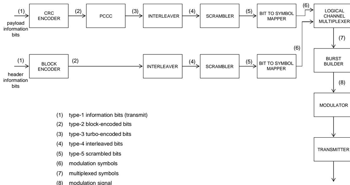
Figure 6.7: Reference configuration for QAM
