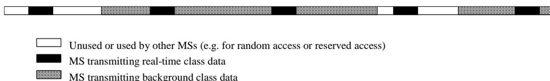
**Figure 7.17: Example of usage of the uplink channel**
