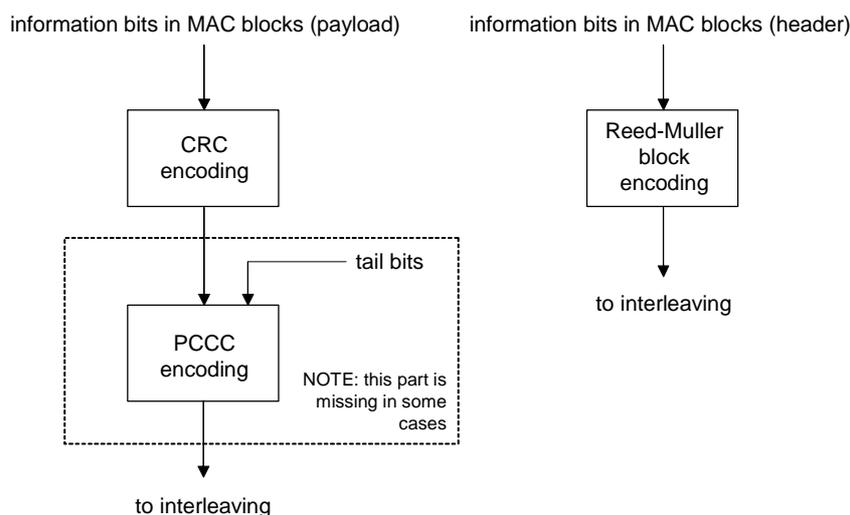
**Figure 6.15: Encoding levels for QAM channels**
