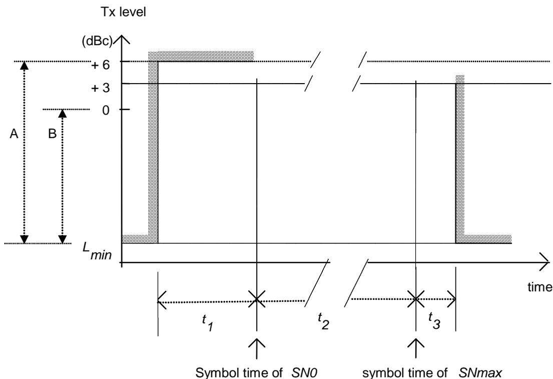
A: Mask height specified for phase modulation.
