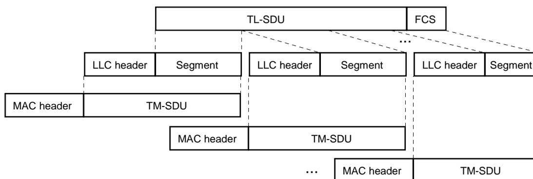
**Figure 7.8: Advanced link segmentation by the LLC**
