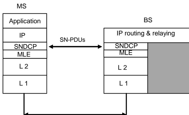
**Figure 7.3: Usage of TETRA packet data IP applications**
