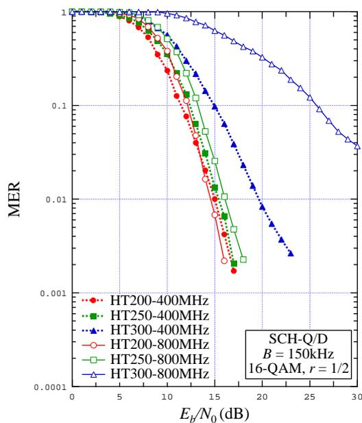
Figure 8.8: MER vs.  $E_b/N_0$  for  $B = 150$  kHz ,
