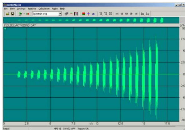
Figure 10: Periodical repetition of the Composite Source Signal to determine the activation sensitivity under single talk conditions
