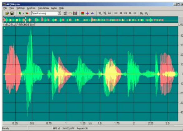
Figure 23: Enlarged time sequence from a double talk sequence (real speech sample, green: male voice, red: female voice)
