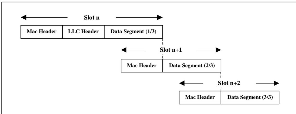
**Figure 2: Spanning Advanced Link Segments**
