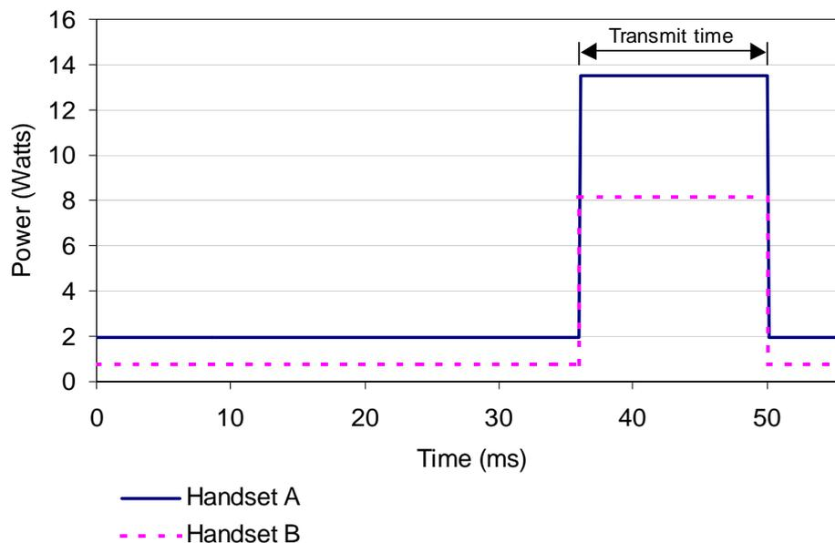
**Figure 1: First Generation Handset Power Consumption Profiles**
