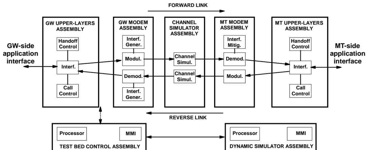
Figure 10.5: Top level diagram of ROBMOD
