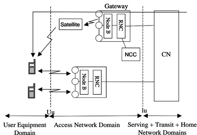
**Figure 7.8: Direct reception from the satellite**
