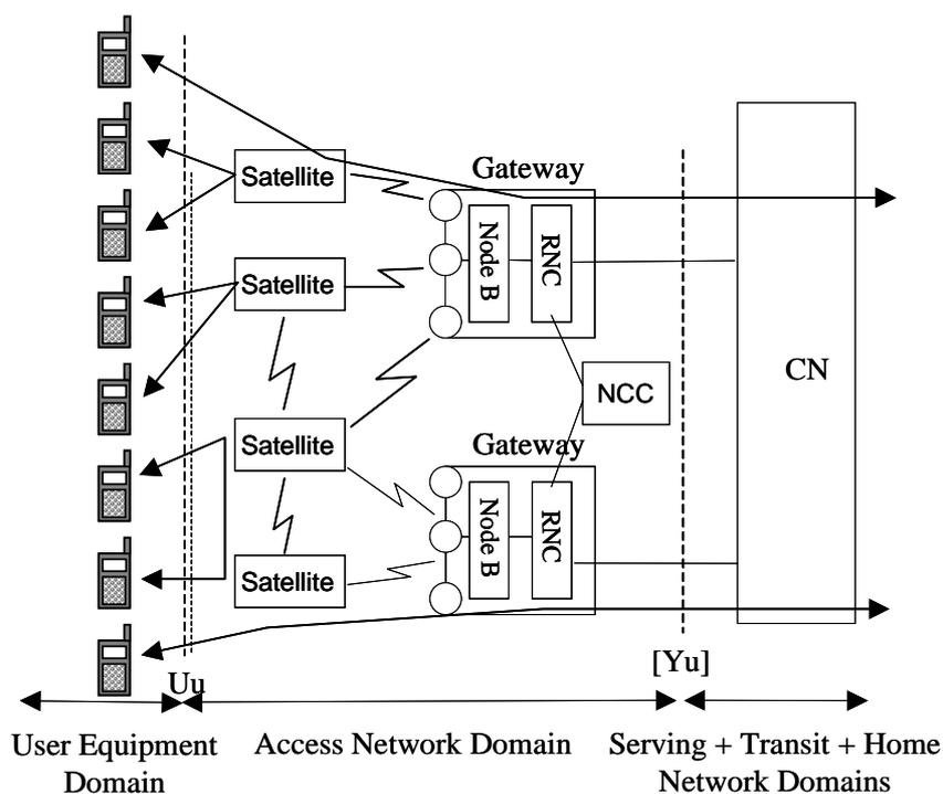
Figure 7.5: GEO and/or Non-GSO reference architecture using regenerative satellites
