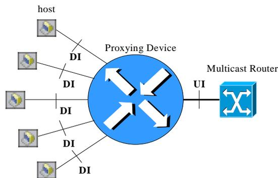
**Figure 8.7: Standard IGMP proxying interfaces classification**
