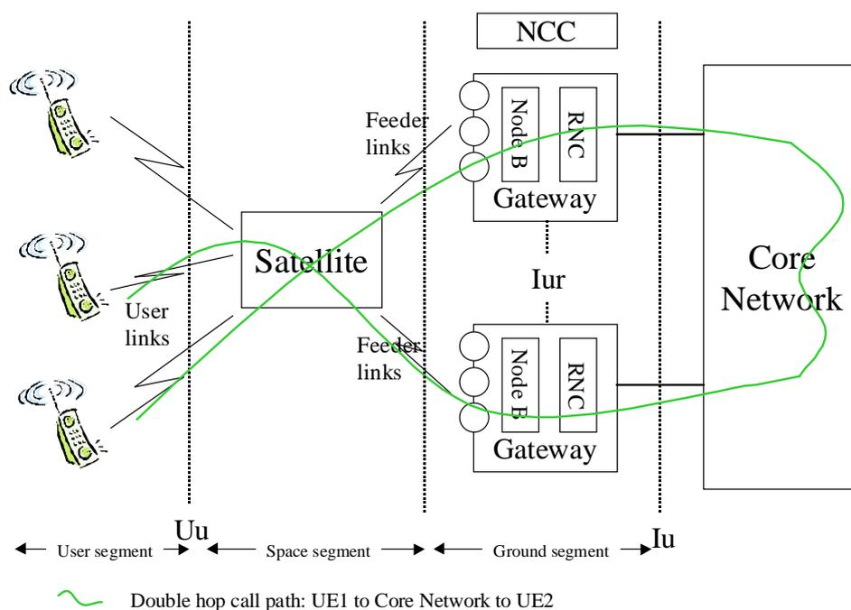
**Figure 7.10: Double-hop, GSO model for S-UMTS**
