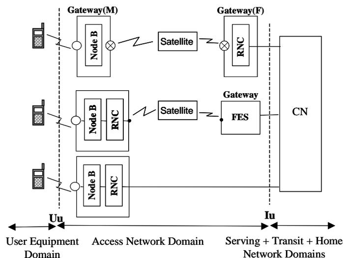
**Figure 7.6: Indirect access to satellite - Collective configuration**
