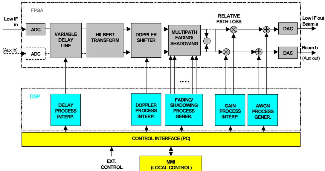
Figure 10.4: Channel Simulator block diagram
