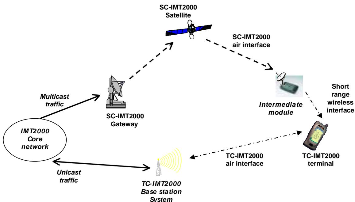
Figure 5.6: Broadcast oriented - Indirect access to satellite - Source [24]
