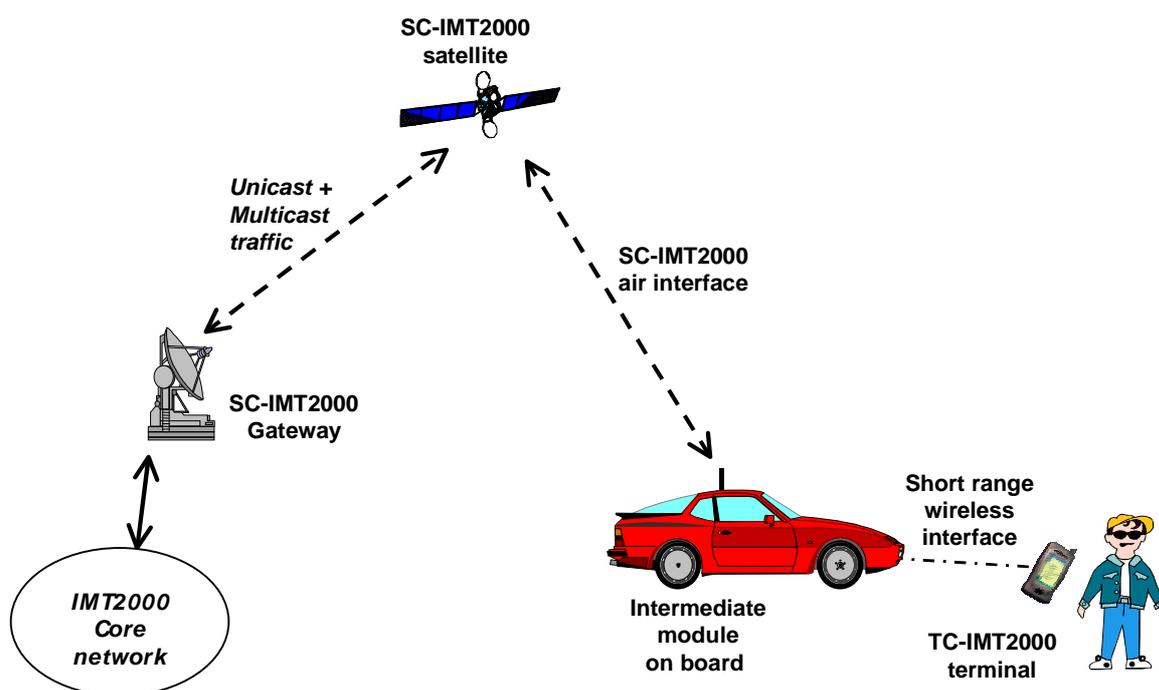
**Figure 5.4: Indirect access to satellite - individual configuration - Source [24]**
