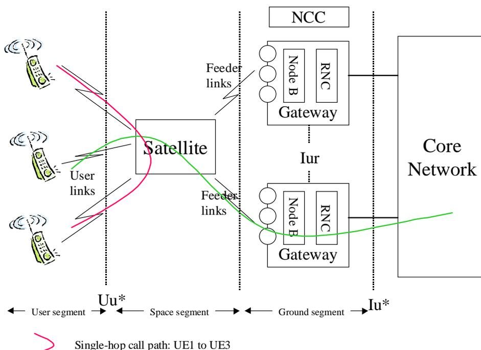
Figure 7.11: Single-hop, GSO model for S-UMTS
