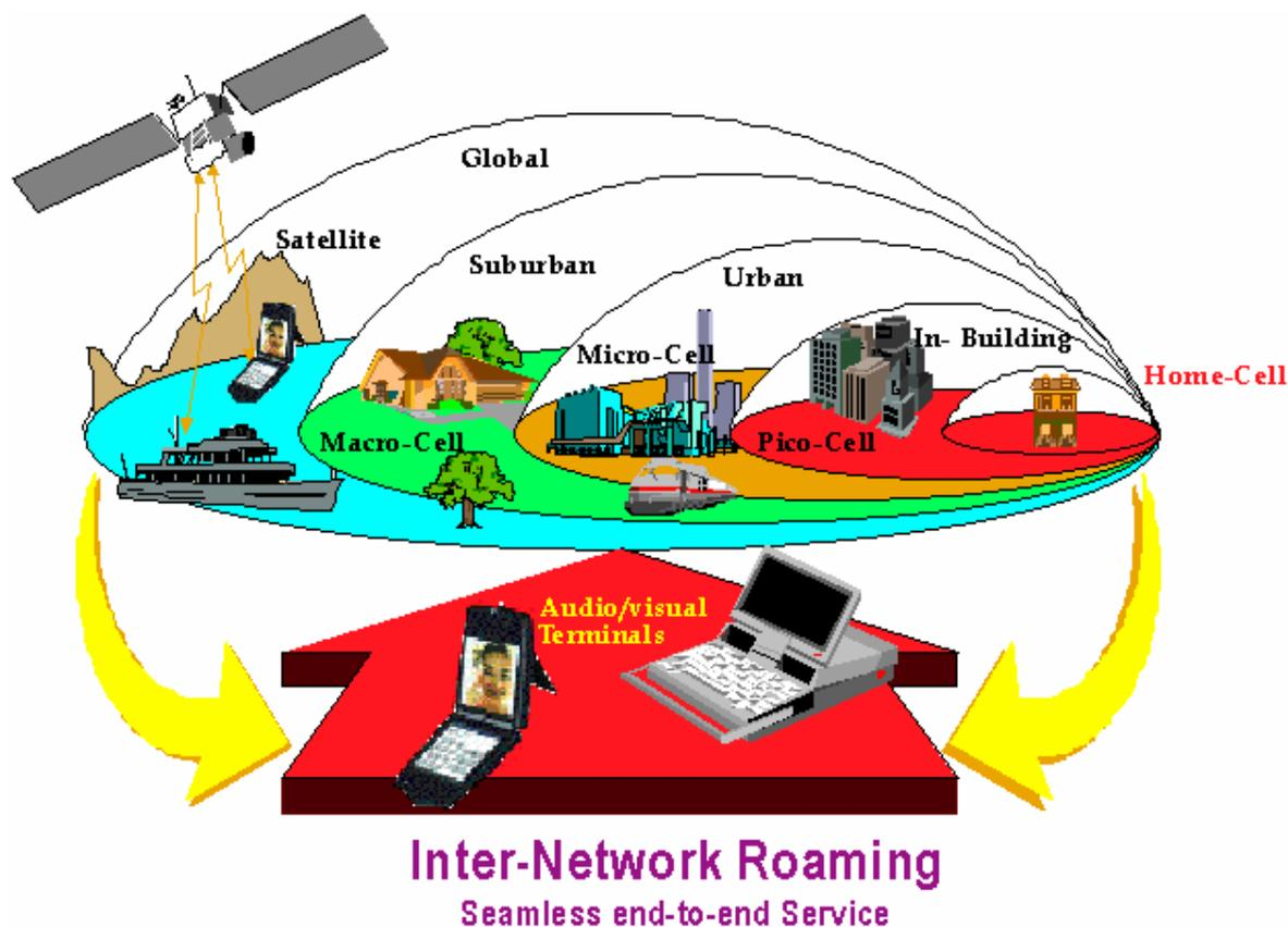
Figure 4.2: The role of S-UMTS as an integral part of the UMTS network (UMTS Forum)
