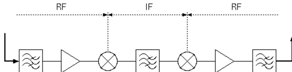
**Figure 6.16: Basic architecture for simple unidirectional IMR**
