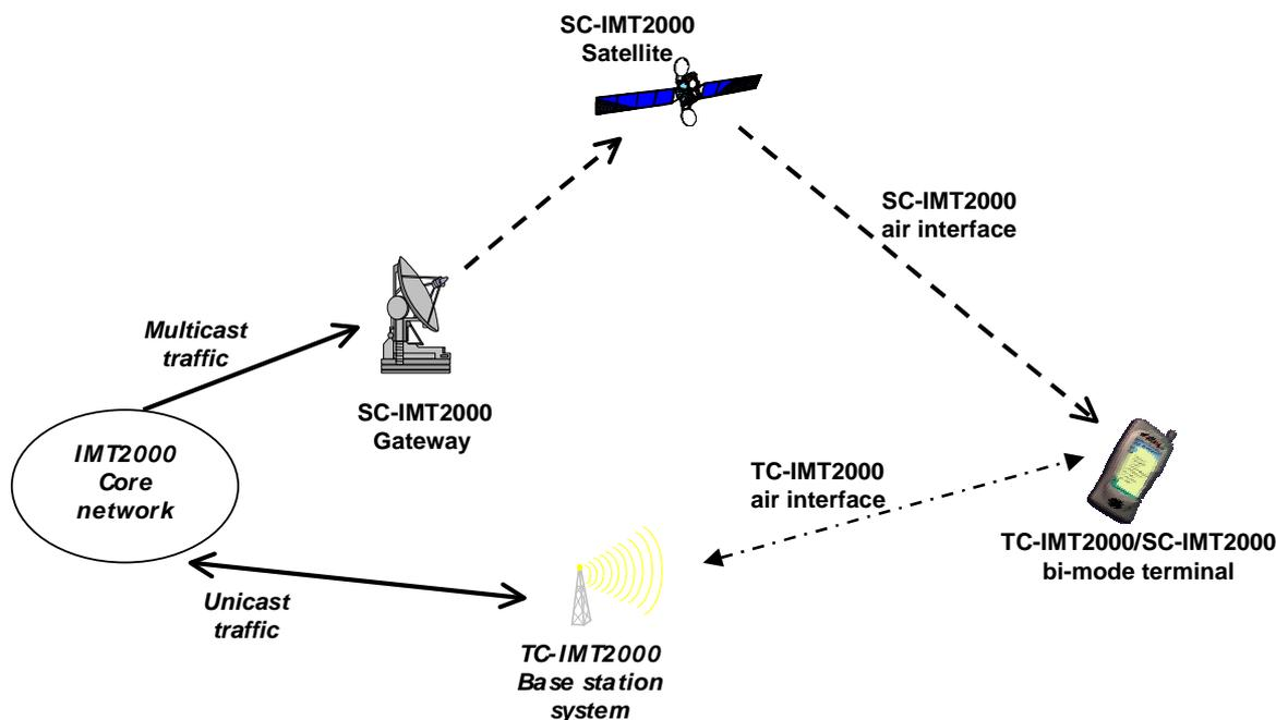
Figure 5.7: Direct access to satellite (Broadcast oriented) - Source [24]
