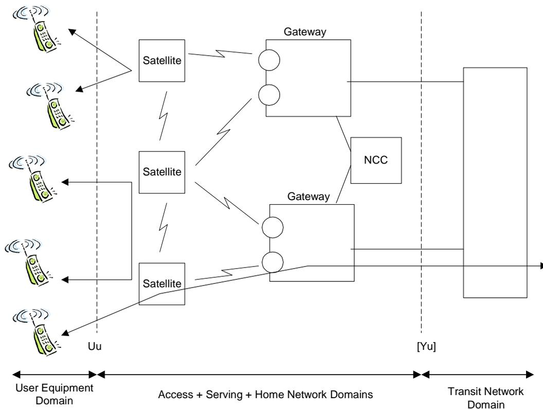
**Figure 7.13: Single-hop, regenerative, ISL, LEO model for S-UMTS**
