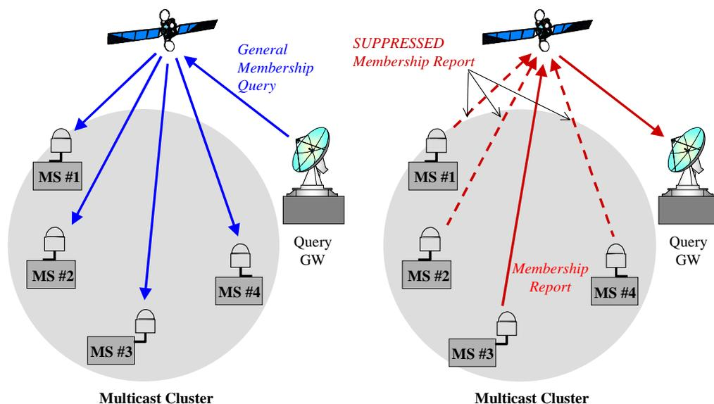
**Figure 8.8: Principle of IGMP overhead reduction**
