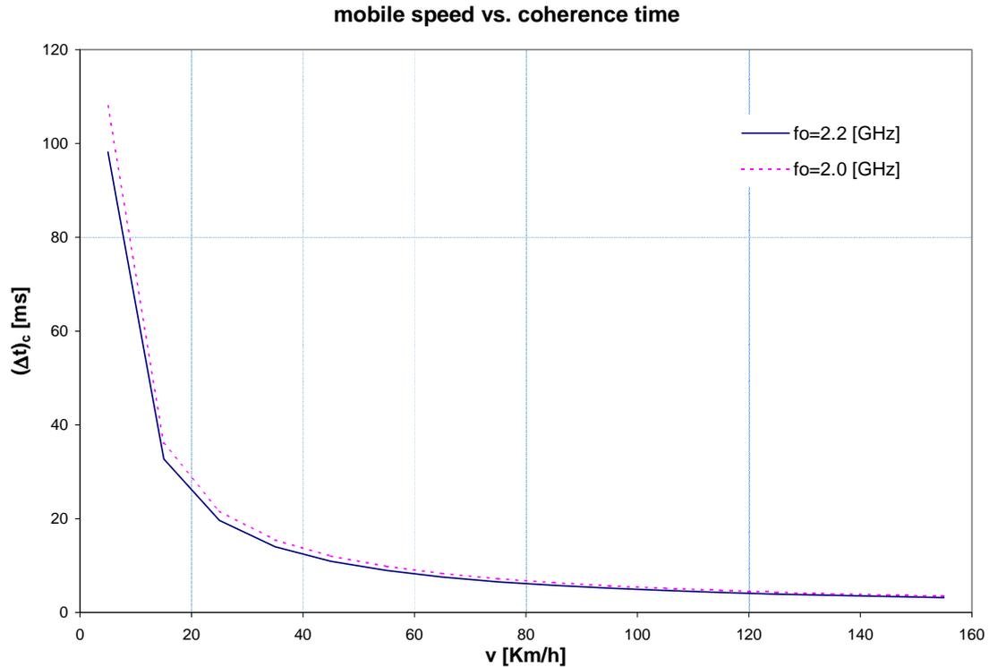
**Figure 8.2: Channel coherence time as a function of the MT speed in Km/h**
