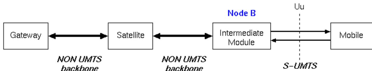
Figure 6.12: IMR with full Node B functionality
