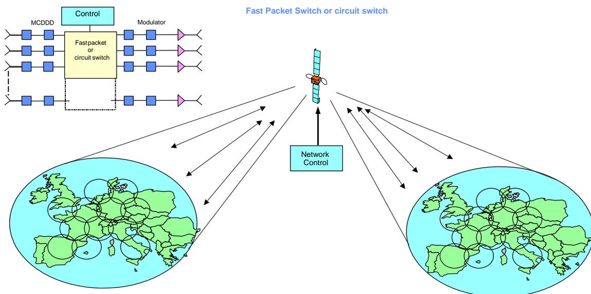
Figure 7.20: Multi-beam full Regenerative satellite
