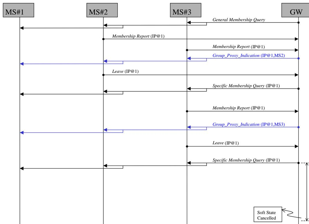
**Figure 8.9: Example of IGMP proxying with overhead reduction**
