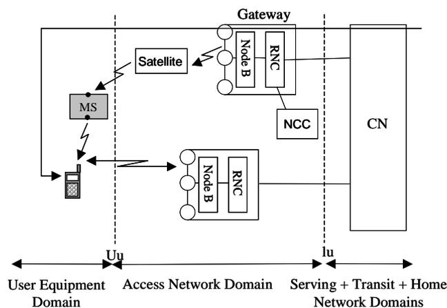
**Figure 7.9: Indirect reception from the satellite**
