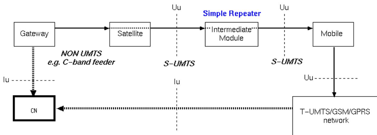
Figure 6.9: Simple unidirectional repeater
