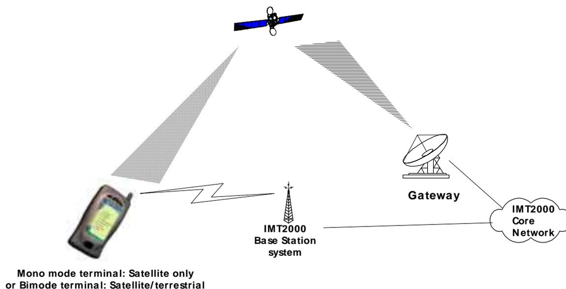
**Figure 5.3: Direct access to satellite configuration - Source [24]**
