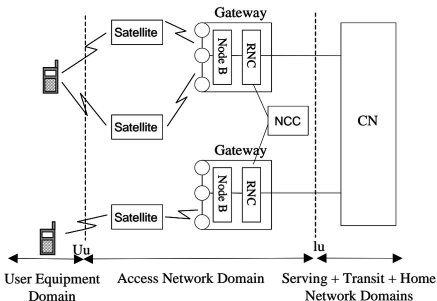
Figure 7.4: GEO and/or Non-GSO reference architecture for S-UMTS
