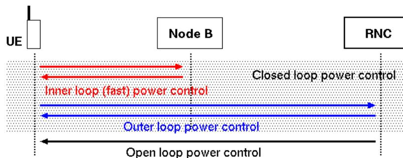
Figure 6.11: W-CDMA power control mechanisms
