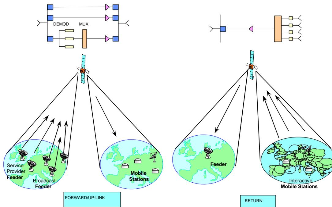
**Figure 7.19: Regenerative/bent-pipe Forward Links and Transparent multiplexed Return Links**
