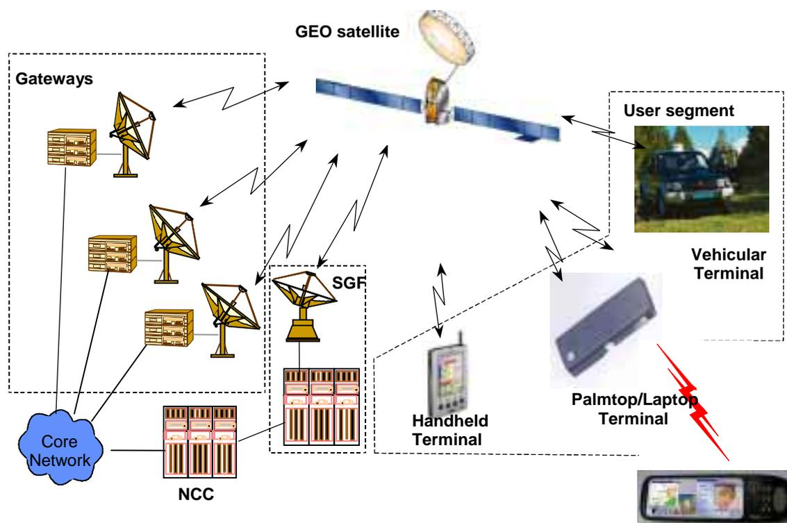
**Figure 7.12: GSO system example for S-UMTS**
