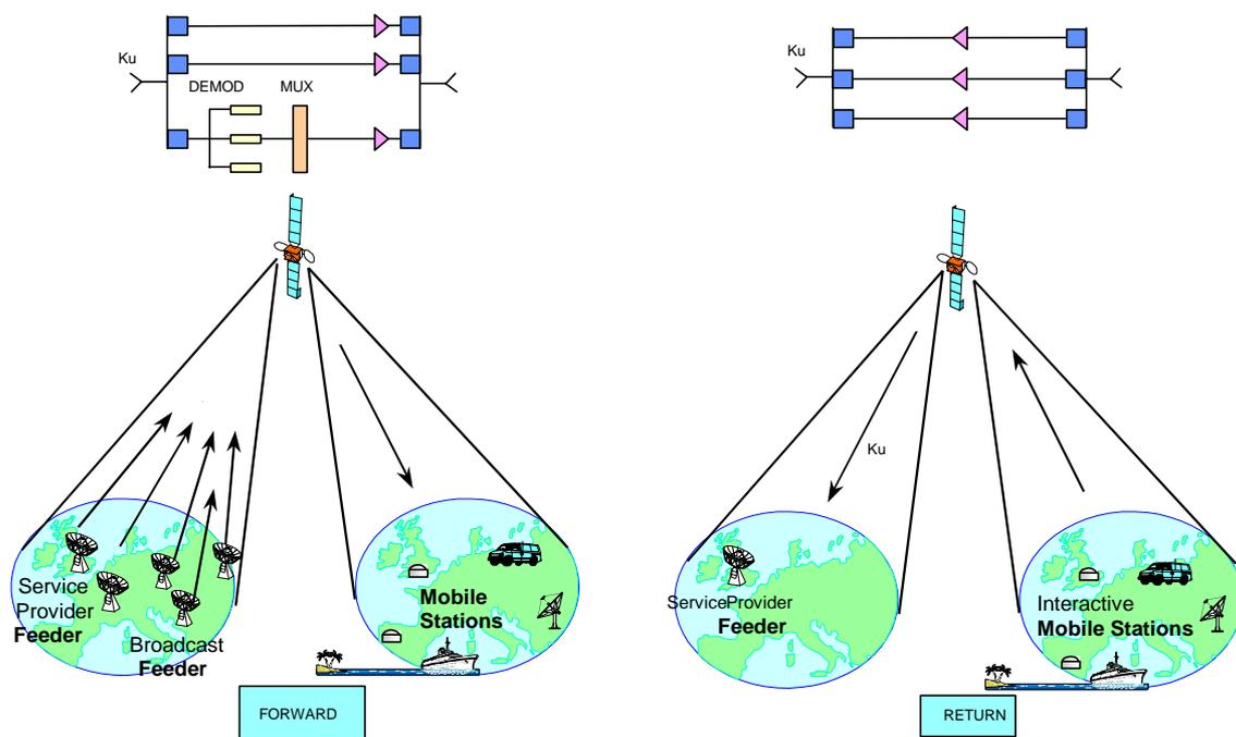
**Figure 7.18: Regenerative/bent-pipe Forward Links and Bent-pipe Return Links**
