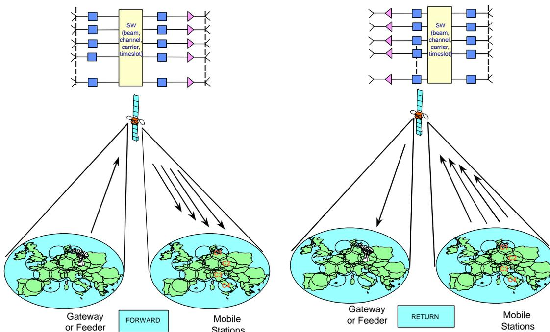
**Figure 7.17: Transparent On-Board Processing satellite with multi-beam**
