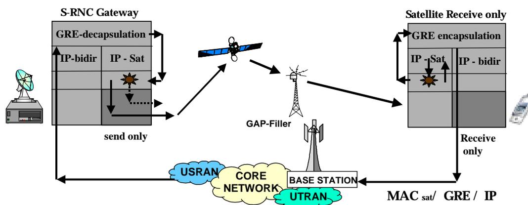
Figure 8.10: UDLR functionality in the unidirectional scenario
