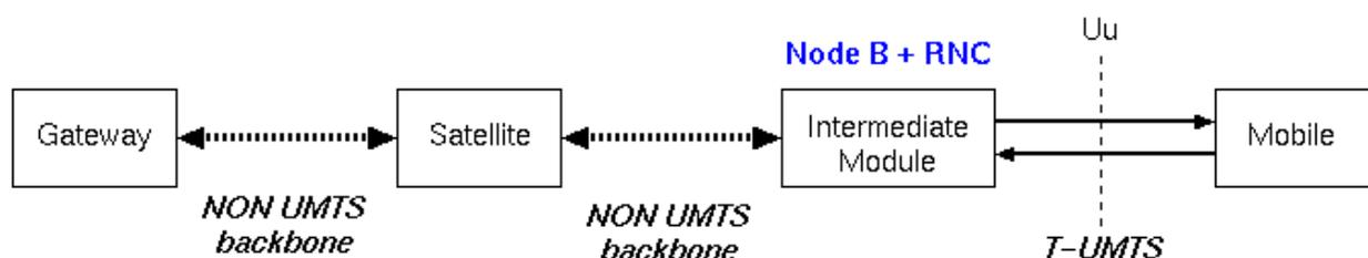
Figure 6.13: IMR with full Node B and RNC functionality
