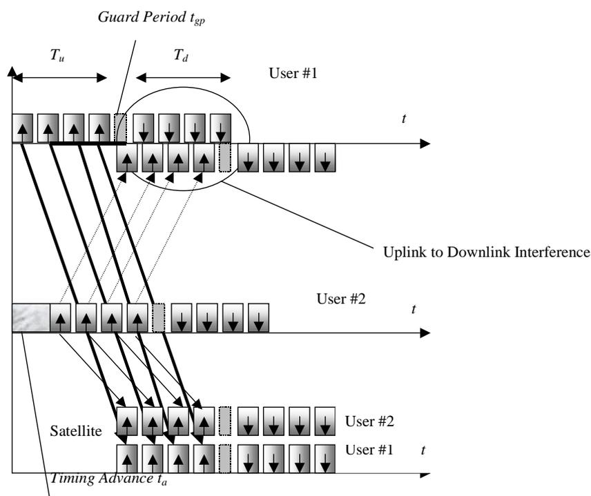
**Figure 8.5: Uplink/Downlink Other user interference scenario**
