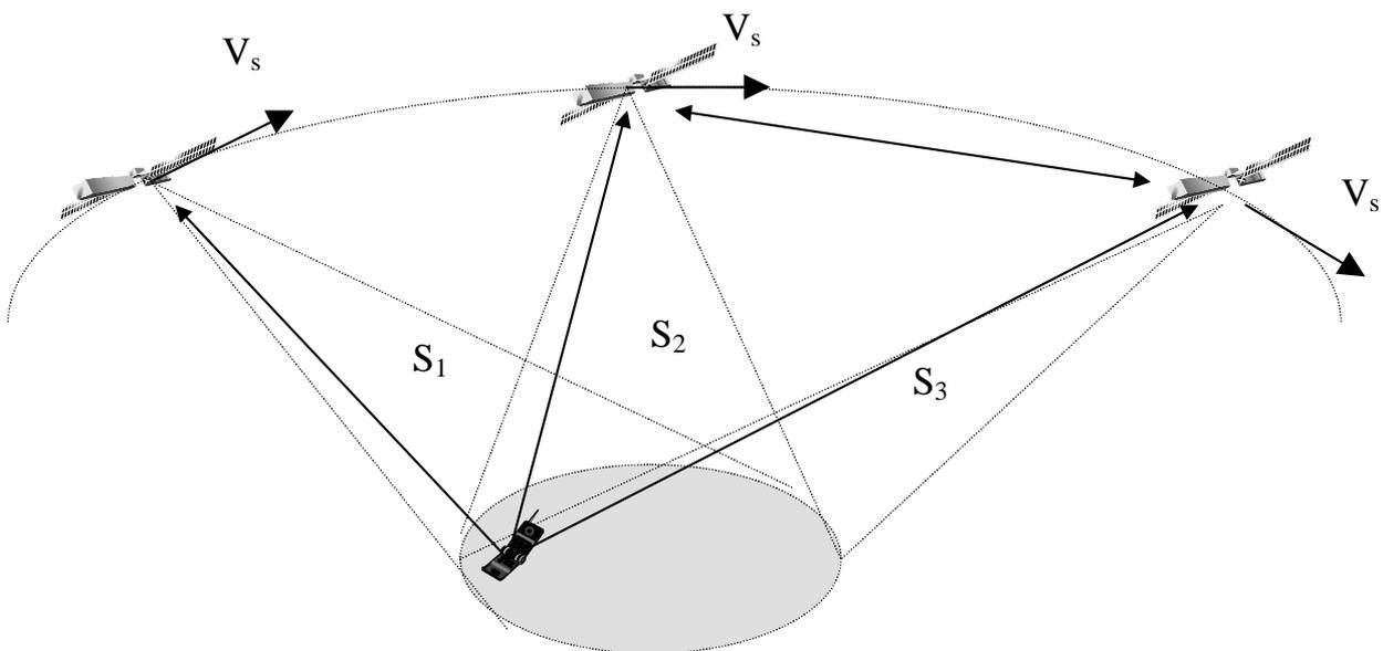
**Figure 8.3: Slant Range/Delay Variation**
