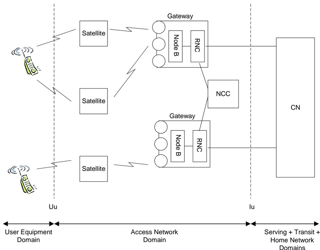
**Figure 7.14: Double-hop, bent-pipe, LEO model for S-UMTS**
