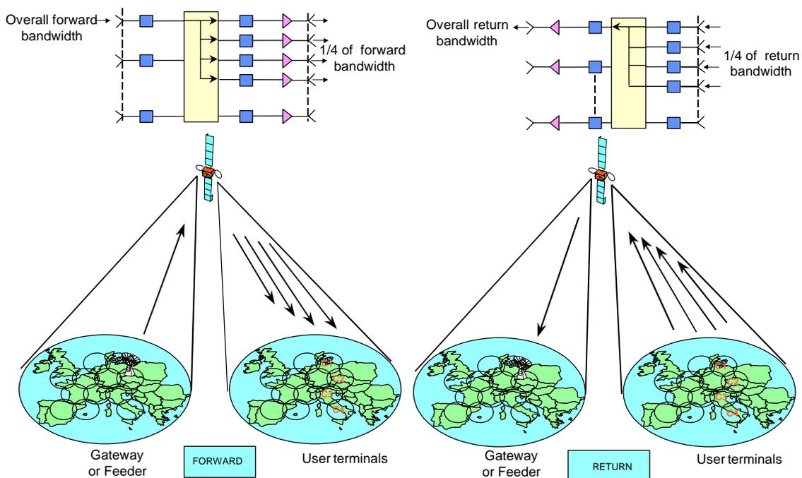
**Figure 7.16: Bent-pipe multi-beam satellite**
