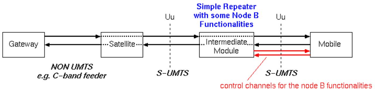
Figure 6.10: Simple IMR with a subset of node B functionalities
