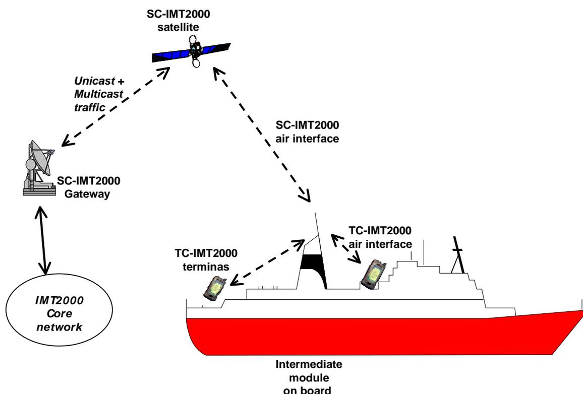
**Figure 5.5: Indirect access to satellite - collective configuration - Source [24]**
