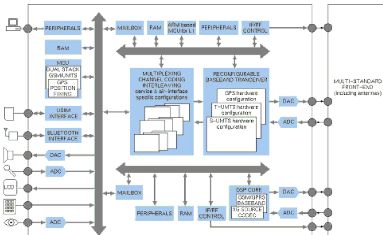
Figure 6.15: Multi-standard terminal architecture
