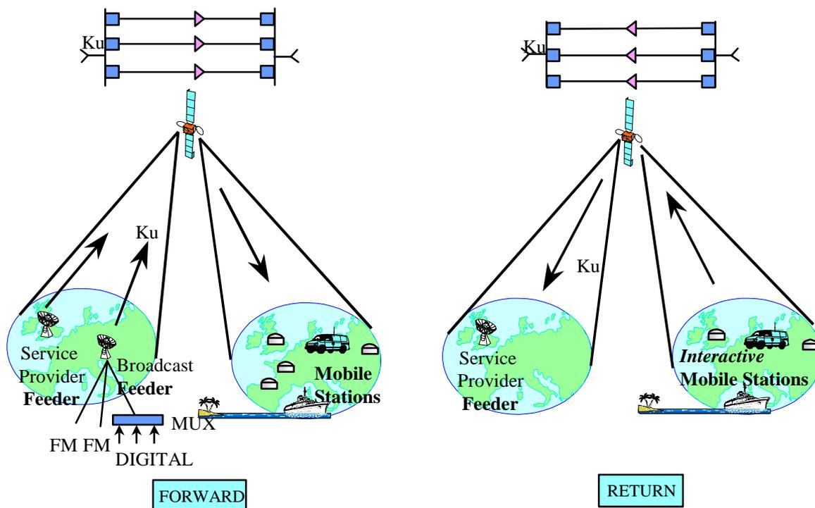
**Figure 7.15: Bent-pipe satellite with wide coverage**
