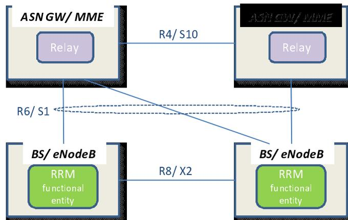
**Figure 4.2: RRM functional entities in the SOTA WiMAX™ and 3GPP LTE architectures**
