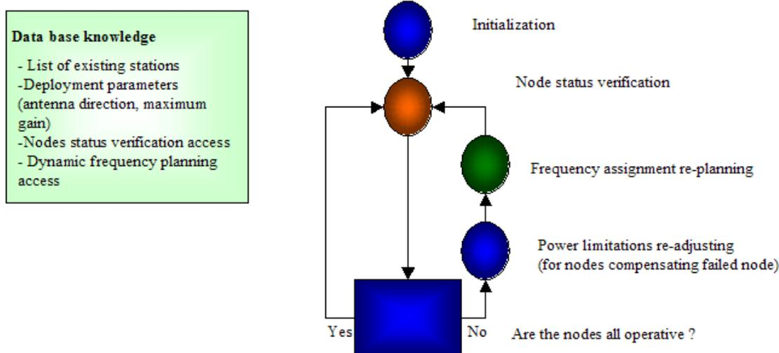
Figure 5.5: Station failure recovery procedure
