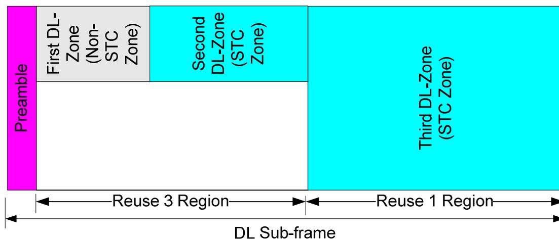
Figure 6.11: Example of FFR frame structure
