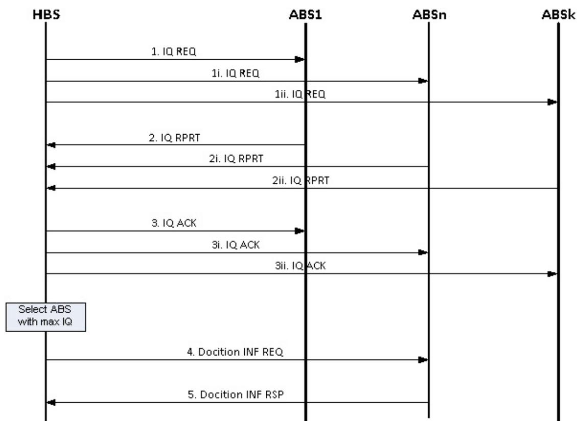
Figure 5.18: Request IQ procedure
