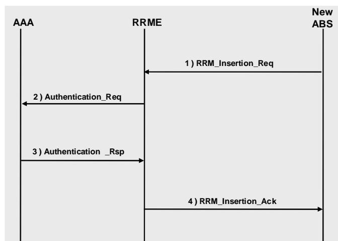
Figure 5.7: A new station insertion message flow
