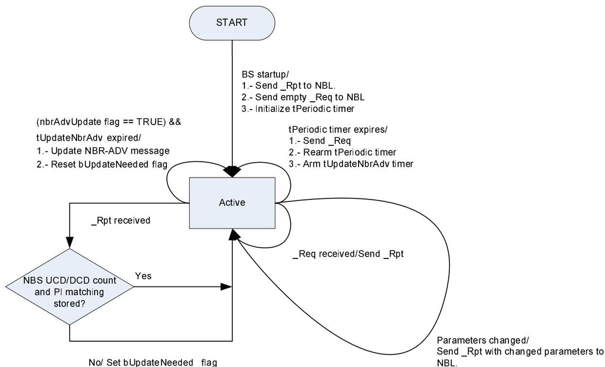
**Figure 6.9: BS radio configuration message state machine**
