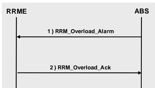
Figure 5.8: Overload alarm message flow
