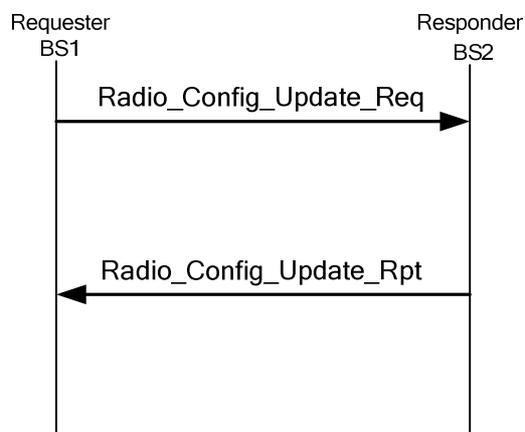
**Figure 6.7: Radio Configuration update (Pull)**
