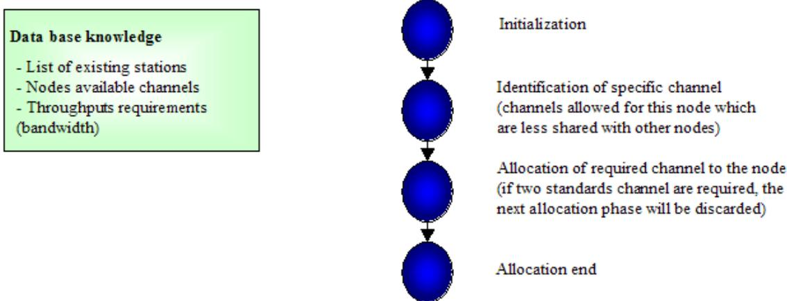
**Figure 5.4: Channel allocation process**
