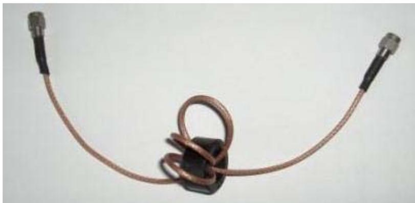
**Figure 17: Choke Absorber**
