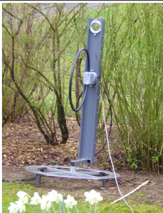
Loop Antenna (magnetic field) [i.10]
