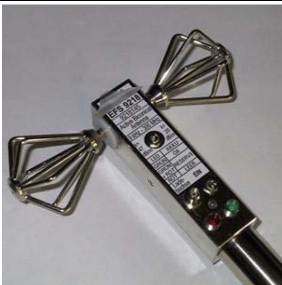
Biconical Active Electric Field Probe [i.8]
