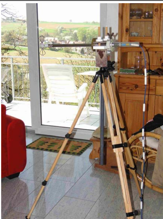
Biconical Antenna on wooden tripod
