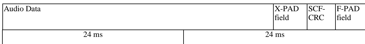
Figure 3.2.9: Case of Low Sampling Frequency (48 ms Audio frames)
