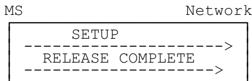
Figure 5.7b/GSM 04.08 Recall acceptance or rejection by user
