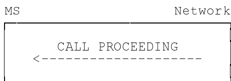
Figure 5.3/GSM 04.08 Call proceeding sequence at mobile originating call establishment
