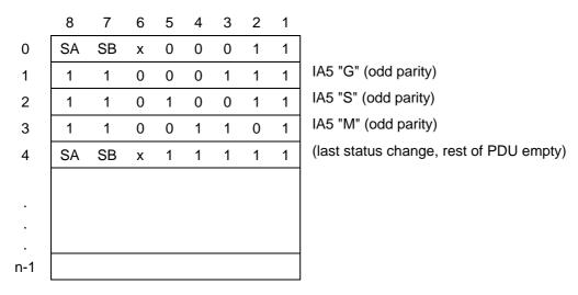
Figure 2a Single-link RLP and multi-link RLP with status octet transfer in PDU.
