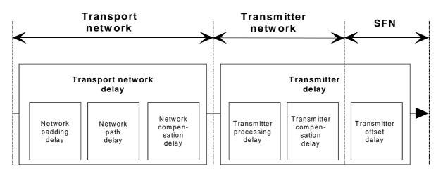
Figure 13: Distribution and transmission network delays
