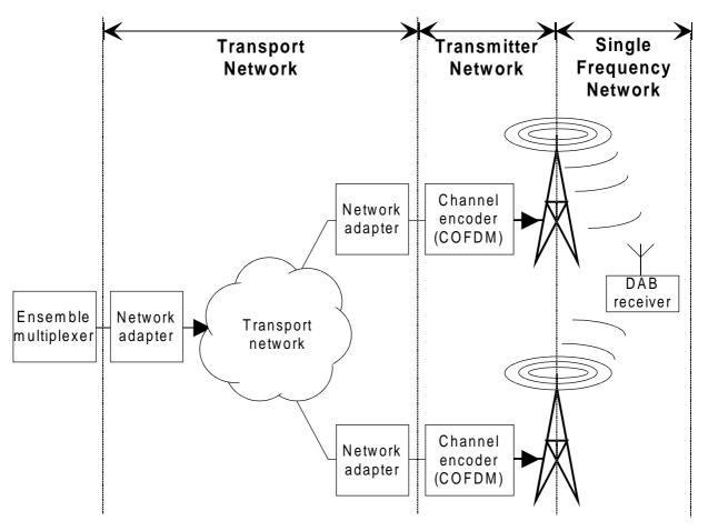
Figure 12: General Structure of Single Frequency Networks
