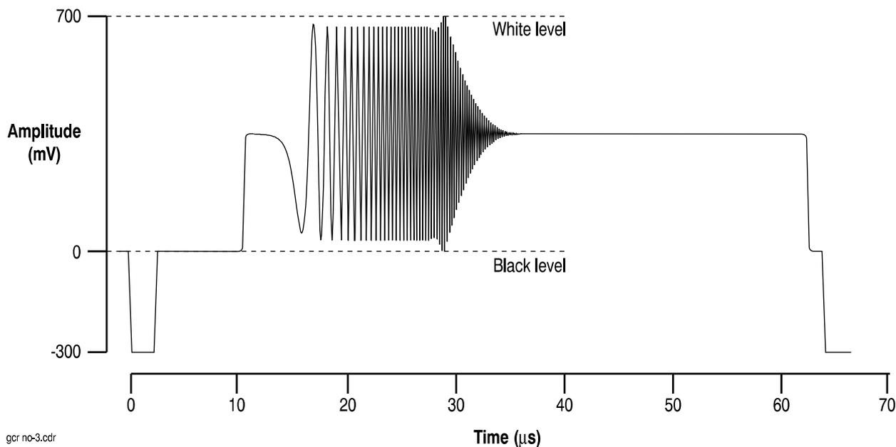
**Figure 3: Line B (negative going) GCR signal**
