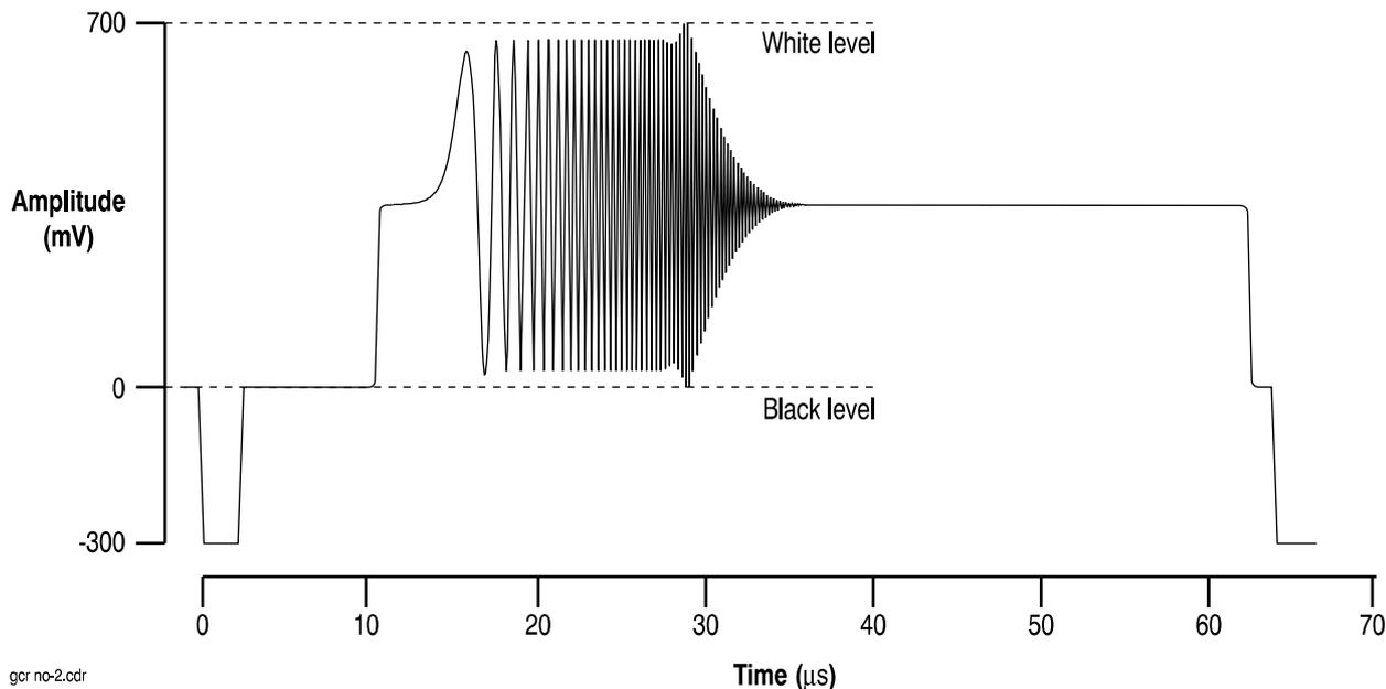
**Figure 2: Line A (positive going) GCR signal**
