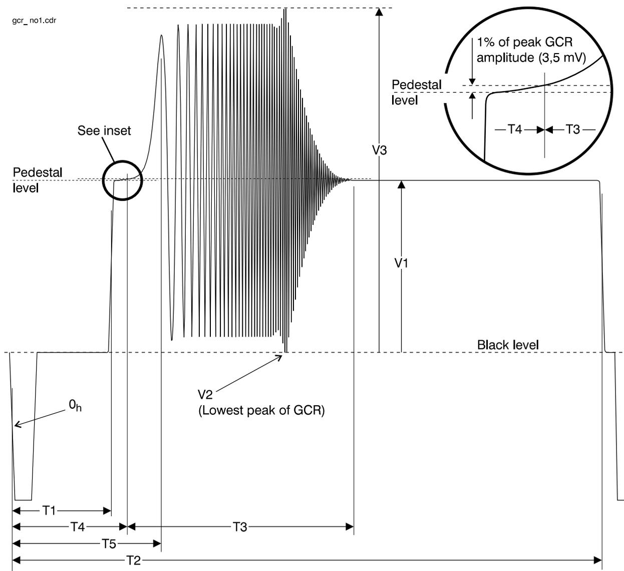
Figure 1: Amplitude and timing of the GCR signal
