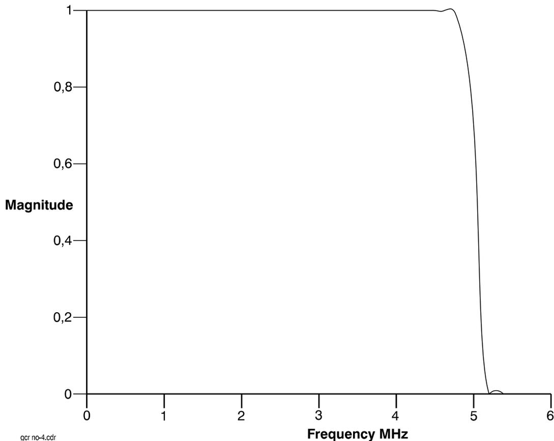
**Figure B.1: Magnitude of the energy spectrum of the GCR signal**
