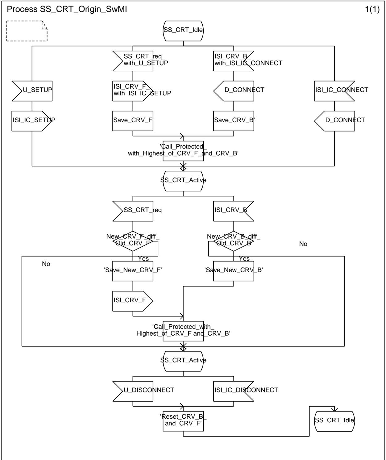
Figure B.2: Originating SwMI SDL (SS-CRT)
