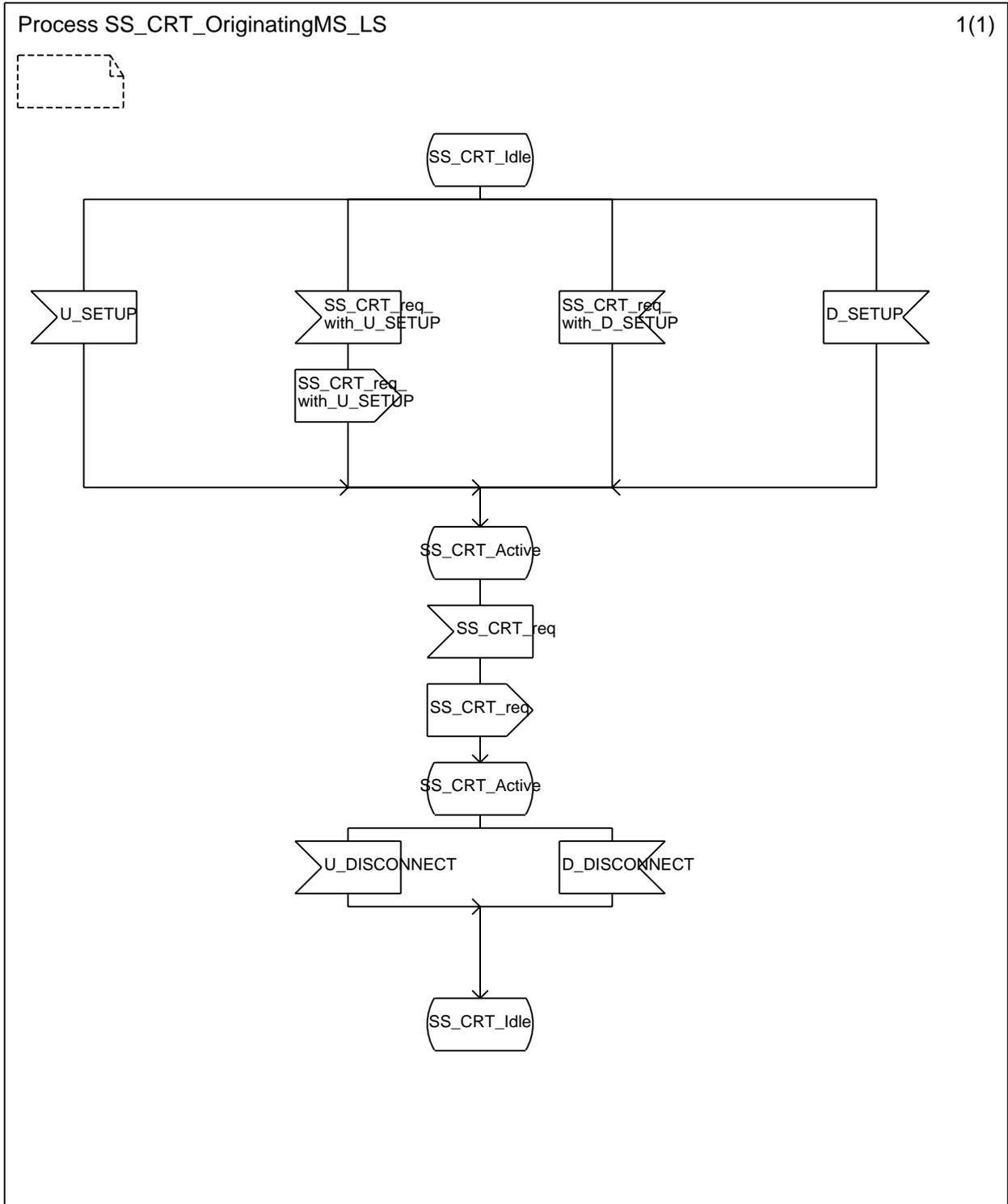
Figure B.1: Originating MS/LS SDL (SS-CRT)
