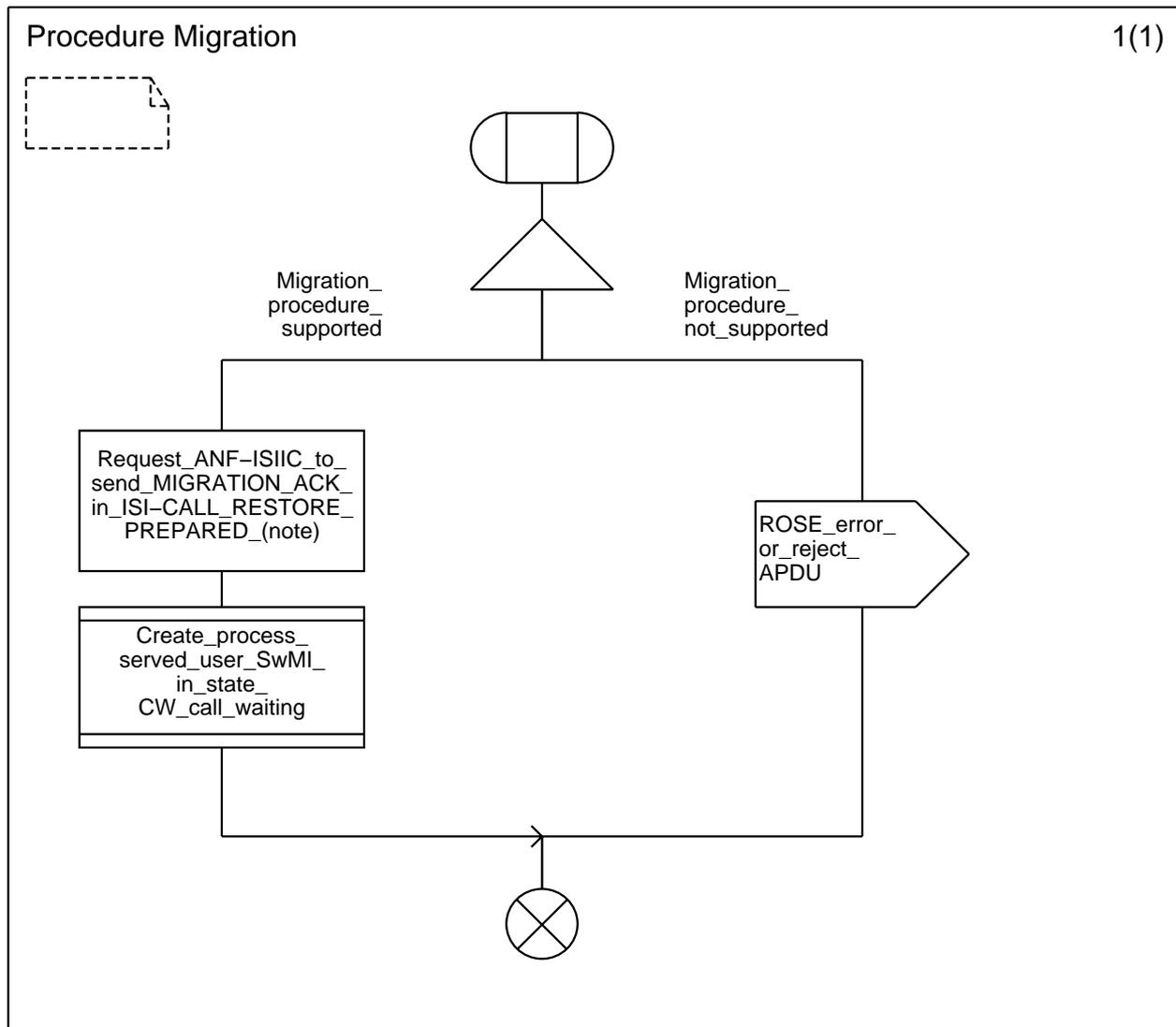
NOTE: ANF-ISIIC may delay the sending of the ANF-ISIIC-CALL RESTORE PREPARED PDU by a few seconds. If the served user decides to accept the waiting call during that time (in sending the U-CONNECT PDU), ANF-ISIIC may skip the sending of the ANF-ISIIC-CALL RESTORE PREPARED PDU in sending directly the ANF-CONNECT PDU. In such a case, the MIGRATION ACK PDU will not be sent.
