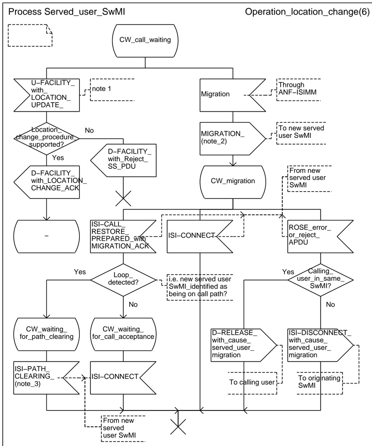
NOTE 1: In the case of migration, i.e. when the new served user SwMI receives the LOCATION CHANGE PDU only after it has taken over the role of served user SwMI (see subclause 5.4.2.1.2.3), the test on the support of the location change procedure in that SDL branch shall always be positive.
