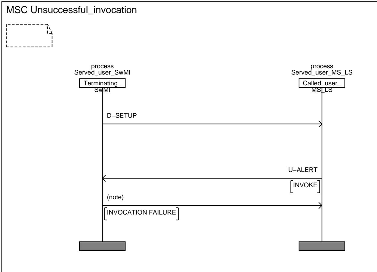
NOTE: The figure corresponds to the case where the basic call procedure continues after SS-CW invocation has failed. The case where the call is cleared because of that invocation failure is also possible (see subclause 5.4.2.2): the INVOCATION FAILURE PDU shall then be sent in the D-RELEASE PDU.
