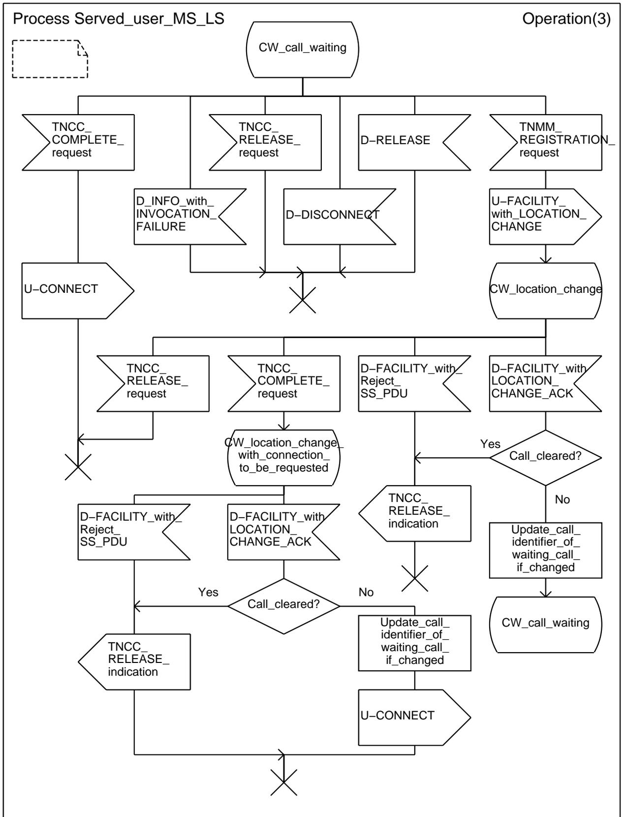
Figure B.1b (sheet 2 of 3): Served user MS/LS SDL - Operation
