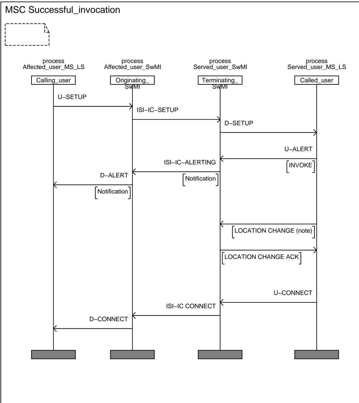
NOTE: The LOCATION CHANGE PDU shall be sent by the served user MS in the cases of roaming or migration and only in such cases. That MS expects then to receive the LOCATION CHANGE ACK PDU. The figure illustrates only the case of roaming.
