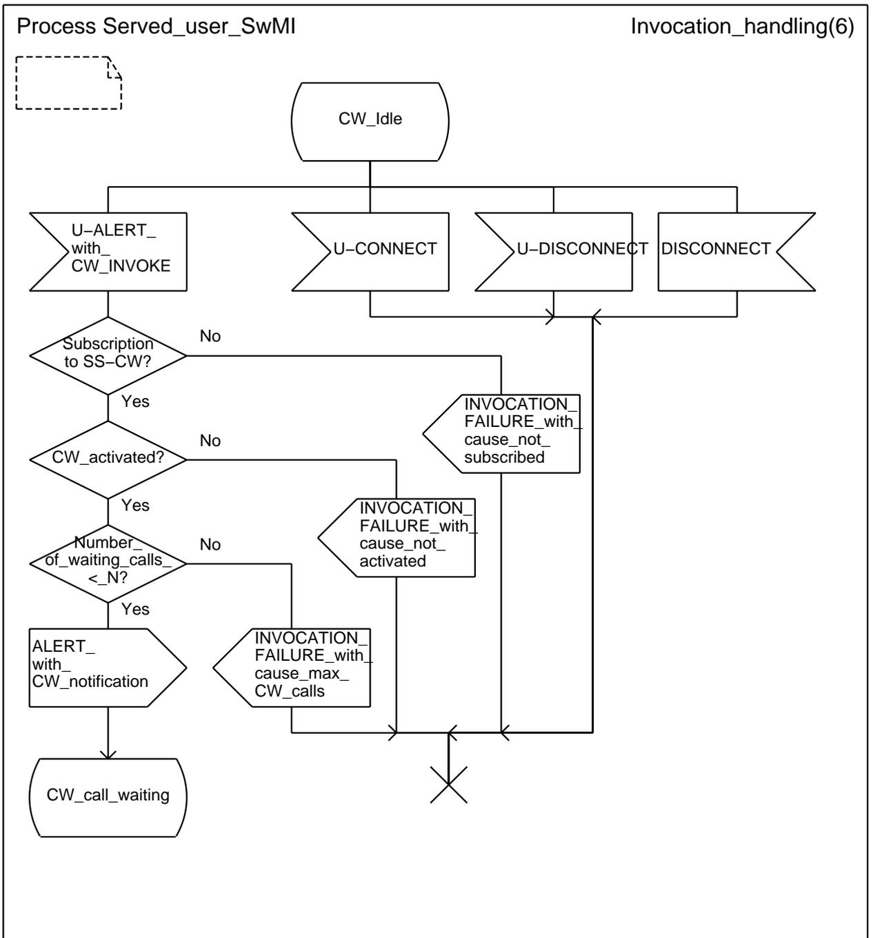
Figure B.2b (sheet 2 of 6): Served user SwMI SDL - Beginning of operation
