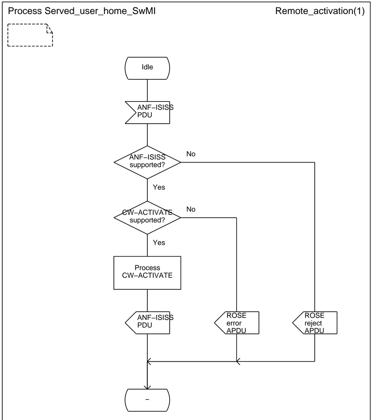
NOTE: Every ANF-ISISS PDU or ROSE APDU is conveyed by a PSS1 FACILITY message. The latter has not been shown in the corresponding signal symbols by lack of space.
