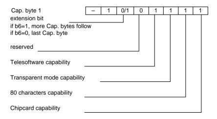
The Telesoftware capability bit and the Transparent mode capability bit shall be used to identify the use of these data types associated with the profiles. Subclause 6.2 gives codes that are used to identify SRM conformance to ETS 300 074 [4] (Transparent data) and ETS 300 075 [5] (Processable data).
