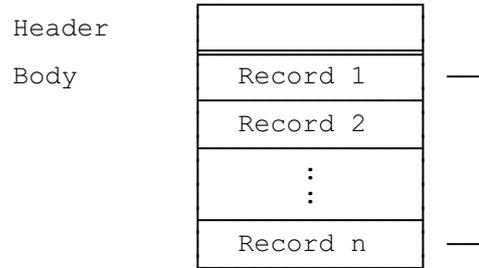
**Figure 6: Structure of a cyclic file**
