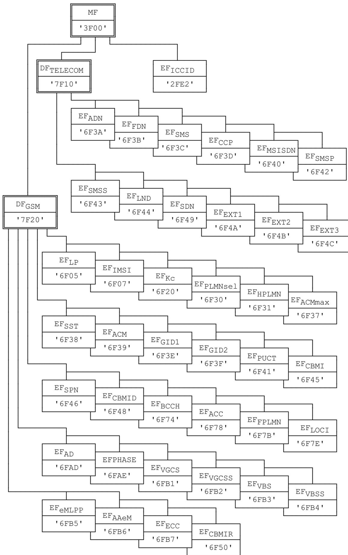
Figure 8: File identifiers and directory structures of GSM
