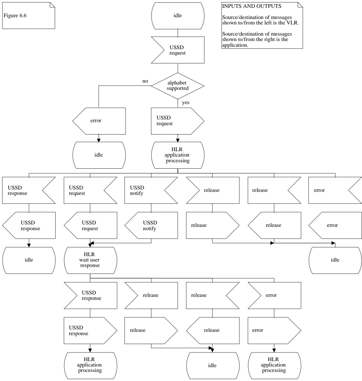
Figure 6.6: Mobile initiated USSD at HLR
